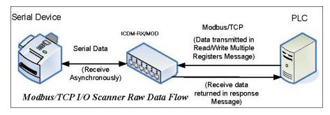
data at set time intervals and typically utilizes the Read/Write multiple Registers message.
