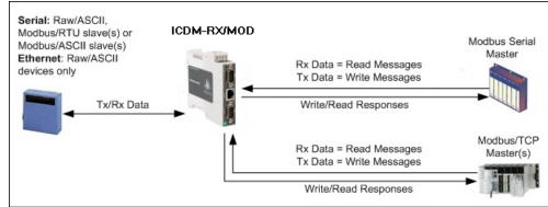
For raw/ASCII mode, the Receive Transfer mode and Transmit Transfer mode are both set to Slave (In Modbus/RTU-to-Slaves and Modbus/ASCII-to-Slaves mode, the ICDM-RX/MOD port only operates in To-Slave mode.
