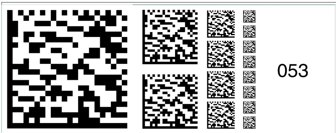
Figure 6.67 The code card "Fieldbus address 053" assigns the fieldbus address 053 to the device.
