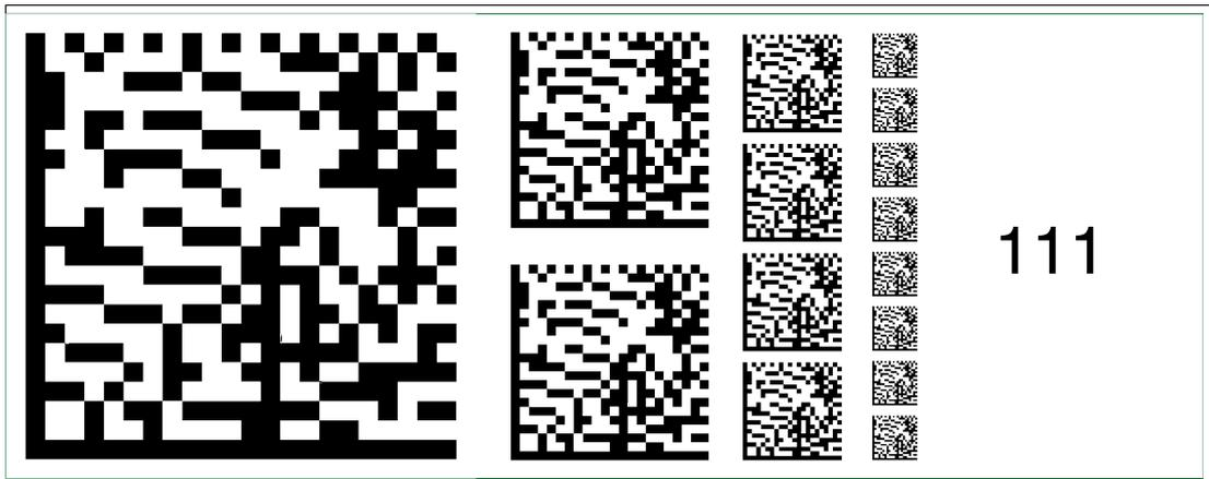
Figure 6.125 The code card "Fieldbus address 111" assigns the fieldbus address 111 to the device.
