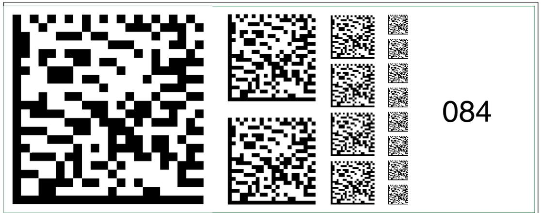
Figure 6.98 The code card "Fieldbus address 084" assigns the fieldbus address 084 to the device.
