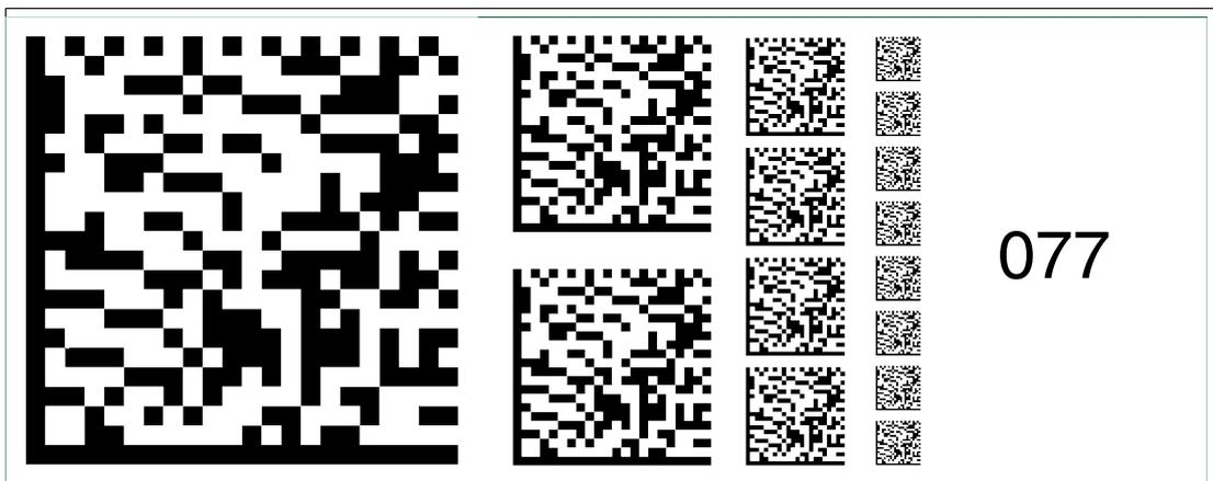
Figure 6.91 The code card "Fieldbus address 077" assigns the fieldbus address 077 to the device.
