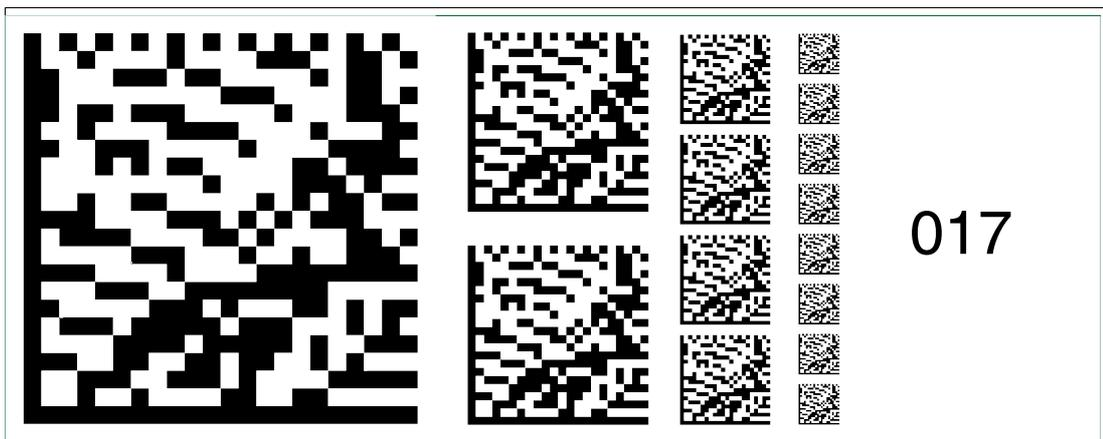
Figure 6.31 The code card "Fieldbus address 017" assigns the fieldbus address 017 to the device.
