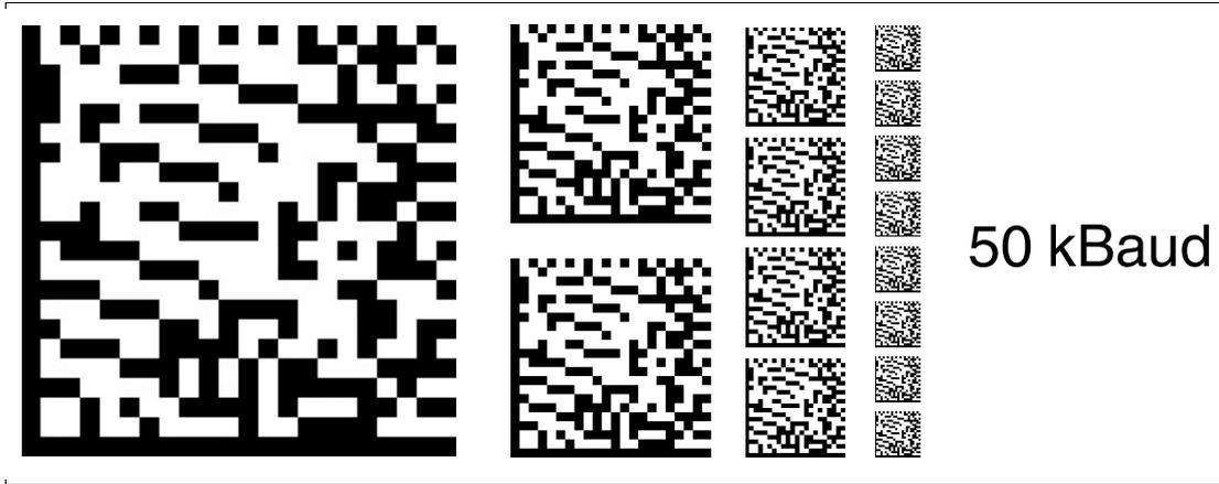
Figure 6.7 The code card assigns the 50 kBaud baud rate to the read head
