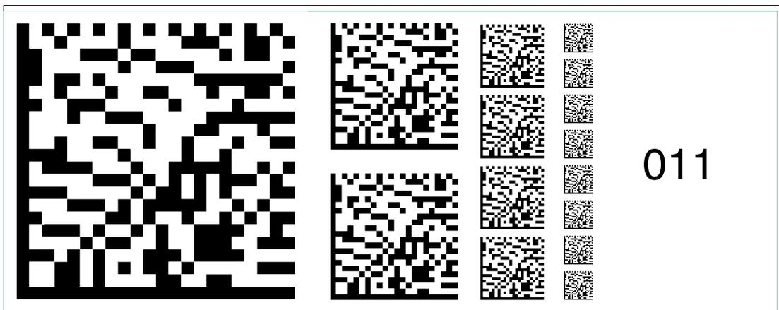
Figure 6.25 The code card "Fieldbus address 011" assigns the fieldbus address 011 to the device.
