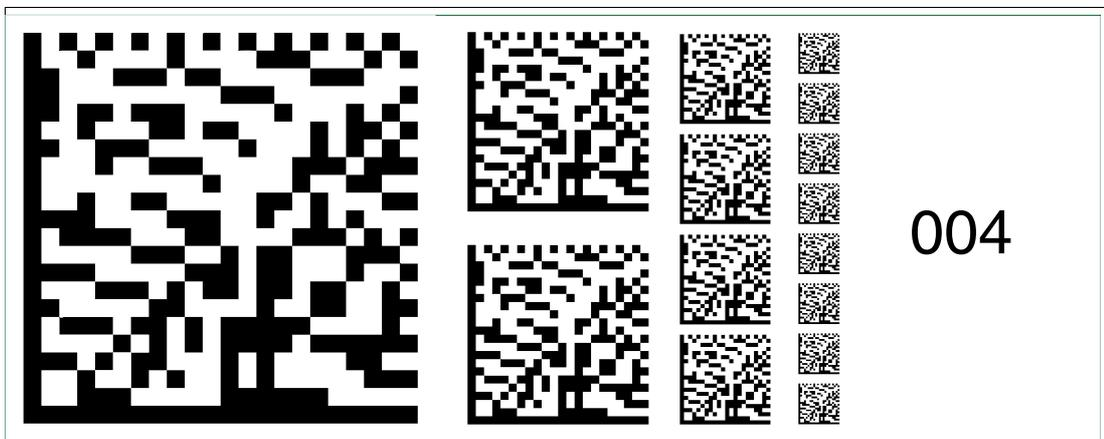
Figure 6.18 The code card "Fieldbus address 004" assigns the fieldbus address 004 to the device.
