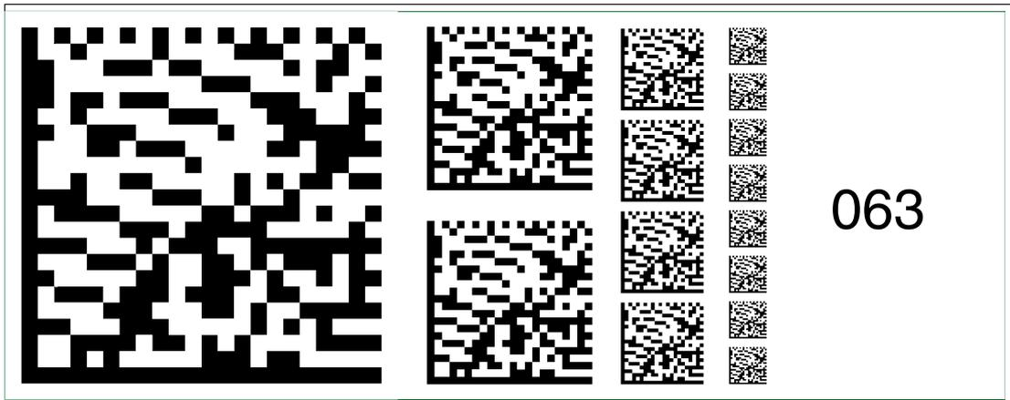
Figure 6.77 The code card "Fieldbus address 063" assigns the fieldbus address 063 to the device.
