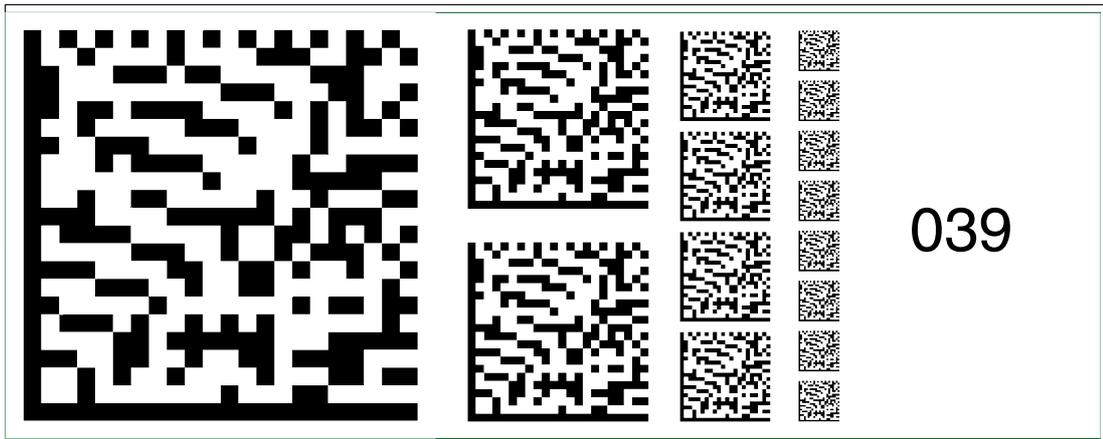
Figure 6.53 The code card "Fieldbus address 039" assigns the fieldbus address 039 to the device.
