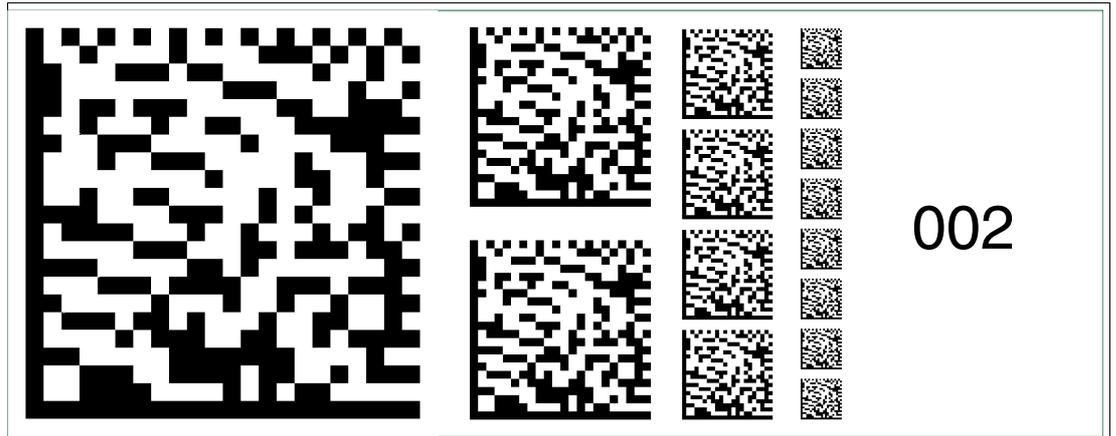
Figure 6.16 The code card "Fieldbus address 002" assigns the fieldbus address 002 to the device.
