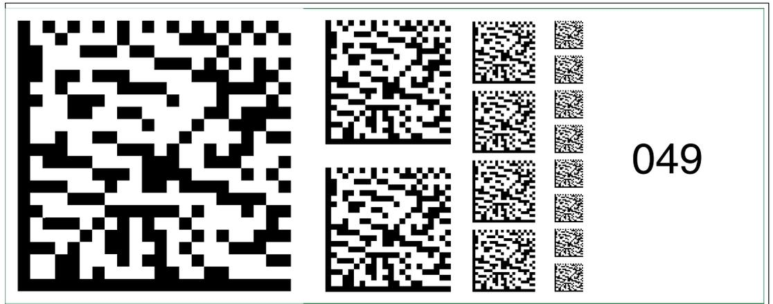
Figure 6.63 The code card "Fieldbus address 049" assigns the fieldbus address 049 to the device.
