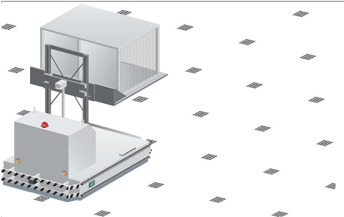
Figure 2.2 Auto-Guided Transport System with Data Matrix tags
