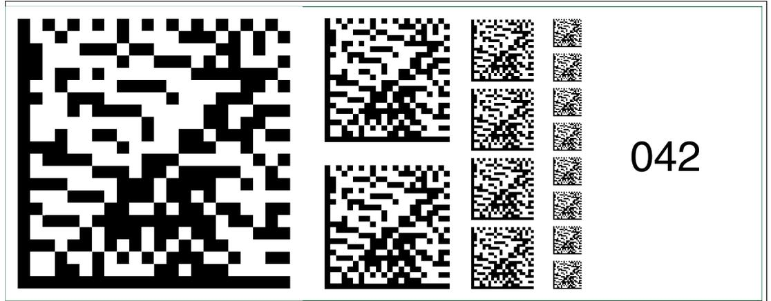
Figure 6.56 The code card "Fieldbus address 042" assigns the fieldbus address 042 to the device.
