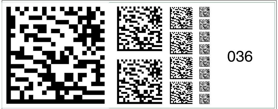
Figure 6.50 The code card "Fieldbus address 036" assigns the fieldbus address 036 to the device.
