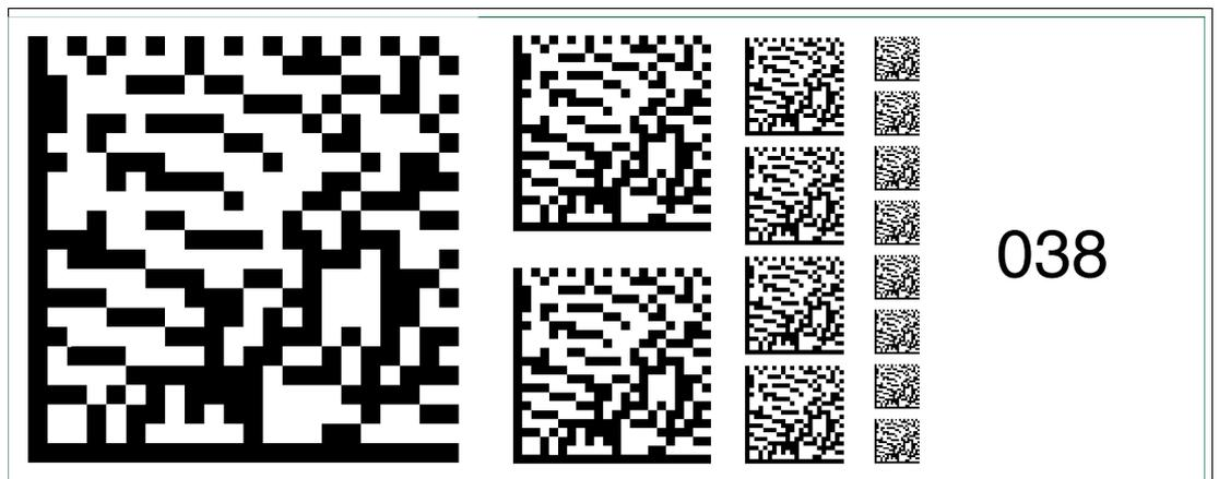
Figure 6.52 The code card "Fieldbus address 038" assigns the fieldbus address 038 to the device.
