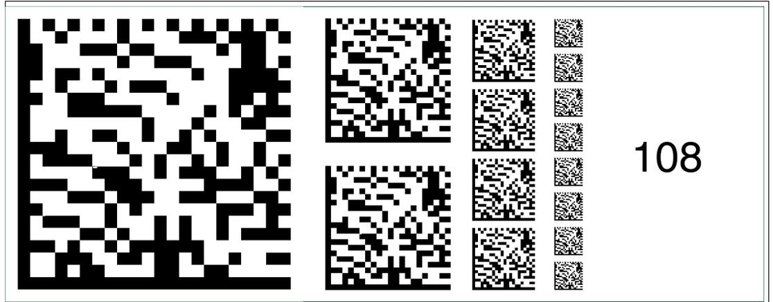
Figure 6.122 The code card "Fieldbus address 108" assigns the fieldbus address 108 to the device.
