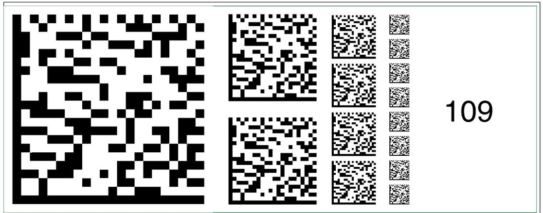
Figure 6.123 The code card "Fieldbus address 109" assigns the fieldbus address 109 to the device.
