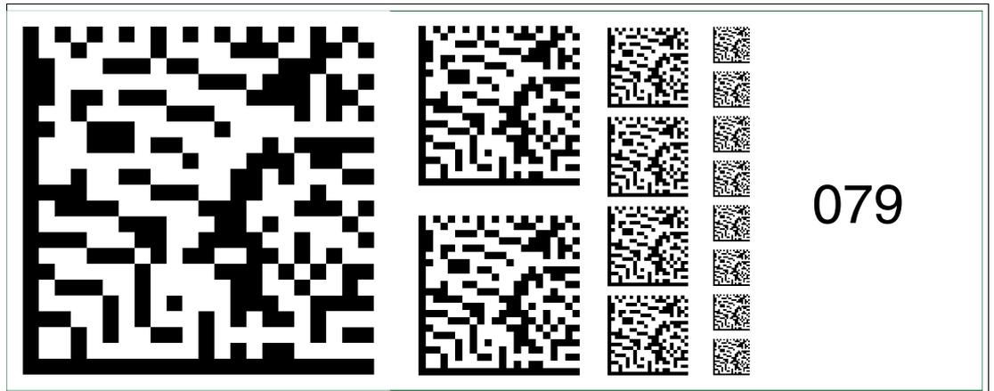
Figure 6.93 The code card "Fieldbus address 079" assigns the fieldbus address 079 to the device.
