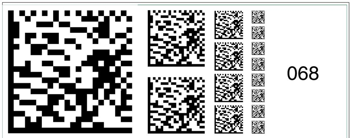
Figure 6.82 The code card "Fieldbus address 068" assigns the fieldbus address 068 to the device.
