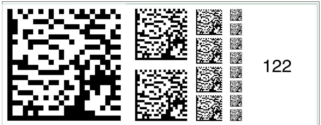
Figure 6.136 The code card "Fieldbus address 122" assigns the fieldbus address 122 to the device.
