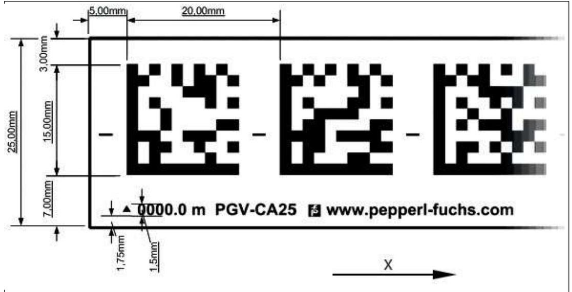
Figure 3.2 Dimensions of the Data Matrix code tape
