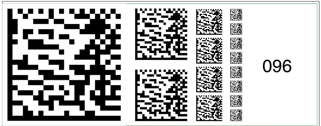
Figure 6.110 The code card "Fieldbus address 096" assigns the fieldbus address 096 to the device.
