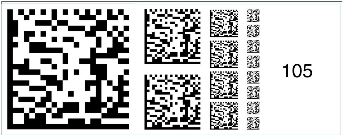
Figure 6.119 The code card "Fieldbus address 105" assigns the fieldbus address 105 to the device.
