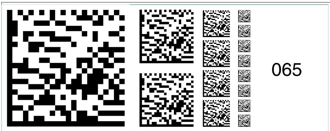
Figure 6.79 The code card "Fieldbus address 065" assigns the fieldbus address 065 to the device.
