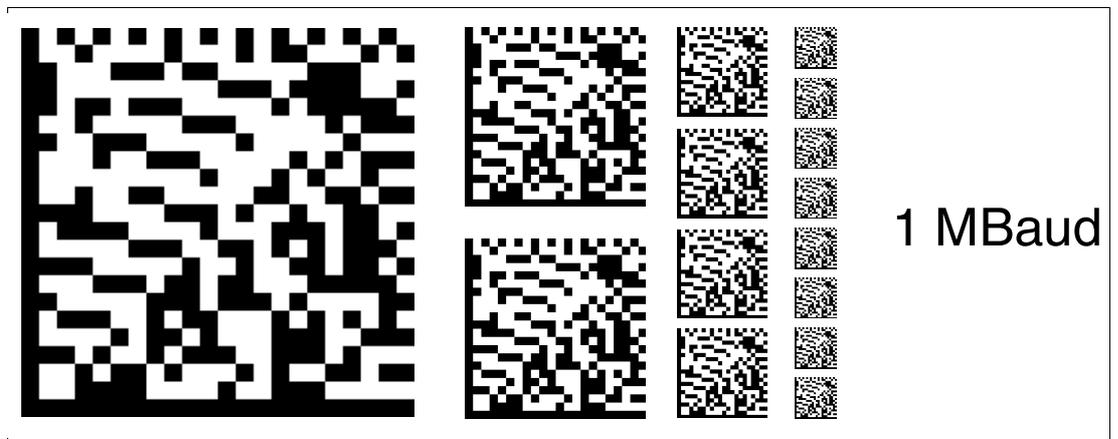
Figure 6.11 The code card assigns the 1 MBaud baud rate to the read head
