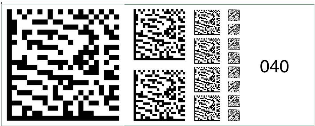
Figure 6.54 The code card "Fieldbus address 040" assigns the fieldbus address 040 to the device.
