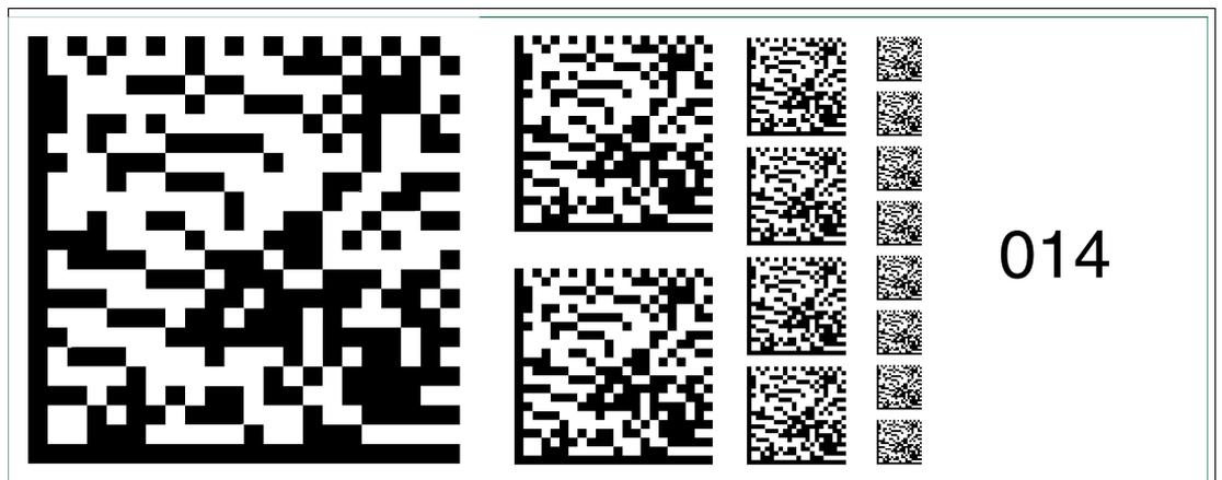
Figure 6.28 The code card "Fieldbus address 014" assigns the fieldbus address 014 to the device.
