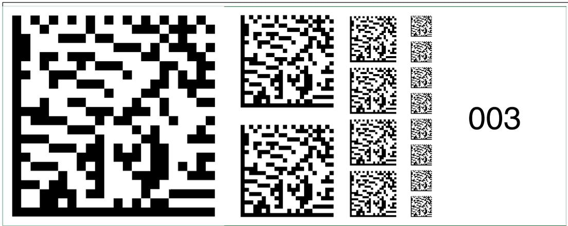
Figure 6.17 The code card "Fieldbus address 003" assigns the fieldbus address 003 to the device.
