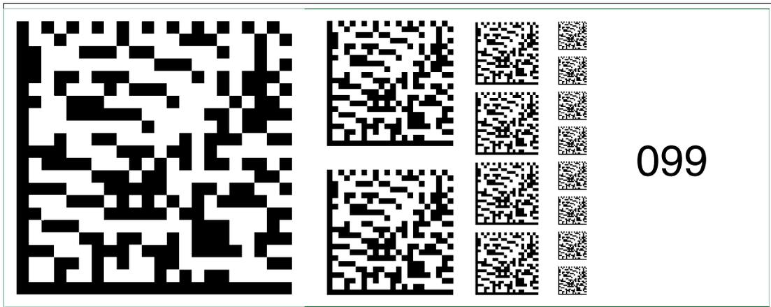
Figure 6.113 The code card "Fieldbus address 099" assigns the fieldbus address 099 to the device.
