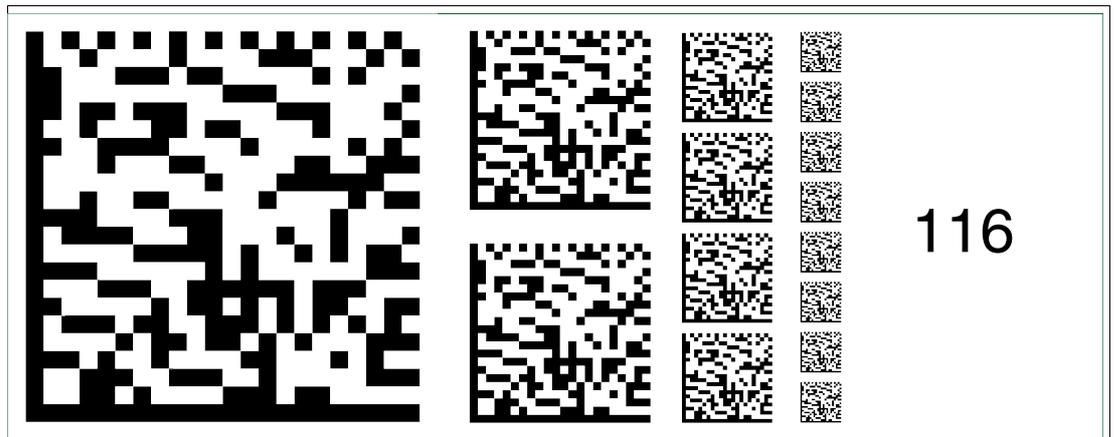
Figure 6.130 The code card "Fieldbus address 116" assigns the fieldbus address 116 to the device.
