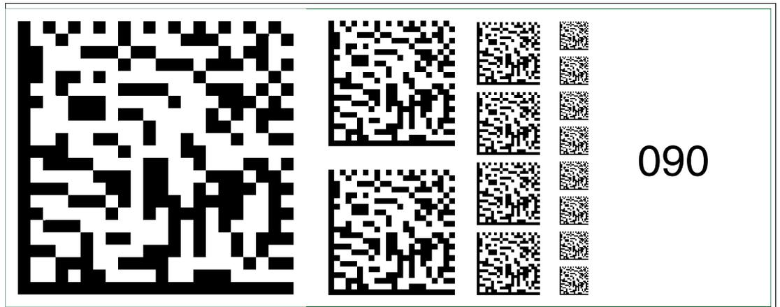
Figure 6.104 The code card "Fieldbus address 090" assigns the fieldbus address 090 to the device.
