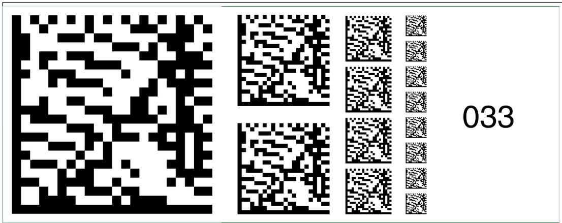
Figure 6.47 The code card "Fieldbus address 033" assigns the fieldbus address 033 to the device.
