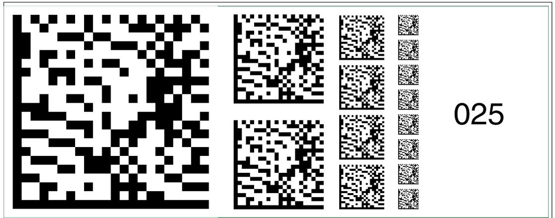
Figure 6.39 The code card "Fieldbus address 025" assigns the fieldbus address 025 to the device.
