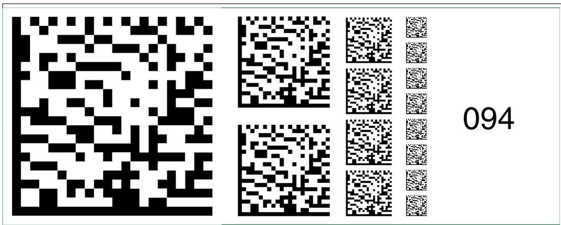
Figure 6.108 The code card "Fieldbus address 094" assigns the fieldbus address 094 to the device.
