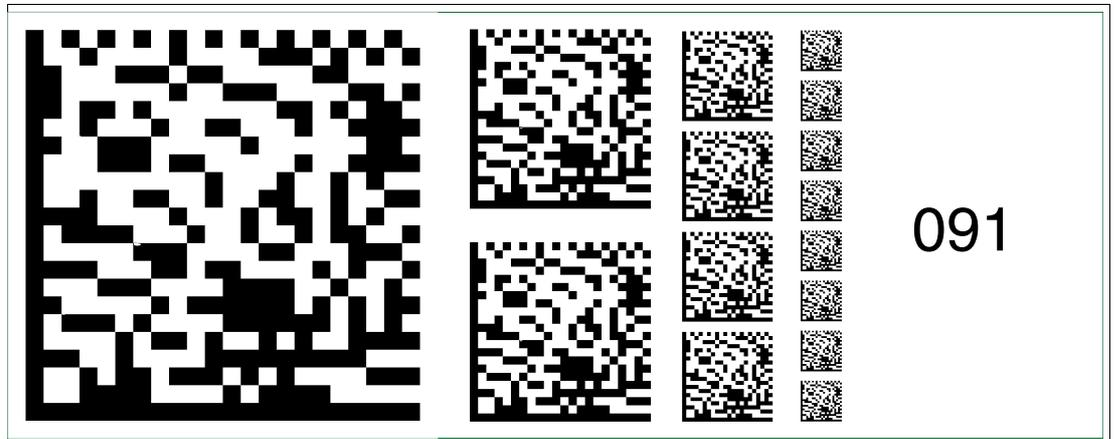
Figure 6.105 The code card "Fieldbus address 091" assigns the fieldbus address 091 to the device.
