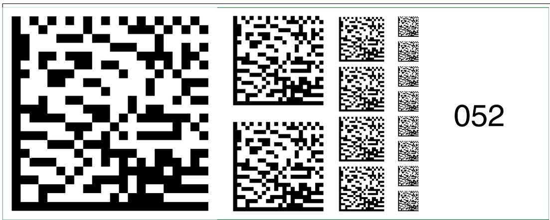
Figure 6.66 The code card "Fieldbus address 052" assigns the fieldbus address 052 to the device.
