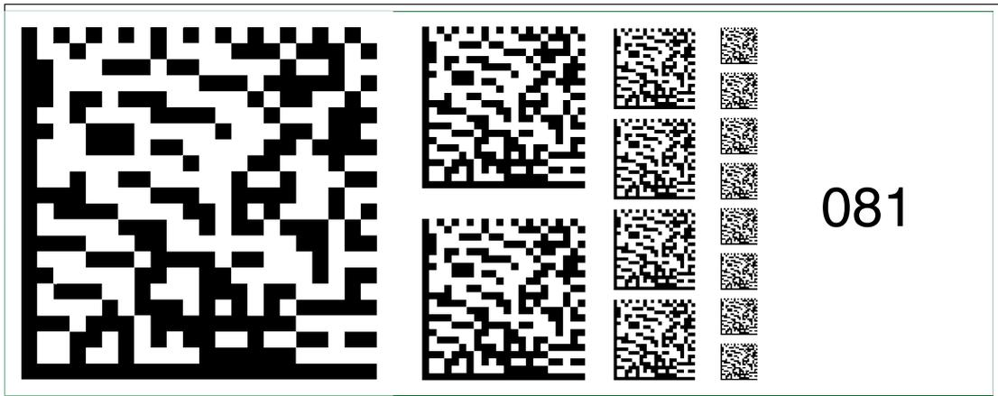
Figure 6.95 The code card "Fieldbus address 081" assigns the fieldbus address 081 to the device.
