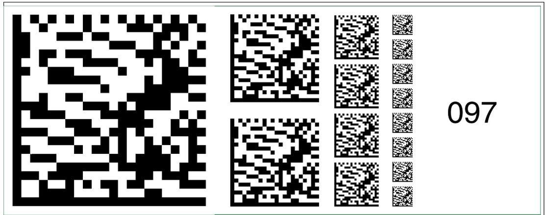
Figure 6.111 The code card "Fieldbus address 097" assigns the fieldbus address 097 to the device.
