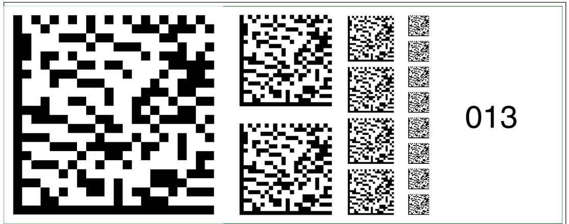
Figure 6.27 The code card "Fieldbus address 013" assigns the fieldbus address 013 to the device.
