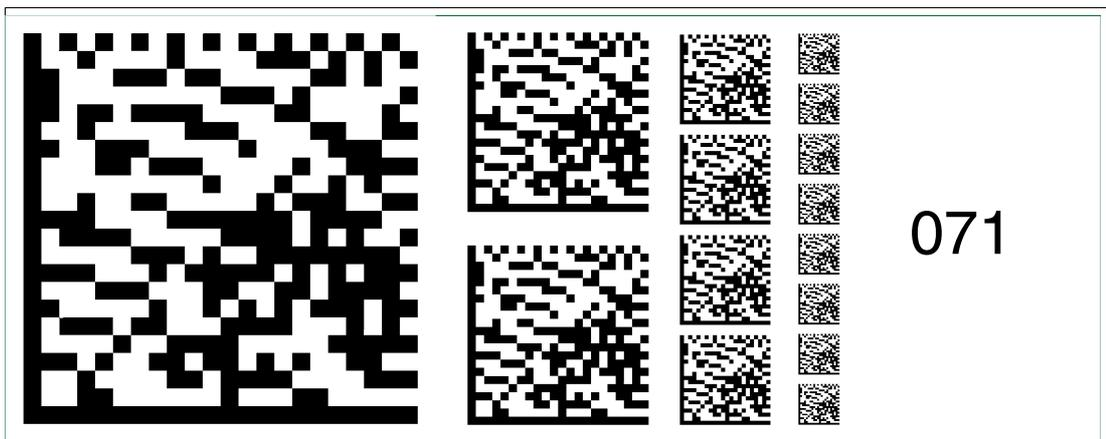
Figure 6.85 The code card "Fieldbus address 071" assigns the fieldbus address 071 to the device.
