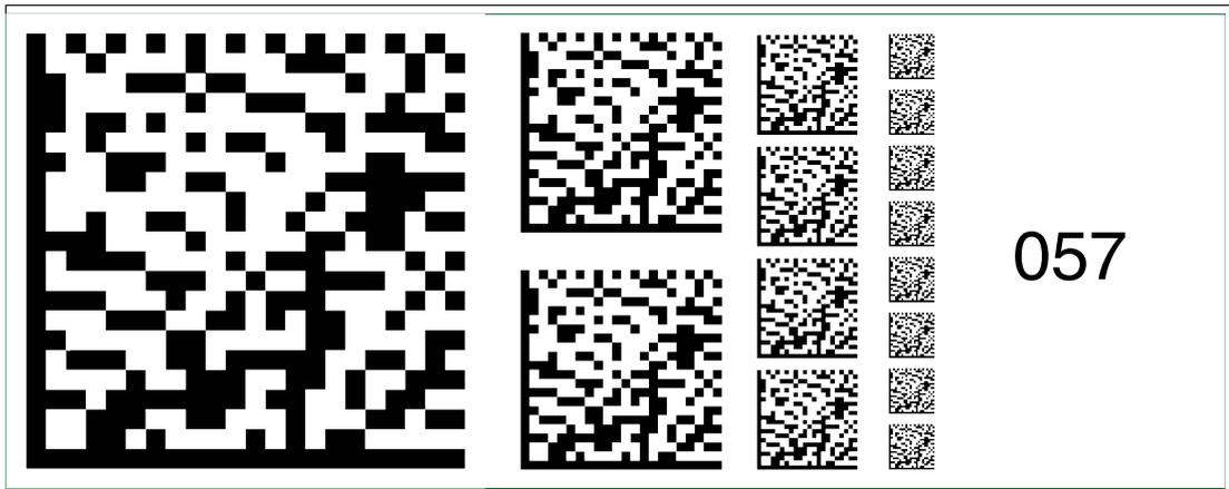
Figure 6.71 The code card "Fieldbus address 057" assigns the fieldbus address 057 to the device.
