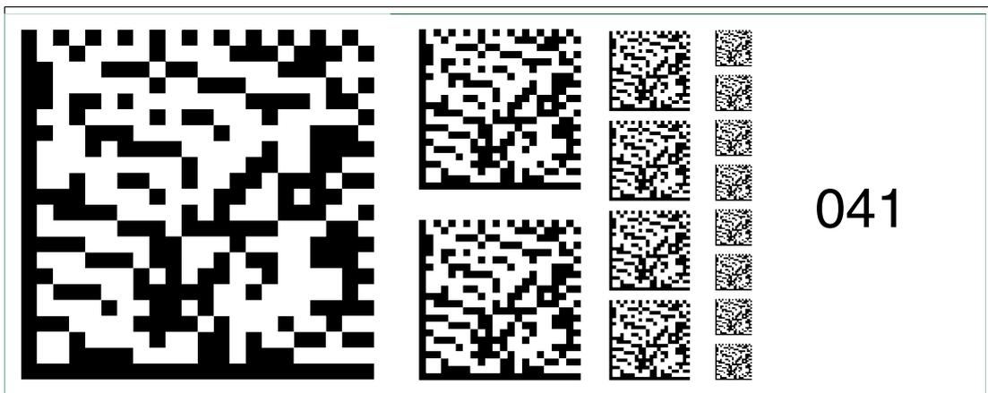
Figure 6.55 The code card "Fieldbus address 041" assigns the fieldbus address 041 to the device.
