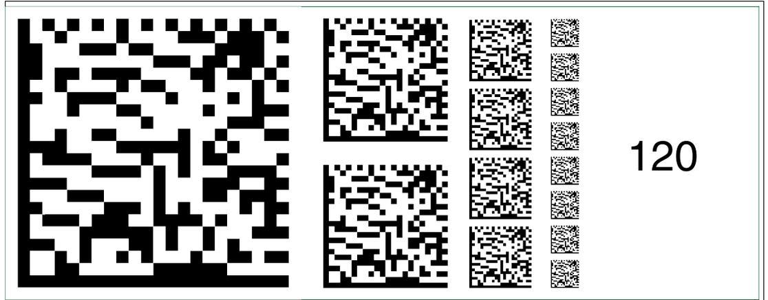
Figure 6.134 The code card "Fieldbus address 120" assigns the fieldbus address 120 to the device.
