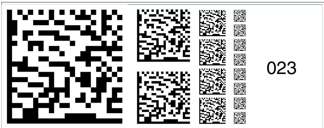
Figure 6.37 The code card "Fieldbus address 023" assigns the fieldbus address 023 to the device.
