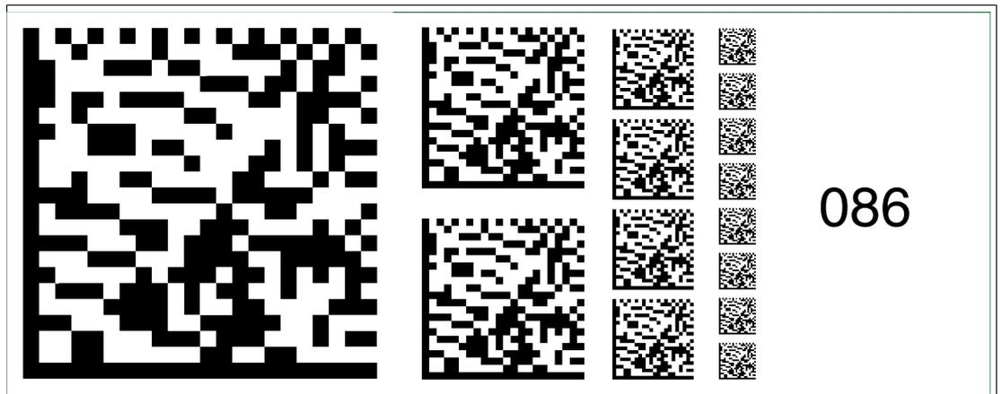
Figure 6.100 The code card "Fieldbus address 086" assigns the fieldbus address 086 to the device.
