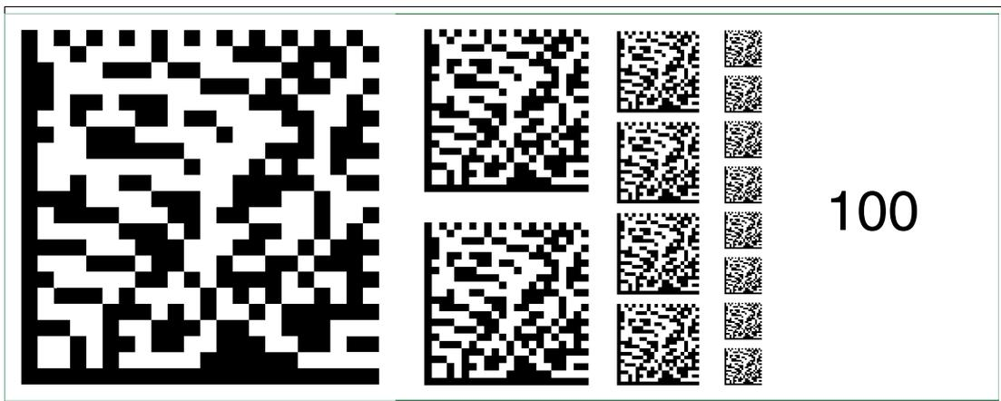
Figure 6.114 The code card "Fieldbus address 100" assigns the fieldbus address 100 to the device.
