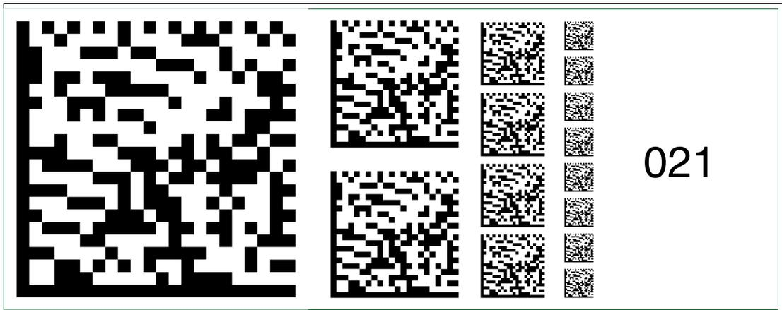
Figure 6.35 The code card "Fieldbus address 021" assigns the fieldbus address 021 to the device.
