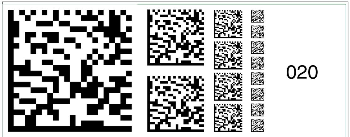
Figure 6.34 The code card "Fieldbus address 020" assigns the fieldbus address 020 to the device.
