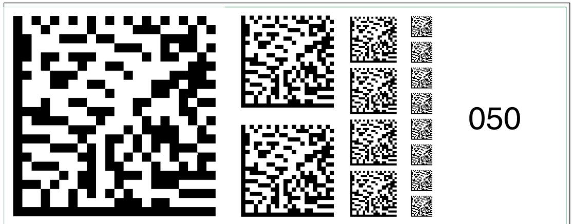
Figure 6.64 The code card "Fieldbus address 050" assigns the fieldbus address 050 to the device.
