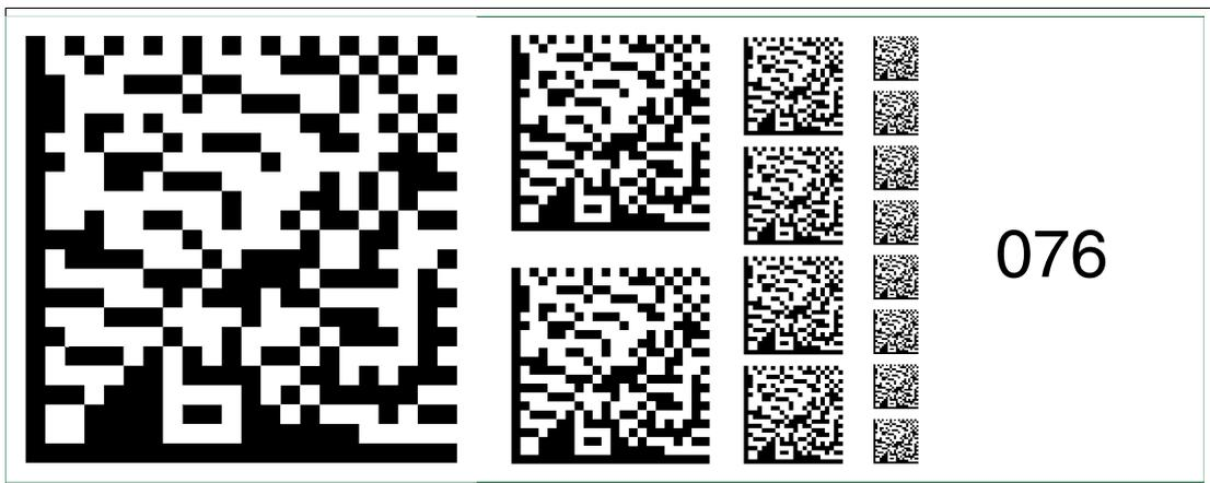
Figure 6.90 The code card "Fieldbus address 076" assigns the fieldbus address 076 to the device.
