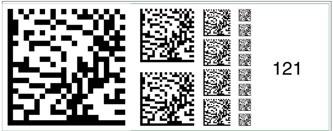
Figure 6.135 The code card "Fieldbus address 121" assigns the fieldbus address 121 to the device.
