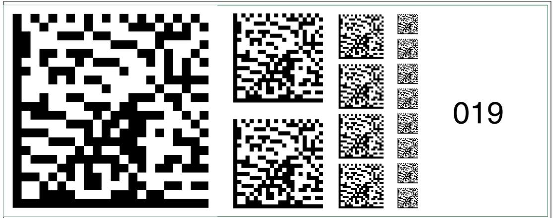
Figure 6.33 The code card "Fieldbus address 019" assigns the fieldbus address 019 to the device.
