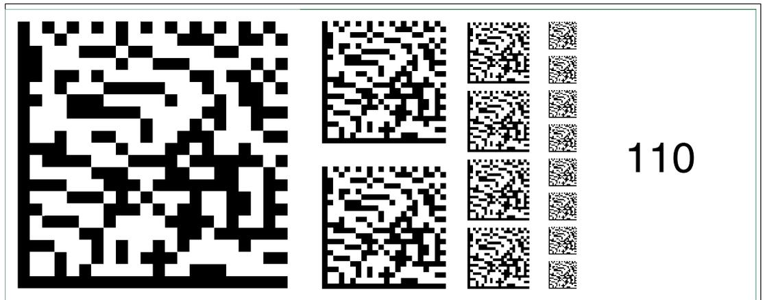
Figure 6.124 The code card "Fieldbus address 110" assigns the fieldbus address 110 to the device.
