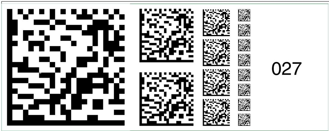
Figure 6.41 The code card "Fieldbus address 027" assigns the fieldbus address 027 to the device.
