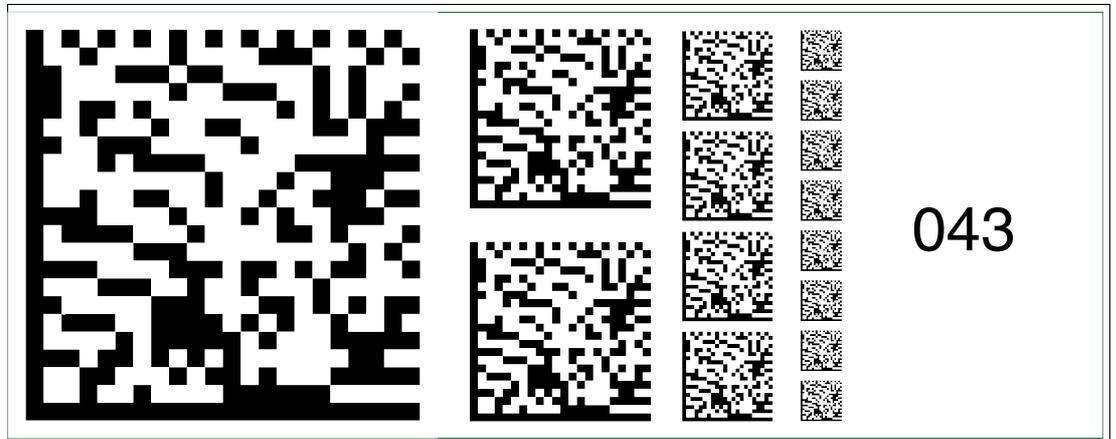
Figure 6.57 The code card "Fieldbus address 043" assigns the fieldbus address 043 to the device.
