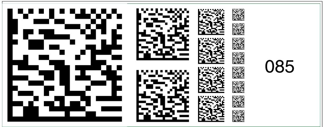
Figure 6.99 The code card "Fieldbus address 085" assigns the fieldbus address 085 to the device.
