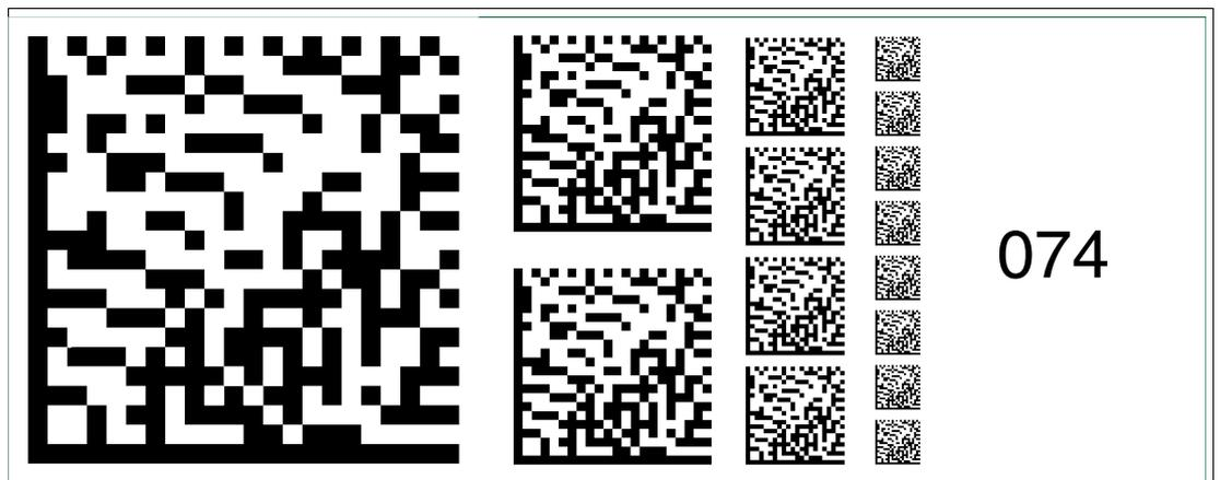
Figure 6.88 The code card "Fieldbus address 074" assigns the fieldbus address 074 to the device.
