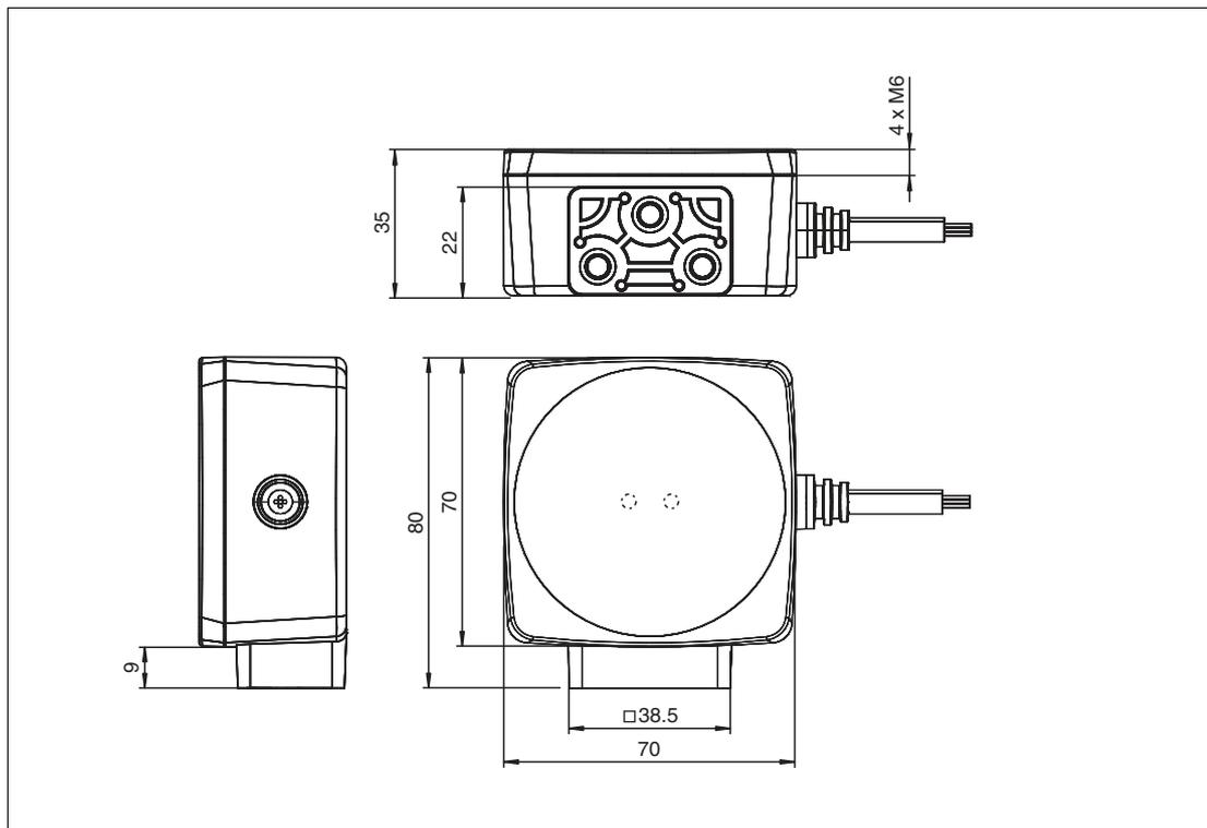
Figure 3.1 Housing dimensions
