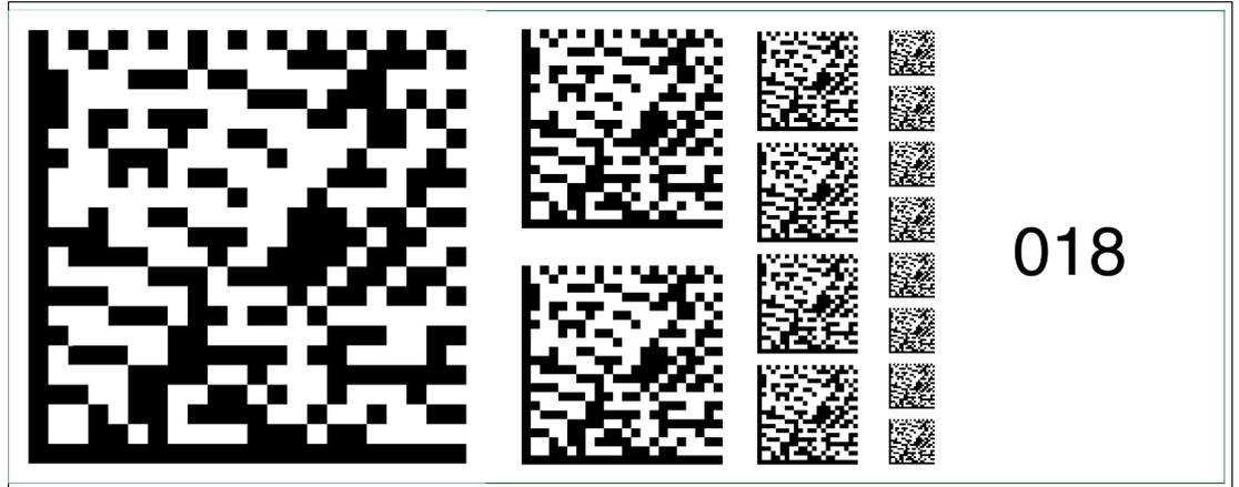
Figure 6.32 The code card "Fieldbus address 018" assigns the fieldbus address 018 to the device.
