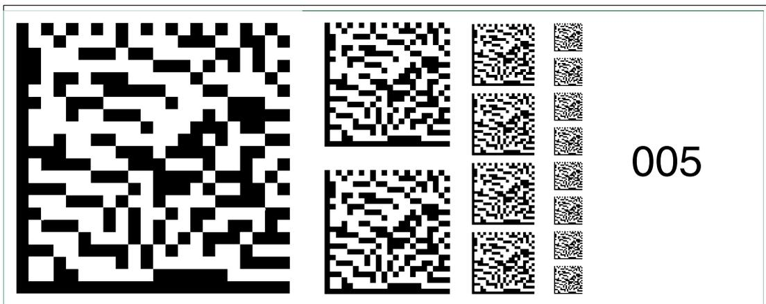
Figure 6.19 The code card "Fieldbus address 005" assigns the fieldbus address 005 to the device.
