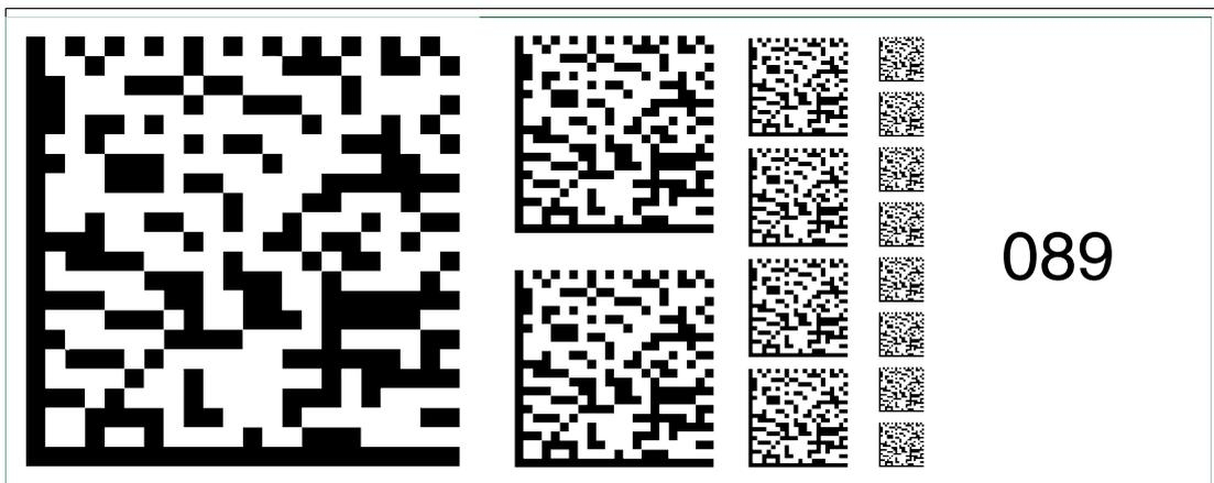
Figure 6.103 The code card "Fieldbus address 089" assigns the fieldbus address 089 to the device.
