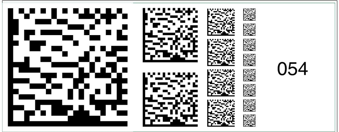
Figure 6.68 The code card "Fieldbus address 054" assigns the fieldbus address 054 to the device.
