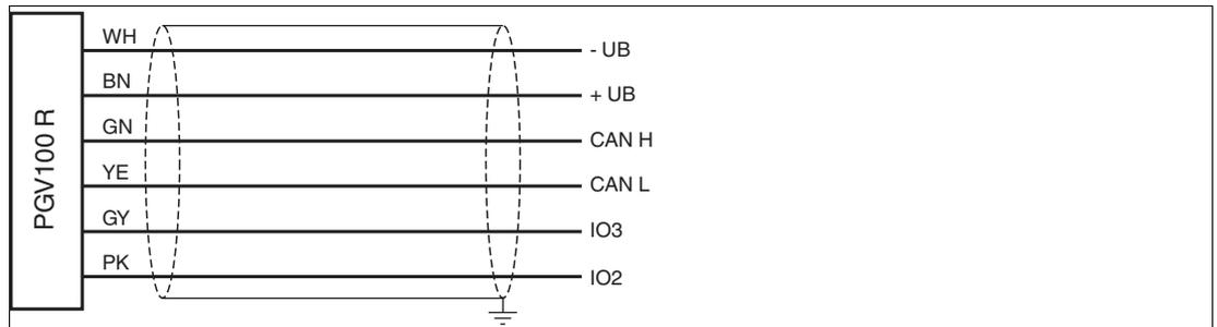
Figure 3.15 Electrical Connection
