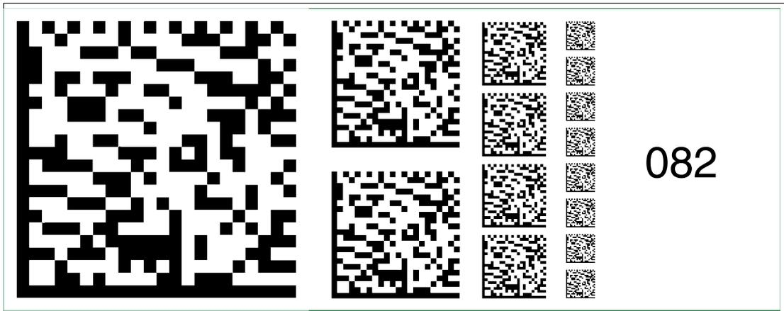
Figure 6.96 The code card "Fieldbus address 082" assigns the fieldbus address 082 to the device.
