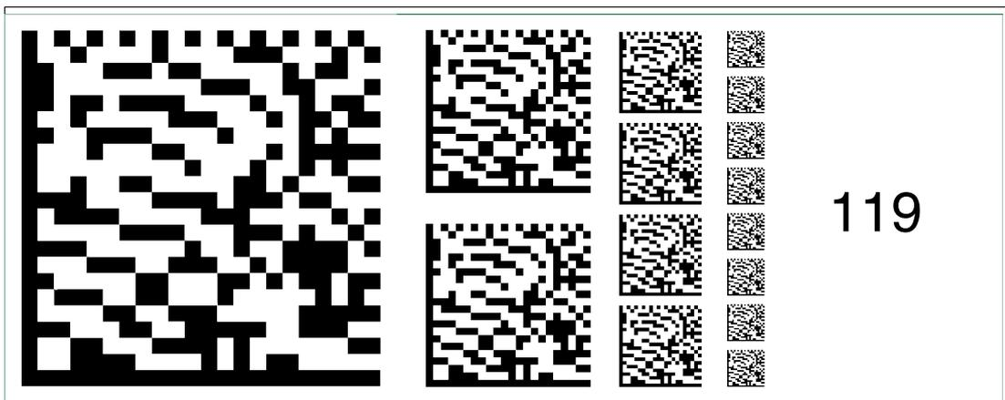
Figure 6.133 The code card "Fieldbus address 119" assigns the fieldbus address 119 to the device.
