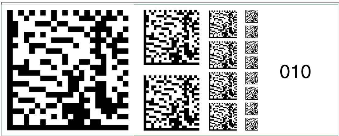
Figure 6.24 The code card "Fieldbus address 010" assigns the fieldbus address 010 to the device.
