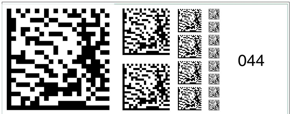
Figure 6.58 The code card "Fieldbus address 044" assigns the fieldbus address 044 to the device.
