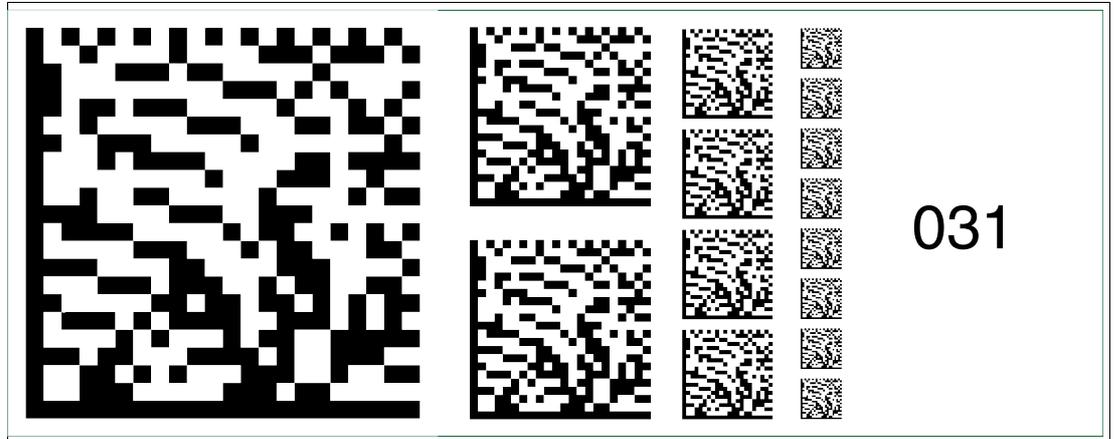
Figure 6.45 The code card "Fieldbus address 031" assigns the fieldbus address 031 to the device.
