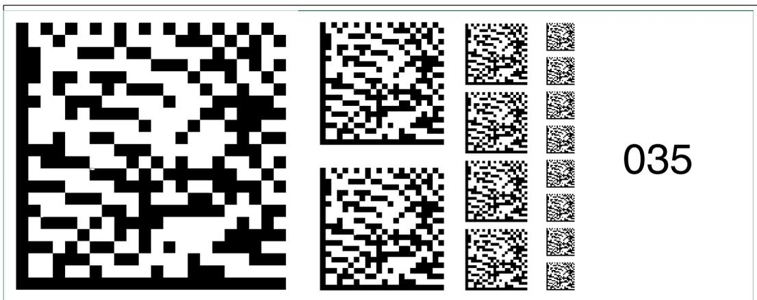
Figure 6.49 The code card "Fieldbus address 035" assigns the fieldbus address 035 to the device.
