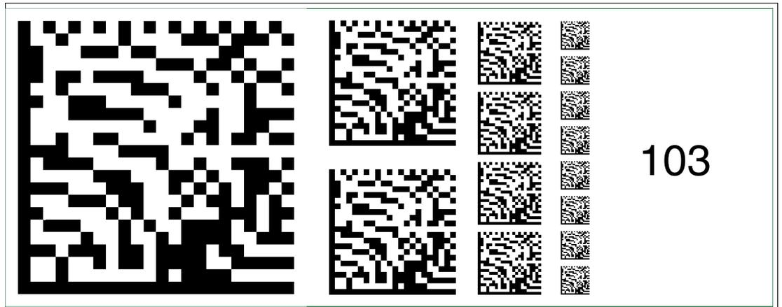
Figure 6.117 The code card "Fieldbus address 103" assigns the fieldbus address 103 to the device.
