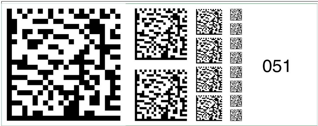
Figure 6.65 The code card "Fieldbus address 051" assigns the fieldbus address 051 to the device.
