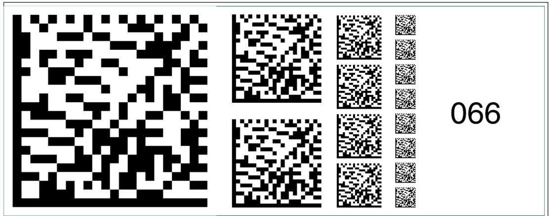
Figure 6.80 The code card "Fieldbus address 066" assigns the fieldbus address 066 to the device.
