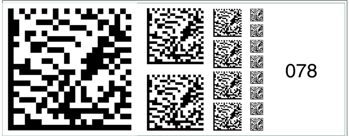
Figure 6.92 The code card "Fieldbus address 078" assigns the fieldbus address 078 to the device.
