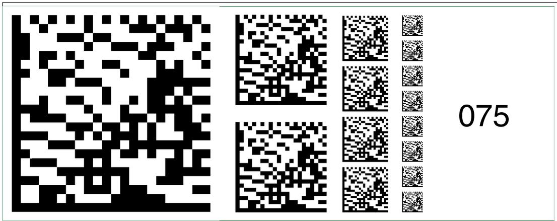
Figure 6.89 The code card "Fieldbus address 075" assigns the fieldbus address 075 to the device.
