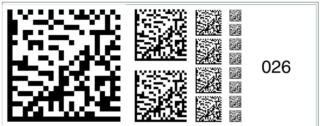
Figure 6.40 The code card "Fieldbus address 026" assigns the fieldbus address 026 to the device.
