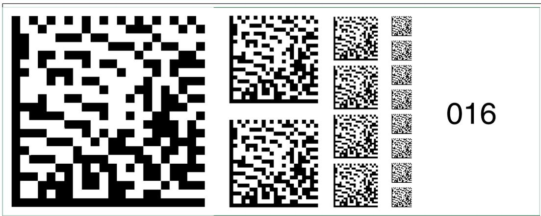
Figure 6.30 The code card "Fieldbus address 016" assigns the fieldbus address 016 to the device.
