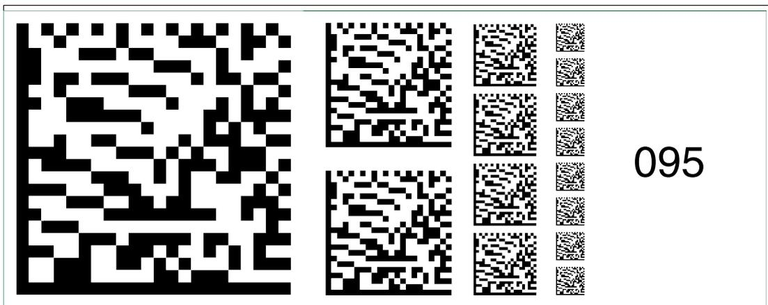
Figure 6.109 The code card "Fieldbus address 095" assigns the fieldbus address 095 to the device.
