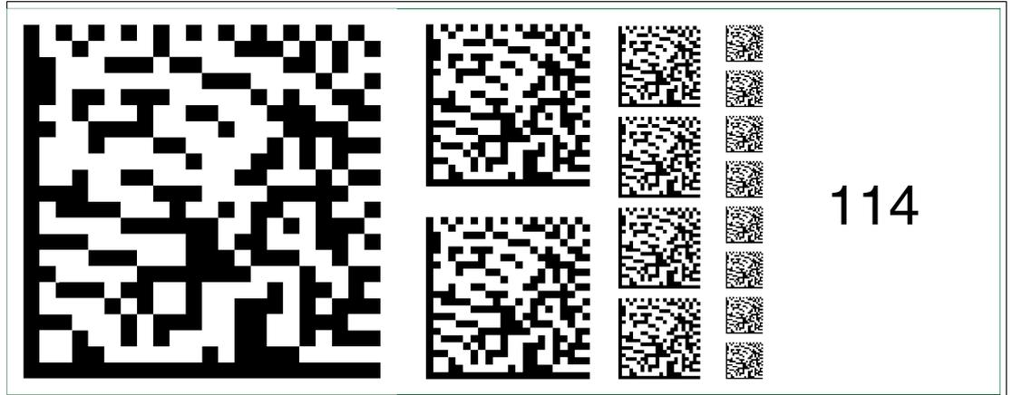
Figure 6.128 The code card "Fieldbus address 114" assigns the fieldbus address 114 to the device.
