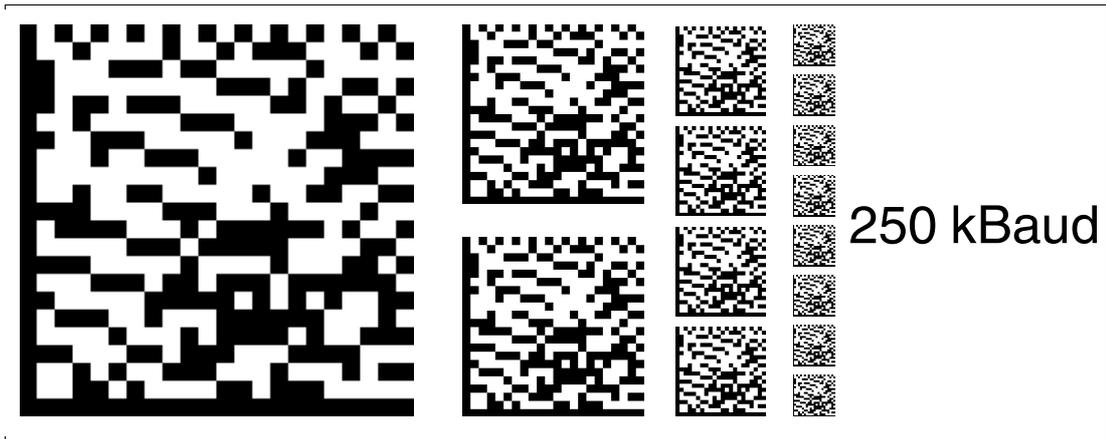
Figure 6.9 The code card assigns the 250 kBaud baud rate to the read head
