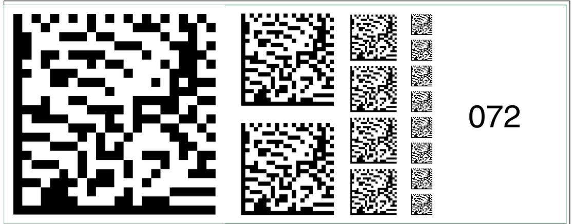
Figure 6.86 The code card "Fieldbus address 072" assigns the fieldbus address 072 to the device.
