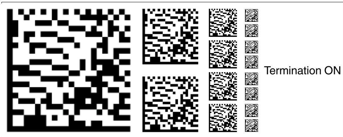
Figure 6.13 The Termination ON code card activates the termination resistor on the bus.
