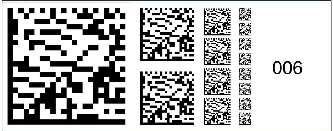
Figure 6.20 The code card "Fieldbus address 006" assigns the fieldbus address 006 to the device.
