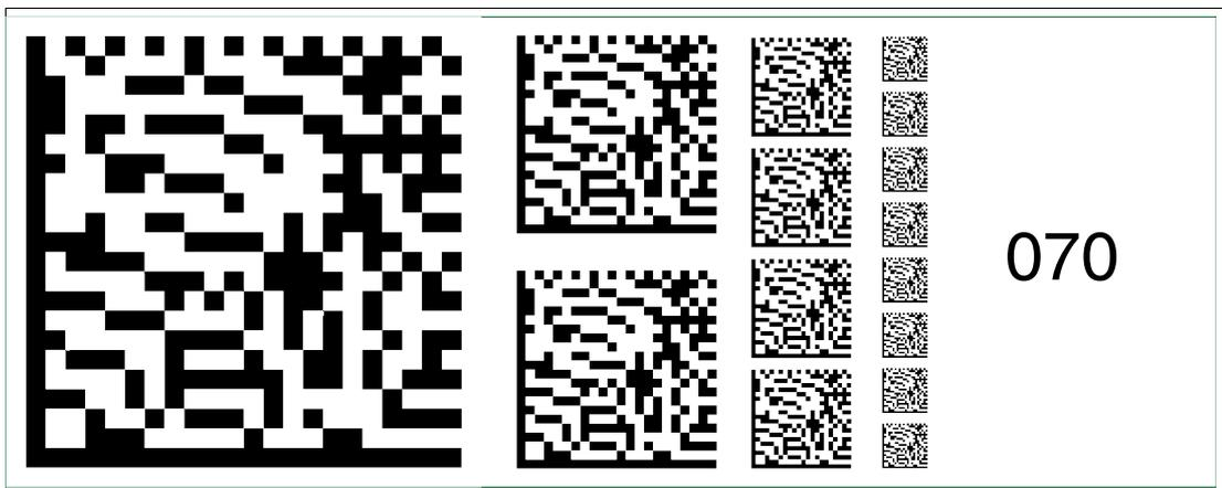
Figure 6.84 The code card "Fieldbus address 070" assigns the fieldbus address 070 to the device.
