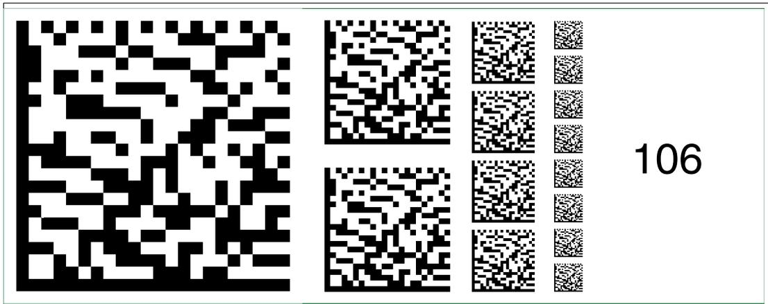
Figure 6.120 The code card "Fieldbus address 106" assigns the fieldbus address 106 to the device.
