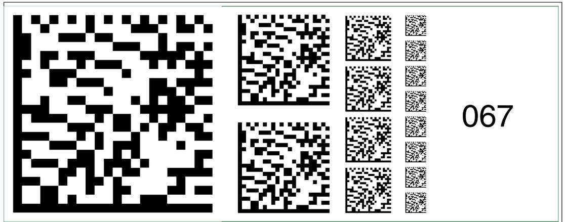
Figure 6.81 The code card "Fieldbus address 067" assigns the fieldbus address 067 to the device.
