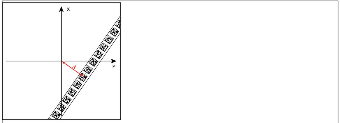
Figure 3.5 Distance A for Data Matrix code tape
