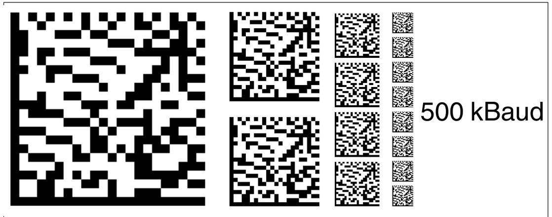
Figure 6.10 The code card assigns the 500 kBaud baud rate to the read head
