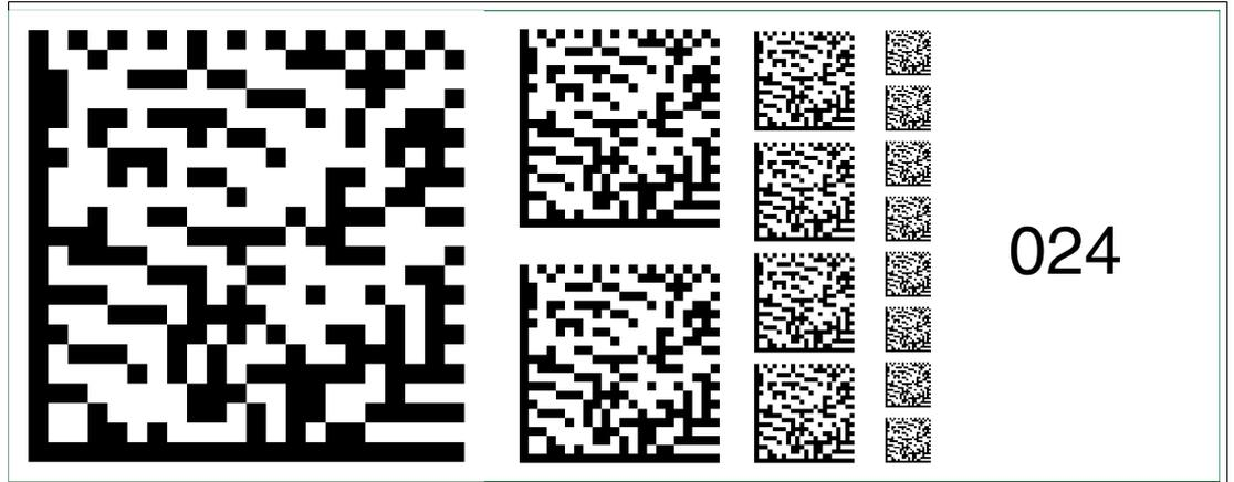
Figure 6.38 The code card "Fieldbus address 024" assigns the fieldbus address 024 to the device.
