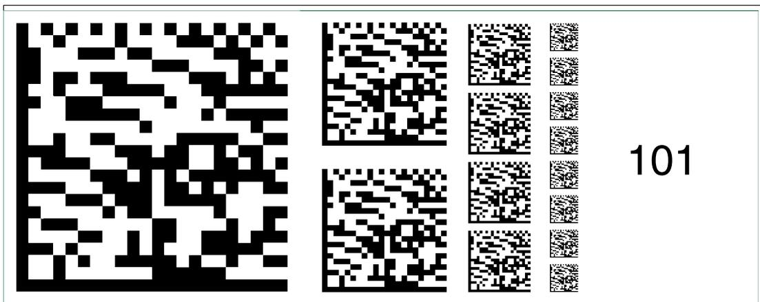
Figure 6.115 The code card "Fieldbus address 101" assigns the fieldbus address 101 to the device.
