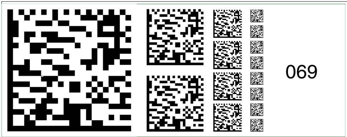
Figure 6.83 The code card "Fieldbus address 069" assigns the fieldbus address 069 to the device.
