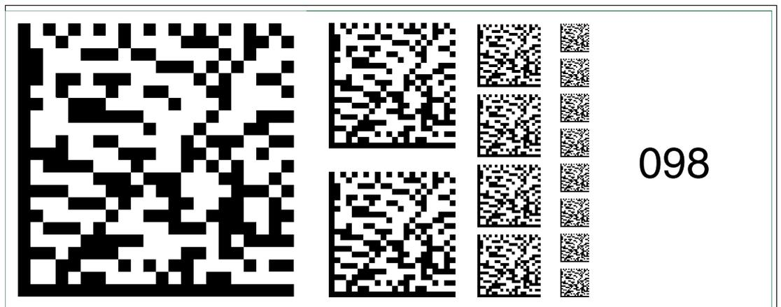
Figure 6.112 The code card "Fieldbus address 098" assigns the fieldbus address 098 to the device.
