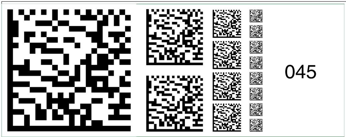
Figure 6.59 The code card "Fieldbus address 045" assigns the fieldbus address 045 to the device.
