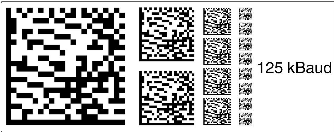
Figure 6.8 The code card assigns the 125 kBaud baud rate to the read head
