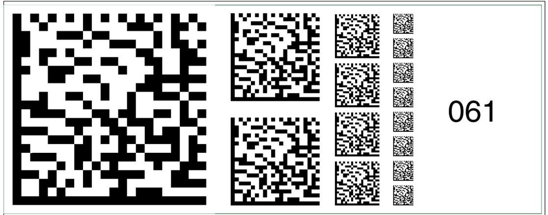
Figure 6.75 The code card "Fieldbus address 061" assigns the fieldbus address 061 to the device.
