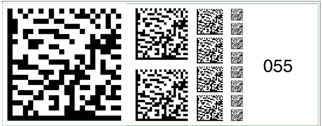
Figure 6.69 The code card "Fieldbus address 055" assigns the fieldbus address 055 to the device.
