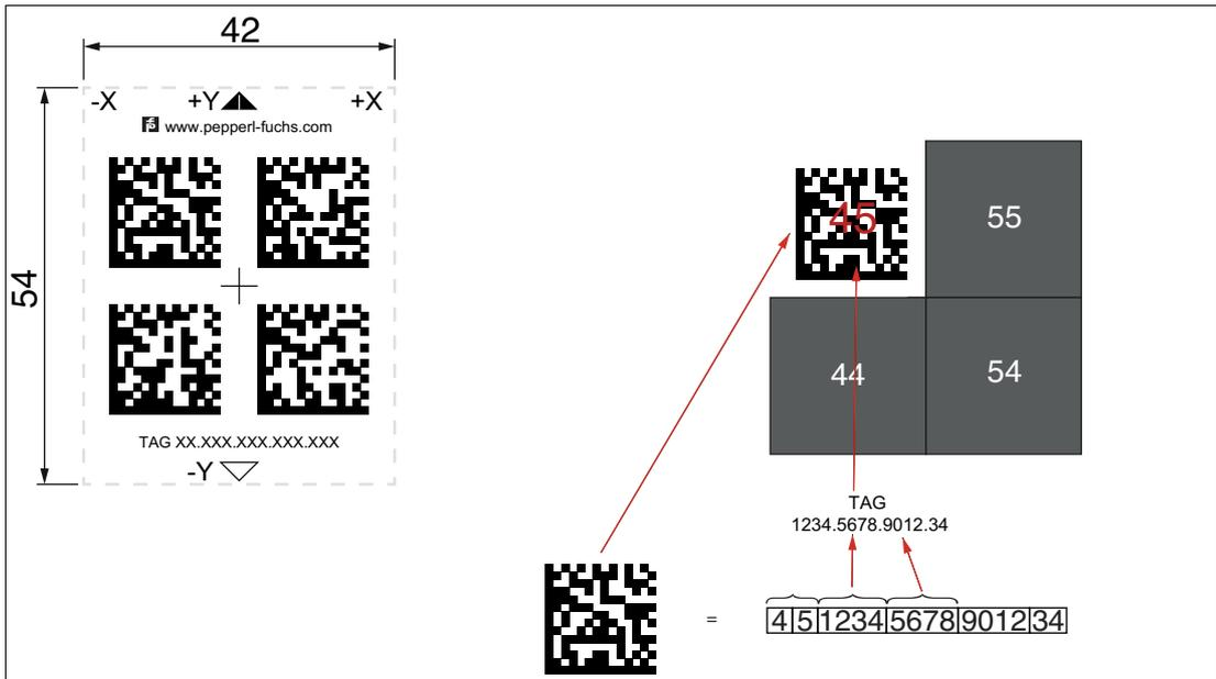
Figure 3.13 2x2 Data Matrix tag with number 12345678901234 and position information
