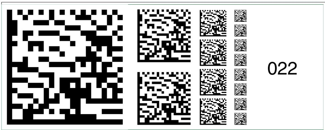
Figure 6.36 The code card "Fieldbus address 022" assigns the fieldbus address 022 to the device.
