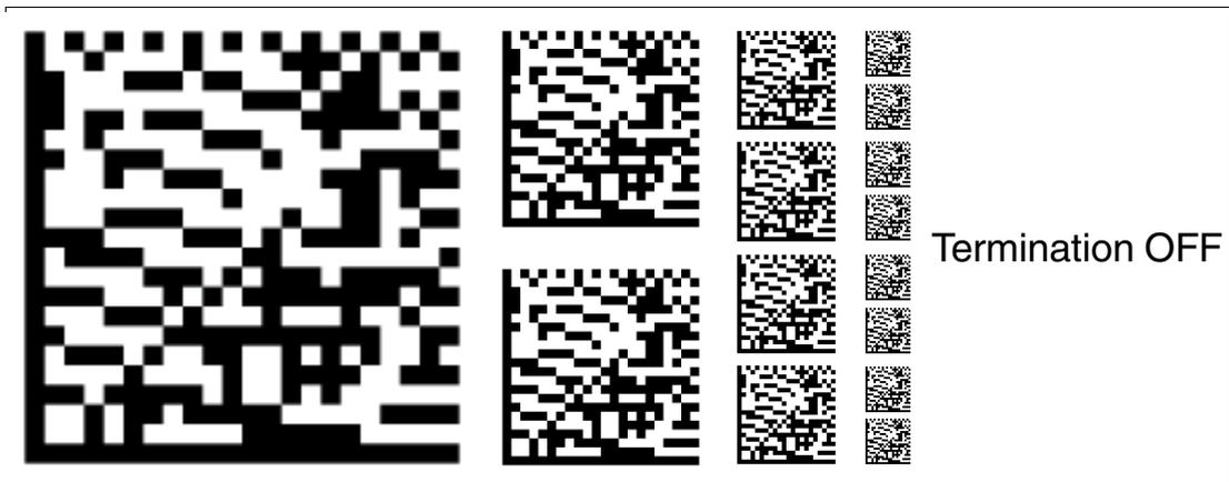
Figure 6.14 The Termination OFF code card deactivates the termination resistor on the bus.
