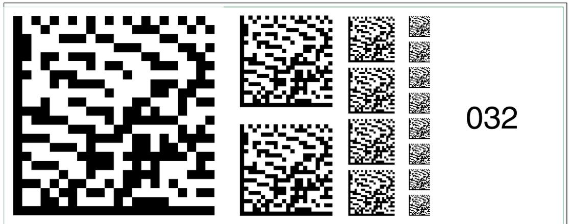
Figure 6.46 The code card "Fieldbus address 032" assigns the fieldbus address 032 to the device.
