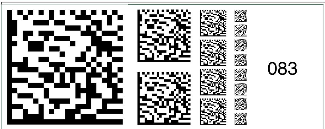
Figure 6.97 The code card "Fieldbus address 083" assigns the fieldbus address 083 to the device.
