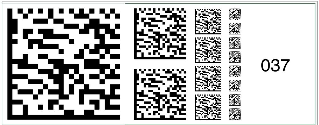
Figure 6.51 The code card "Fieldbus address 037" assigns the fieldbus address 037 to the device.
