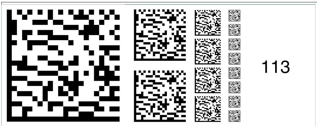
Figure 6.127 The code card "Fieldbus address 113" assigns the fieldbus address 113 to the device.
