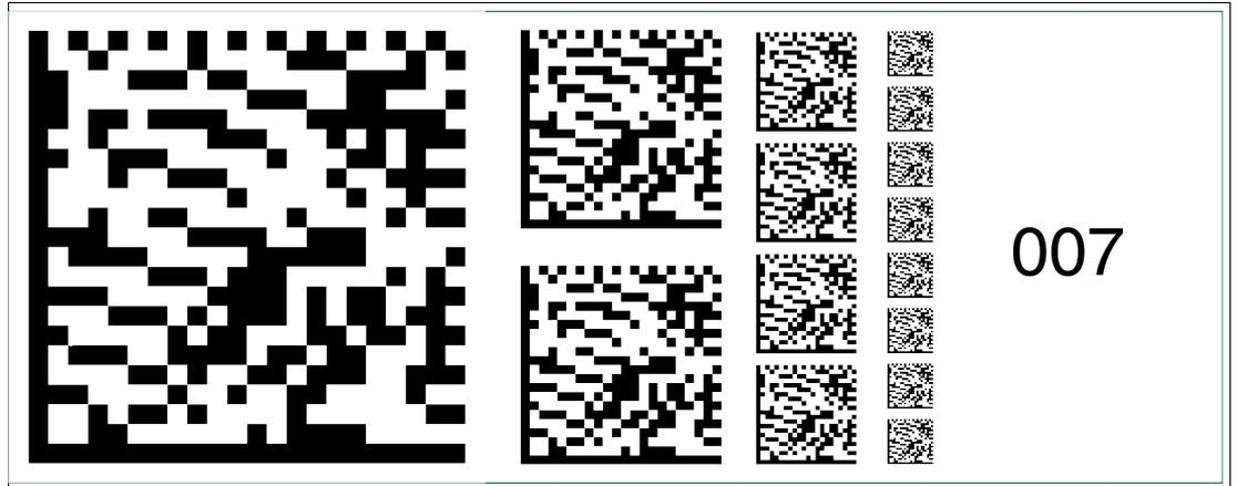
Figure 6.21 The code card "Fieldbus address 007" assigns the fieldbus address 007 to the device.
