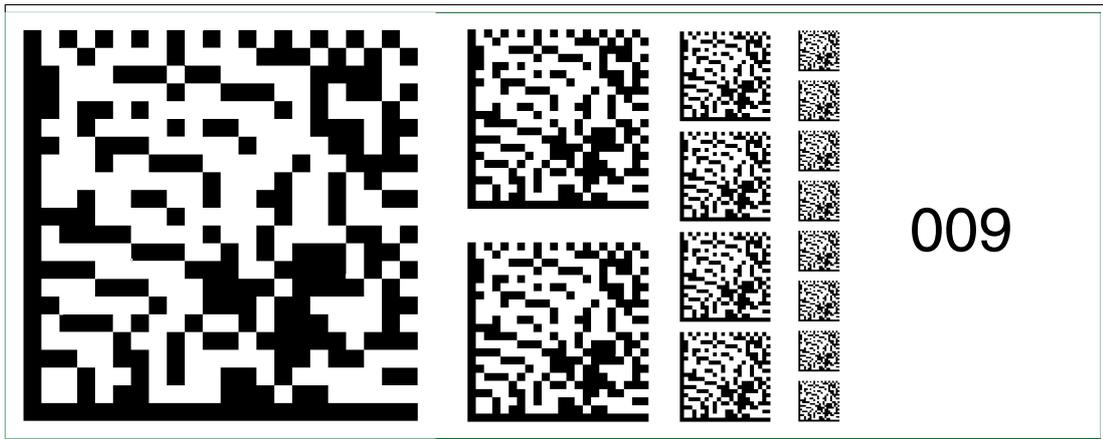
Figure 6.23 The code card "Fieldbus address 009" assigns the fieldbus address 009 to the device.
