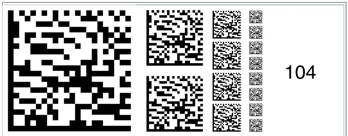
Figure 6.118 The code card "Fieldbus address 104" assigns the fieldbus address 104 to the device.
