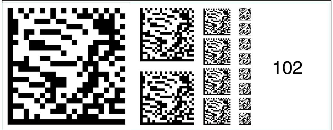
Figure 6.116 The code card "Fieldbus address 102" assigns the fieldbus address 102 to the device.
