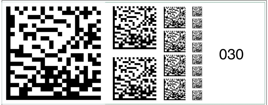
Figure 6.44 The code card "Fieldbus address 030" assigns the fieldbus address 030 to the device.
