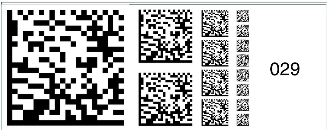
Figure 6.43 The code card "Fieldbus address 029" assigns the fieldbus address 029 to the device.
