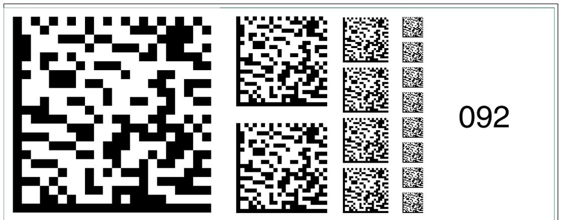
Figure 6.106 The code card "Fieldbus address 092" assigns the fieldbus address 092 to the device.
