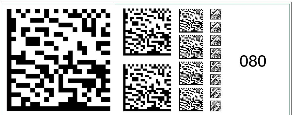
Figure 6.94 The code card "Fieldbus address 080" assigns the fieldbus address 080 to the device.
