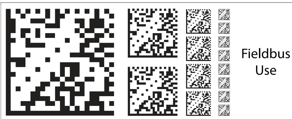
Figure 6.5 The code card "Fieldbus Use" adopts the modified configuration in the **volatile** working memory of the reading head and terminates external parameterization operating mode. The reading head then operates with this configuration. However, if the reading head is switched off and on again, the configuration is lost and the reading head operates with the last valid configuration that was saved. This function is used primarily for test purposes.
