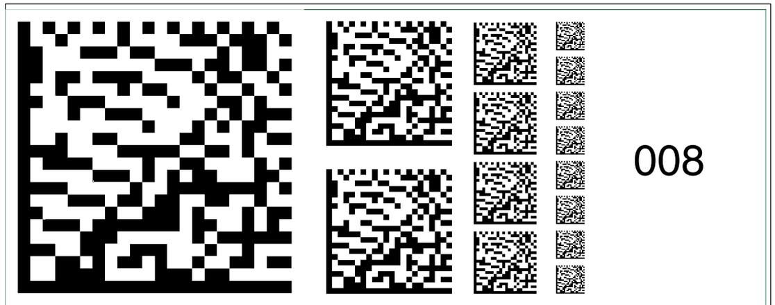
Figure 6.22 The code card "Fieldbus address 008" assigns the fieldbus address 008 to the device.
