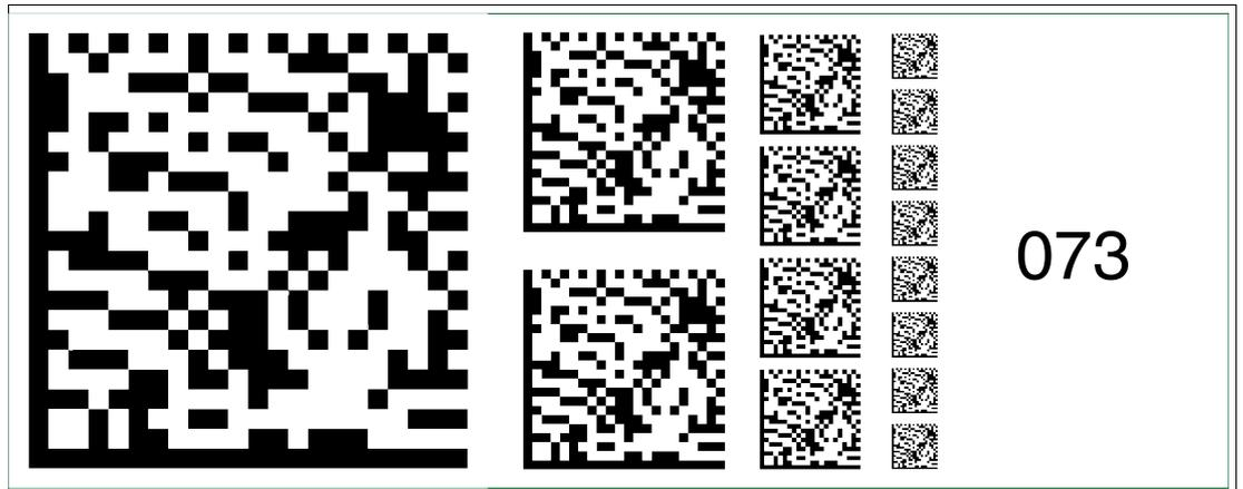
Figure 6.87 The code card "Fieldbus address 073" assigns the fieldbus address 073 to the device.
