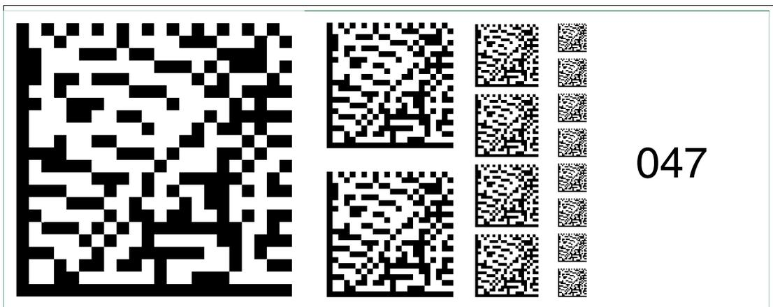
Figure 6.61 The code card "Fieldbus address 047" assigns the fieldbus address 047 to the device.
