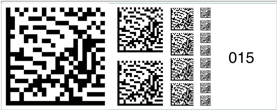
Figure 6.29 The code card "Fieldbus address 015" assigns the fieldbus address 015 to the device.
