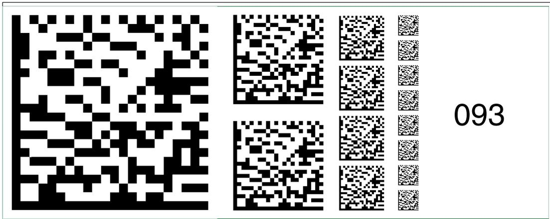
Figure 6.107 The code card "Fieldbus address 093" assigns the fieldbus address 093 to the device.
