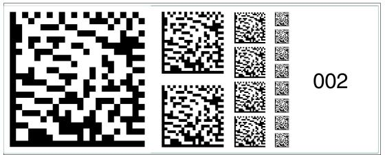
Figure 6.16 The code card "Fieldbus address 002" assigns the fieldbus address 002 to the device.
