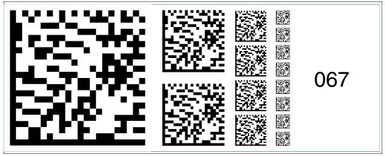
Figure 6.81 The code card "Fieldbus address 067" assigns the fieldbus address 067 to the device.
