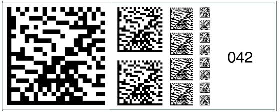
Figure 6.56 The code card "Fieldbus address 042" assigns the fieldbus address 042 to the device. **Fieldbus address 043**
