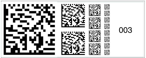
Figure 6.17 The code card "Fieldbus address 003" assigns the fieldbus address 003 to the device. Fieldbus address 004
