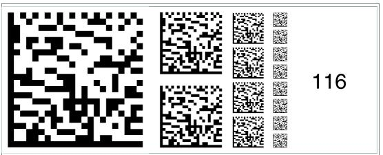
Figure 6.130 The code card "Fieldbus address 116" assigns the fieldbus address 116 to the device.
