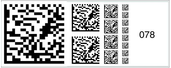
Figure 6.92 The code card "Fieldbus address 078" assigns the fieldbus address 078 to the device. **Fieldbus address 079**
