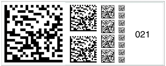
Figure 6.35 The code card "Fieldbus address 021" assigns the fieldbus address 021 to the device. **Fieldbus address 022**
