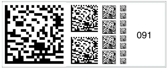
Figure 6.105 The code card "Fieldbus address 091" assigns the fieldbus address 091 to the device.
