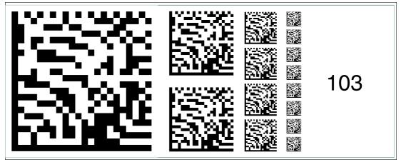
Figure 6.117 The code card "Fieldbus address 103" assigns the fieldbus address 103 to the device.
