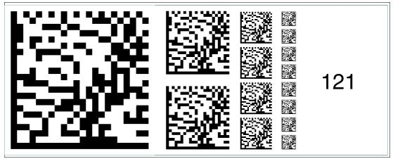
Figure 6.135 The code card "Fieldbus address 121" assigns the fieldbus address 121 to the device.
