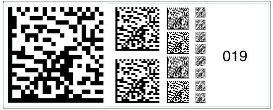
Figure 6.33 The code card "Fieldbus address 019" assigns the fieldbus address 019 to the device.
