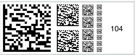
Figure 6.118 The code card "Fieldbus address 104" assigns the fieldbus address 104 to the device.
