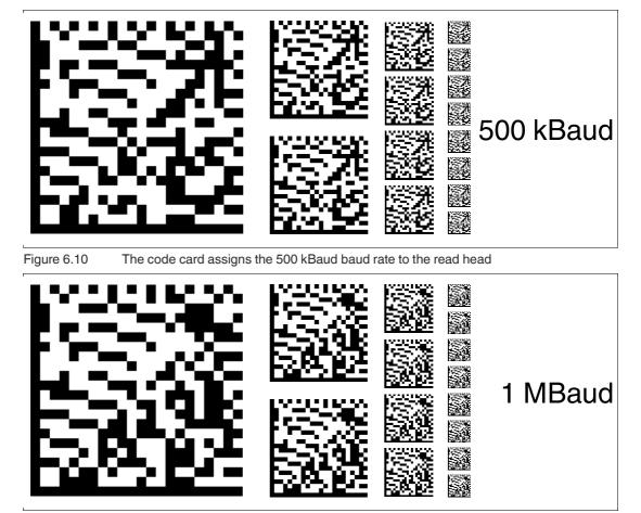
Figure 6.11 The code card assigns the 1 MBaud baud rate to the read head
