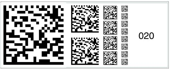
Figure 6.34 The code card "Fieldbus address 020" assigns the fieldbus address 020 to the device.
