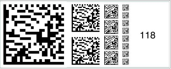
Figure 6.132 The code card "Fieldbus address 118" assigns the fieldbus address 118 to the device.
