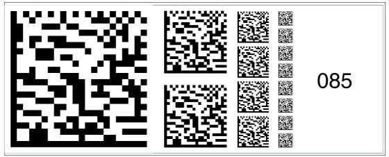
Figure 6.99 The code card "Fieldbus address 085" assigns the fieldbus address 085 to the device.
