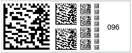
Figure 6.110 The code card "Fieldbus address 096" assigns the fieldbus address 096 to the device. **Fieldbus address 097**
