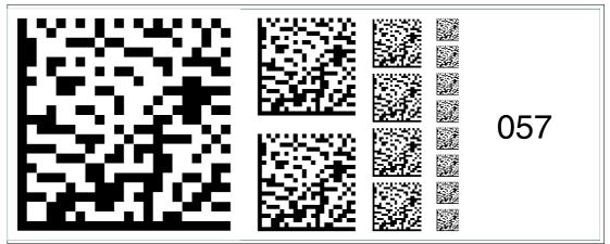
Figure 6.71 The code card "Fieldbus address 057" assigns the fieldbus address 057 to the device. Fieldbus address 058
