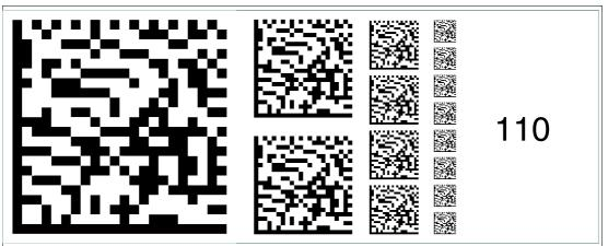
Figure 6.124 The code card "Fieldbus address 110" assigns the fieldbus address 110 to the device.
