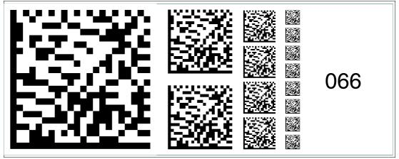
Figure 6.80 The code card "Fieldbus address 066" assigns the fieldbus address 066 to the device. Fieldbus address 067
