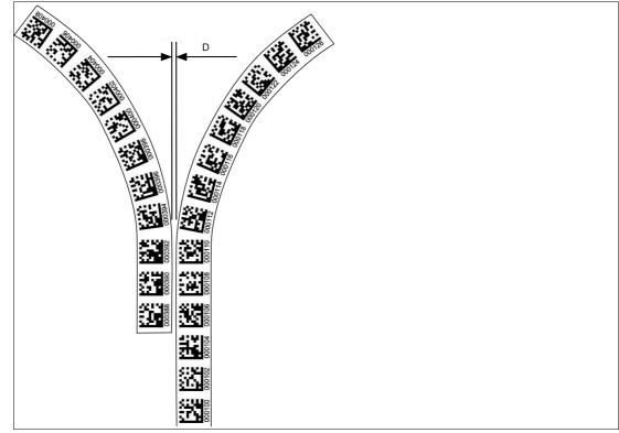
Figure 3.9 Distance: 0 mm  $\le$  D  $\le$  5 mm
