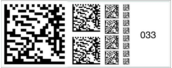
Figure 6.47 The code card "Fieldbus address 033" assigns the fieldbus address 033 to the device. Fieldbus address 034
