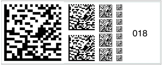
Figure 6.32 The code card "Fieldbus address 018" assigns the fieldbus address 018 to the device. **Fieldbus address 019**
