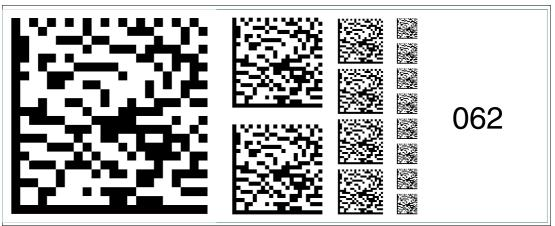
Figure 6.76 The code card "Fieldbus address 062" assigns the fieldbus address 062 to the device.
