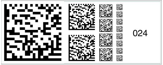
Figure 6.38 The code card "Fieldbus address 024" assigns the fieldbus address 024 to the device. Fieldbus address 025
