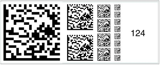
Figure 6.138 The code card "Fieldbus address 124" assigns the fieldbus address 124 to the device.
