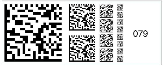
Figure 6.93 The code card "Fieldbus address 079" assigns the fieldbus address 079 to the device.
