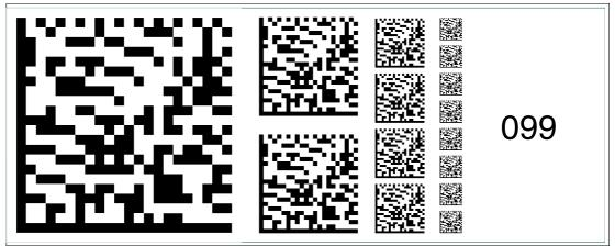
Figure 6.113 The code card "Fieldbus address 099" assigns the fieldbus address 099 to the device. **Fieldbus address 100**
