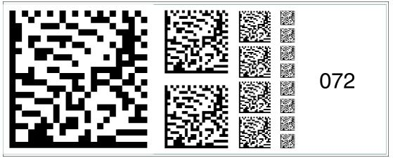
Figure 6.86 The code card "Fieldbus address 072" assigns the fieldbus address 072 to the device. **Fieldbus address 073**
