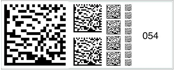
Figure 6.68 The code card "Fieldbus address 054" assigns the fieldbus address 054 to the device. **Fieldbus address 055**
