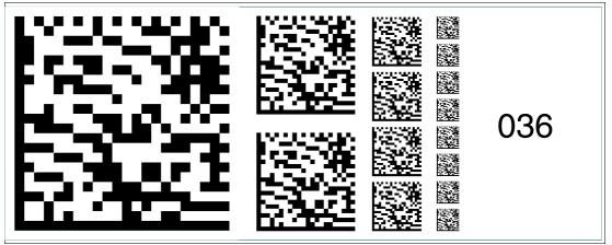
Figure 6.50 The code card "Fieldbus address 036" assigns the fieldbus address 036 to the device. Fieldbus address 037
