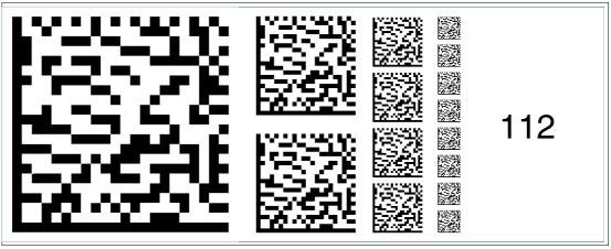
Figure 6.126 The code card "Fieldbus address 112" assigns the fieldbus address 112 to the device.
