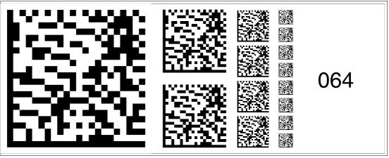
Figure 6.78 The code card "Fieldbus address 064" assigns the fieldbus address 064 to the device.
