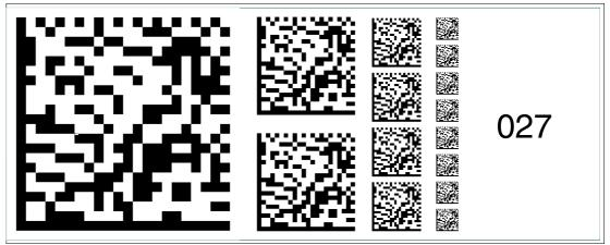
Figure 6.41 The code card "Fieldbus address 027" assigns the fieldbus address 027 to the device. **Fieldbus address 028**
