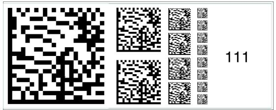
Figure 6.125 The code card "Fieldbus address 111" assigns the fieldbus address 111 to the device. **Fieldbus address 112**
