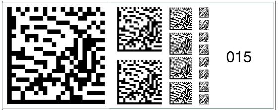
Figure 6.29 The code card "Fieldbus address 015" assigns the fieldbus address 015 to the device. Fieldbus address 016
