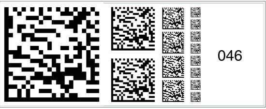
Figure 6.60 The code card "Fieldbus address 046" assigns the fieldbus address 046 to the device.
