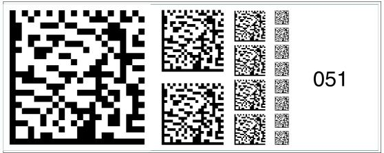
Figure 6.65 The code card "Fieldbus address 051" assigns the fieldbus address 051 to the device. Fieldbus address 052
