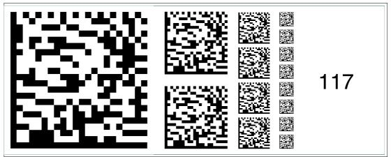
Figure 6.131 The code card "Fieldbus address 117" assigns the fieldbus address 117 to the device. **Fieldbus address 118**
