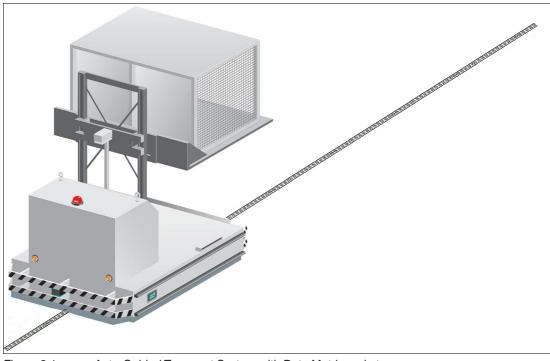
Figure 2.1 Auto-Guided Transport System with Data Matrix code tape
