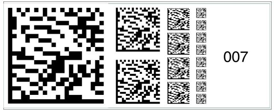
Figure 6.21 The code card "Fieldbus address 007" assigns the fieldbus address 007 to the device.
