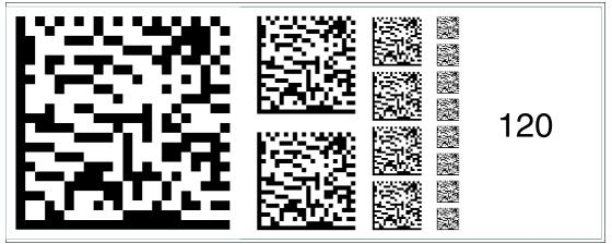
Figure 6.134 The code card "Fieldbus address 120" assigns the fieldbus address 120 to the device. **Fieldbus address 121**
