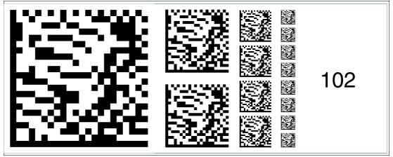
Figure 6.116 The code card "Fieldbus address 102" assigns the fieldbus address 102 to the device. **Fieldbus address 103**
