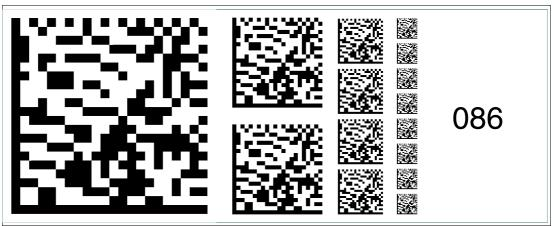
Figure 6.100 The code card "Fieldbus address 086" assigns the fieldbus address 086 to the device.
