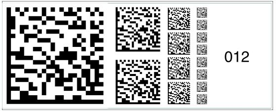
Figure 6.26 The code card "Fieldbus address 012" assigns the fieldbus address 012 to the device. **Fieldbus address 013**
