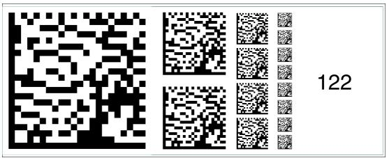
Figure 6.136 The code card "Fieldbus address 122" assigns the fieldbus address 122 to the device.
