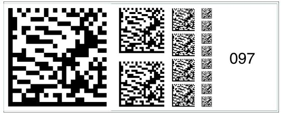
Figure 6.111 The code card "Fieldbus address 097" assigns the fieldbus address 097 to the device.
