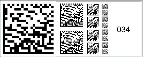
Figure 6.48 The code card "Fieldbus address 034" assigns the fieldbus address 034 to the device.
