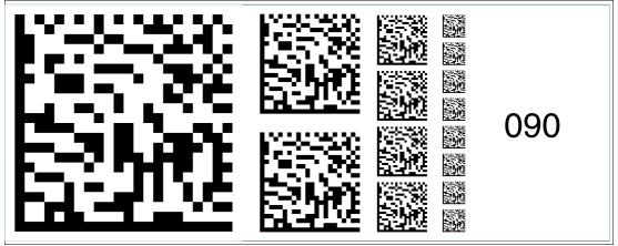
Figure 6.104 The code card "Fieldbus address 090" assigns the fieldbus address 090 to the device. **Fieldbus address 091**
