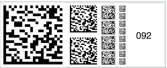
Figure 6.106 The code card "Fieldbus address 092" assigns the fieldbus address 092 to the device.
