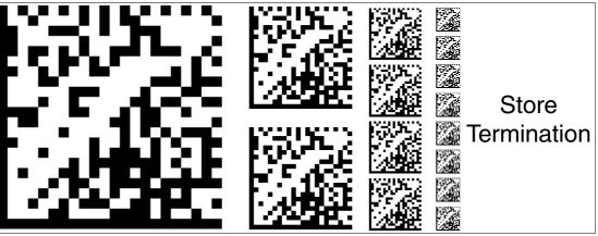
Figure 6.12 The "Store Termination" code card saves the changes made to the termination resistor and ends the parameterization mode.
