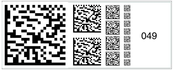
Figure 6.63 The code card "Fieldbus address 049" assigns the fieldbus address 049 to the device.
