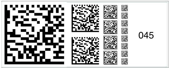
Figure 6.59 The code card "Fieldbus address 045" assigns the fieldbus address 045 to the device. **Fieldbus address 046**
