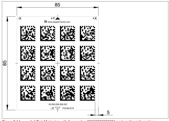
Figure 3.14 4x4 DataMatrix tag with the number 000000000001 and position information
