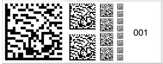
Figure 6.15 The code card "Fieldbus address 001" assigns the fieldbus address 001 to the device.
