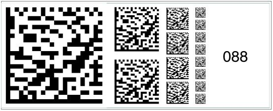
Figure 6.102 The code card "Fieldbus address 088" assigns the fieldbus address 088 to the device.
