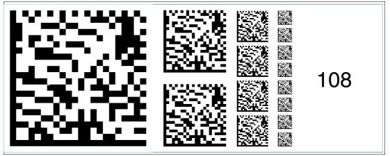
Figure 6.122 The code card "Fieldbus address 108" assigns the fieldbus address 108 to the device. **Fieldbus address 109**
