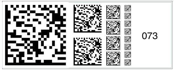
Figure 6.87 The code card "Fieldbus address 073" assigns the fieldbus address 073 to the device.
