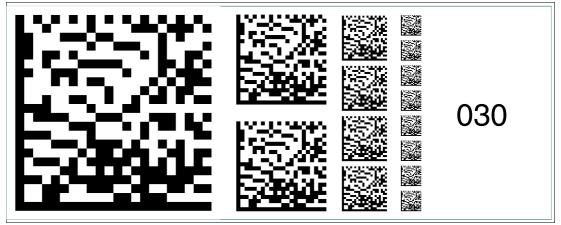
Figure 6.44 The code card "Fieldbus address 030" assigns the fieldbus address 030 to the device. **Fieldbus address 031**
