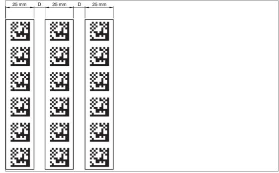
The distance between a Data Matrix position code and a Data Matrix control code must be between 0 mm and 5 mm.
