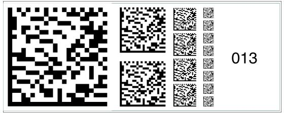
Figure 6.27 The code card "Fieldbus address 013" assigns the fieldbus address 013 to the device.
