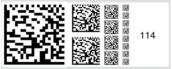
Figure 6.128 The code card "Fieldbus address 114" assigns the fieldbus address 114 to the device. **Fieldbus address 115**
