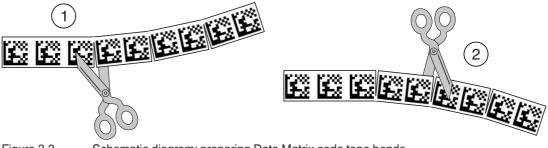
Figure 3.3 Schematic diagram: preparing Data Matrix code tape bends
