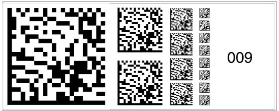
Figure 6.23 The code card "Fieldbus address 009" assigns the fieldbus address 009 to the device. Fieldbus address 010
