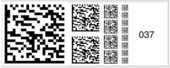
Figure 6.51 The code card "Fieldbus address 037" assigns the fieldbus address 037 to the device.
