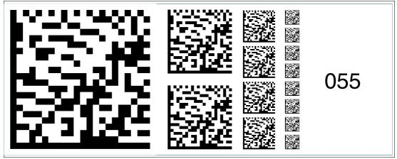
Figure 6.69 The code card "Fieldbus address 055" assigns the fieldbus address 055 to the device.
