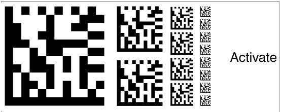
Figure 6.1 The "ACTIVATE" code card is used to activate external parameterization operating mode. To enter the parameterization operating mode the codecart "user" has to be read by the reading head.
