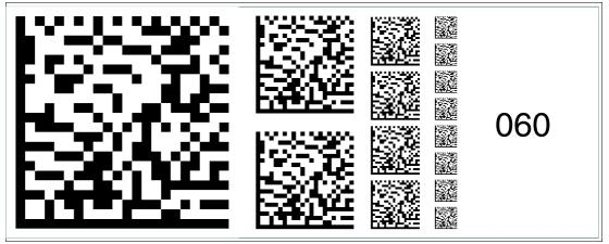
Figure 6.74 The code card "Fieldbus address 060" assigns the fieldbus address 060 to the device. **Fieldbus address 061**
