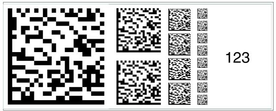
Figure 6.137 The code card "Fieldbus address 123" assigns the fieldbus address 123 to the device. **Fieldbus address 124**
