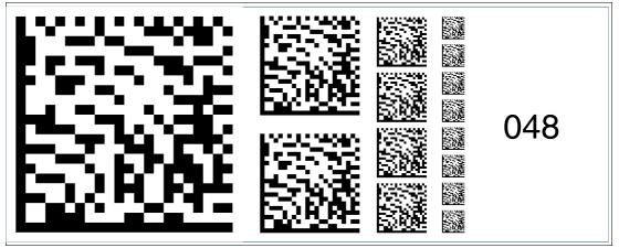
Figure 6.62 The code card "Fieldbus address 048" assigns the fieldbus address 048 to the device. **Fieldbus address 049**
