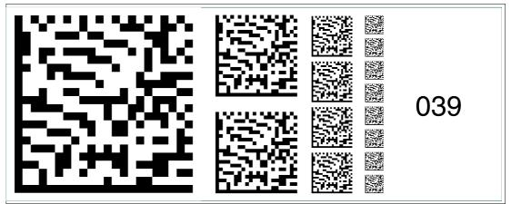
Figure 6.53 The code card "Fieldbus address 039" assigns the fieldbus address 039 to the device. **Fieldbus address 040**
