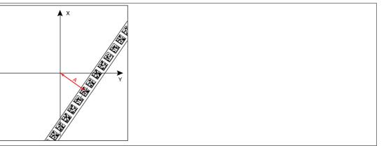
Figure 3.5 Distance A for Data Matrix code tape
