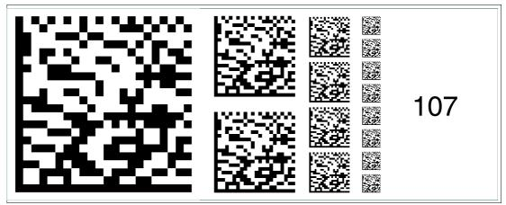
Figure 6.121 The code card "Fieldbus address 107" assigns the fieldbus address 107 to the device.
