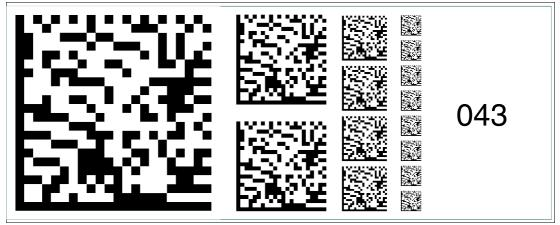
Figure 6.57 The code card "Fieldbus address 043" assigns the fieldbus address 043 to the device.
