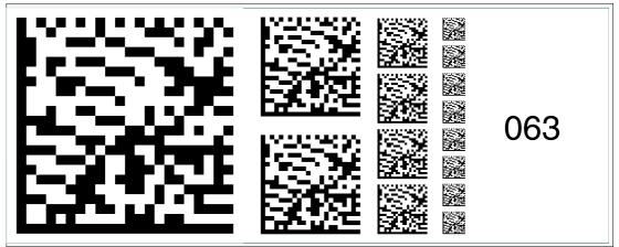
Figure 6.77 The code card "Fieldbus address 063" assigns the fieldbus address 063 to the device. Fieldbus address 064
