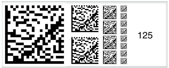
Figure 6.139 The code card "Fieldbus address 125" assigns the fieldbus address 125 to the device.
