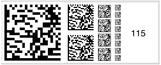
Figure 6.129 The code card "Fieldbus address 115" assigns the fieldbus address 115 to the device.
