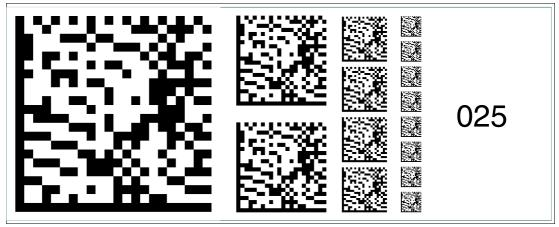
Figure 6.39 The code card "Fieldbus address 025" assigns the fieldbus address 025 to the device.
