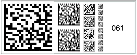
Figure 6.75 The code card "Fieldbus address 061" assigns the fieldbus address 061 to the device.
