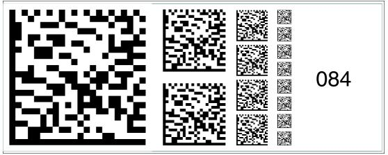
Figure 6.98 The code card "Fieldbus address 084" assigns the fieldbus address 084 to the device. **Fieldbus address 085**
