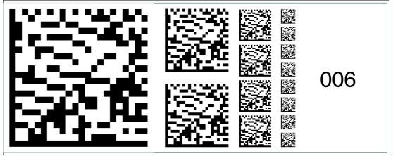
Figure 6.20 The code card "Fieldbus address 006" assigns the fieldbus address 006 to the device. **Fieldbus address 007**
