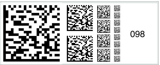
Figure 6.112 The code card "Fieldbus address 098" assigns the fieldbus address 098 to the device.
