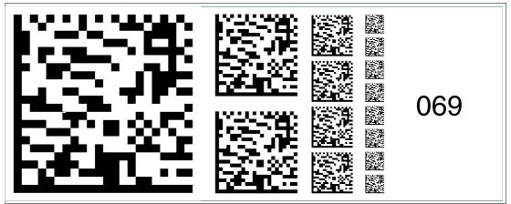
Figure 6.83 The code card "Fieldbus address 069" assigns the fieldbus address 069 to the device. **Fieldbus address 070**
