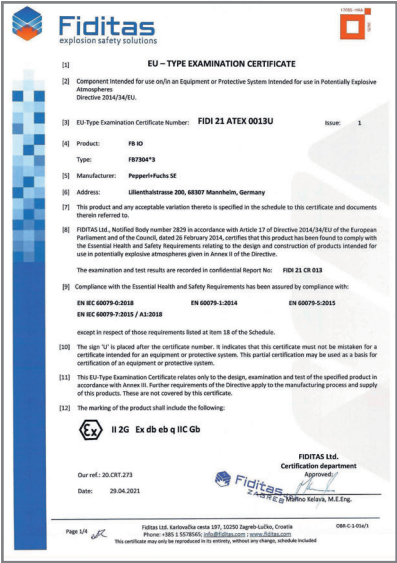
Figure 3.6 Example: Title page of the certificate FIDI 21 ATEX 0013 U for a component that is by itself not ready for use in potentially explosive atmospheres
