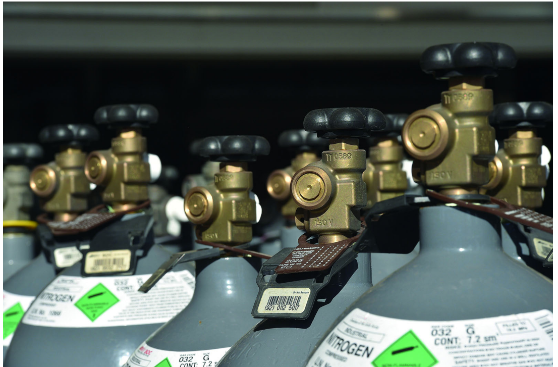
Figure 13 Example of bottled inert gas: Nitrogen
