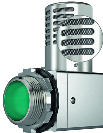
Figure 7 Example of pressure relief vent spark and particle barrier Pepperl+Fuchs EPV 7500: The spark and particle barrier consists of a wire mesh
