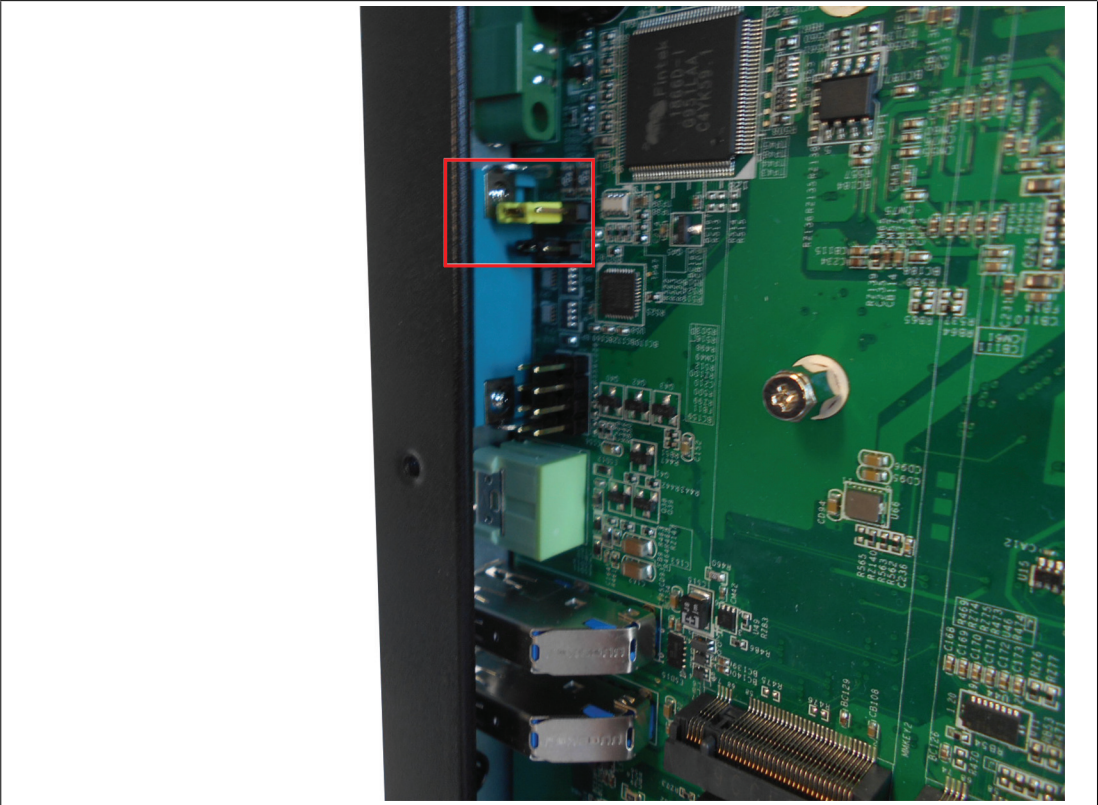
Figure 5.4 (2) Jumper 1 (yellow) DSR (Default Setting) or Power Jumper 2 Set 5V (Default) or 12V
