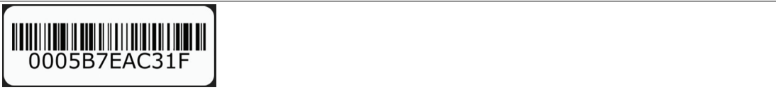
Figure 3.9 Find the MAC ID on top of the ports that describes a worldwide unique hardware address of a single network adapter. The physical address is used to identify a device in computer networks.
