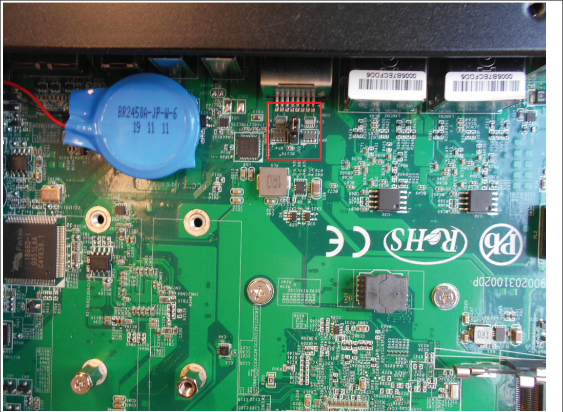
Figure 5.5 (3) Jumper 3 (black) DSR (Default Setting) or Power
