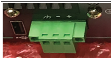
Figure 5.3 Power connector is included in the delivery.
