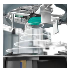
Clear identification of green tires before insertion into the vulcanization press. Damage to the press and tires caused by mixing up the tires is prevented. Perfectly suitable for difficult ambient conditions (heat, limited installation space, etc.).
