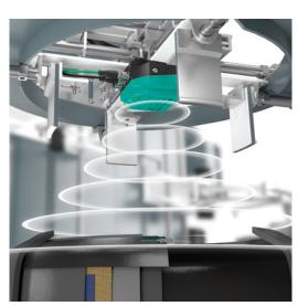
Clear identification of green tires before insertion into the vulcanization press. Damage to the press and tires caused by mixing up the tires is prevented. Perfectly suitable for difficult ambient conditions (heat, limited installation space, etc.).
