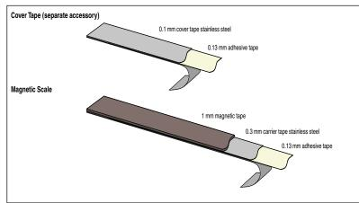
A magnetically permeable steel band to cover the elastomer layer is available as an option. The band can be assembled at the factory or ordered for retrofitting.
