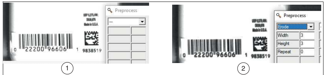
Figure 7.22 Eroding 1. Original image 2. Eroded image
