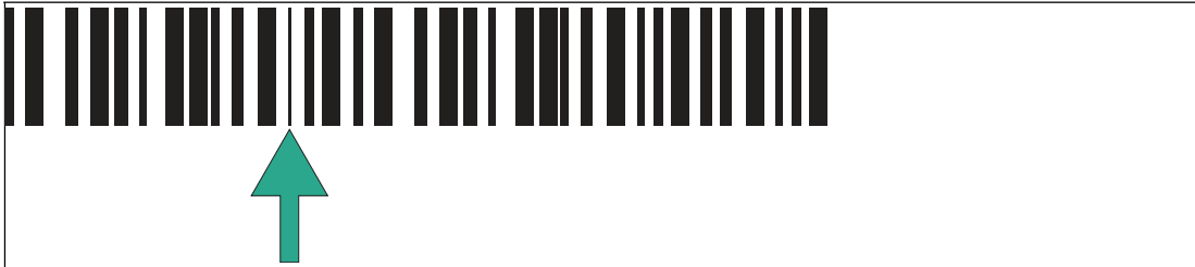
Figure 4.4 Module size = minimum bar width
