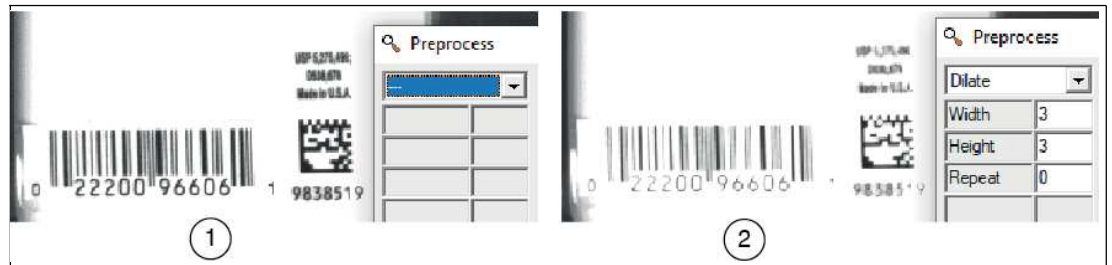
Figure 7.21 Dilate function 1. Original image 2. Dilate Preprocessing Filter
