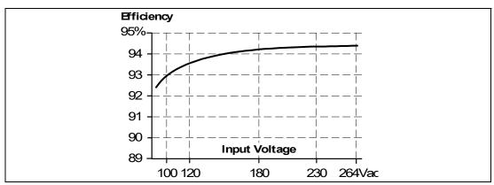
Figure 11.3 Efficiency vs. input voltage at 24V, 5A, typ.
