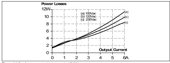
Figure 11.2 Losses vs. output current at 24V, typ.
