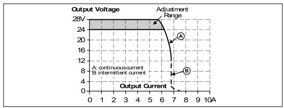
Figure 8.1 Output voltage vs. output current, typ.
