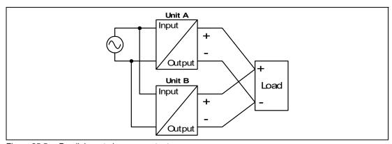
Figure 25.5 Parallel use to increase output power
