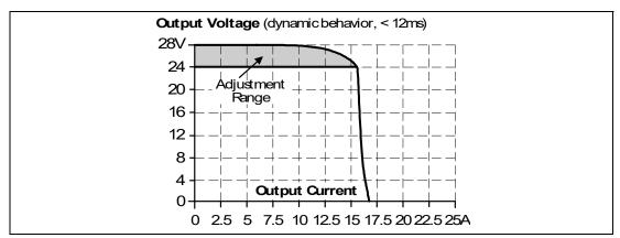
Figure 8.2 Dynamic output current capability, typ.
