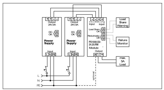
Figure 25.6 1+1 redundant configuration with active load share for 5A load current with a dual redundancy module
