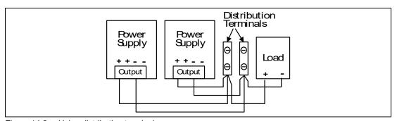
Figure 14.2 Using distribution terminals
