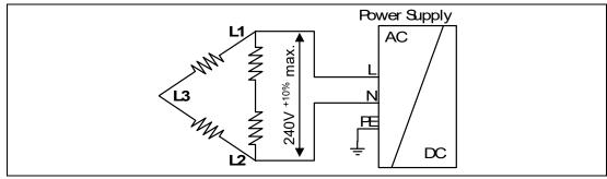
Figure 25.8 Two phases operation
