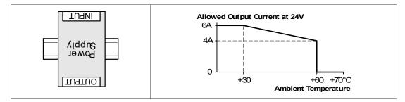
Figure 25.10 Mounting orientation B (upside down)
