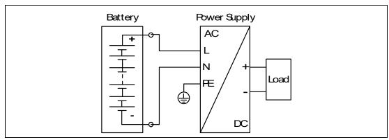
Figure 6.1 Wiring for DC Input
