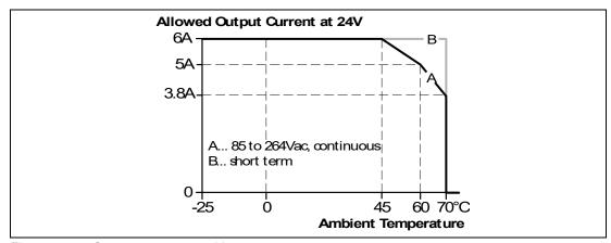
Figure 18.1 Output current vs. ambient temp.
