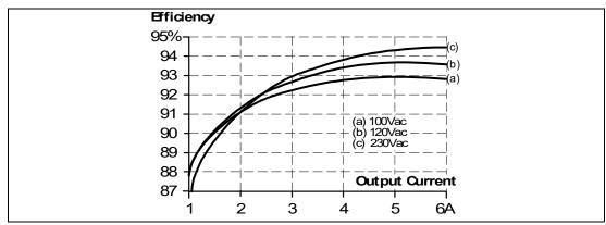
Figure 11.1 Efficiency vs. output current at 24V, typ.
