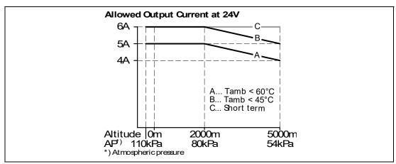
Figure 18.2 Output current vs. altitude
