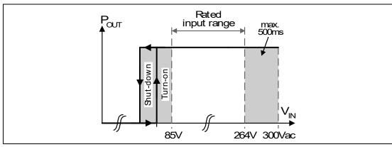
Figure 5.1 Input voltage range
