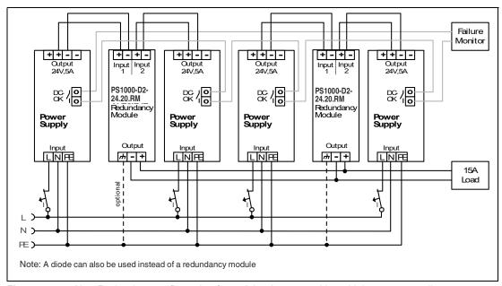
Figure 25.7 N+1 Redundant configuration for 15A load current with multiple power supplies and redundancy modules
