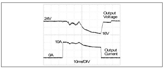
Figure 25.1 10A peak current for 50ms, typ. (2x the nominal current)
