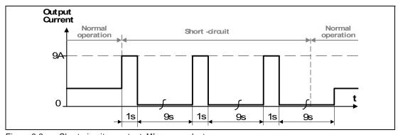
Figure 8.3 Short-circuit on output, **Hiccup** mode, typ.
