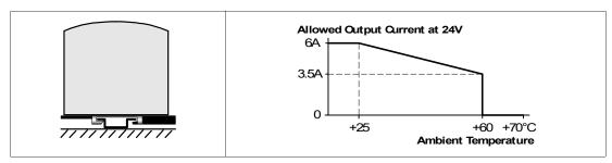
Figure 25.11 Mounting orientation C (table-top mounting)
