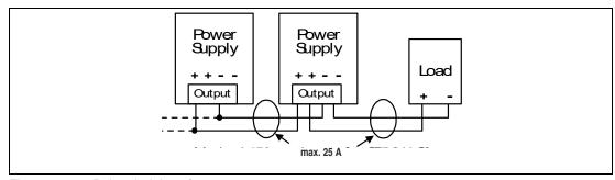
Figure 14.1 Daisy chaining of outputs
