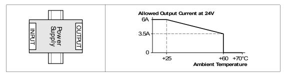
Figure 25.12 Mounting orientation D (horizontal cw)
