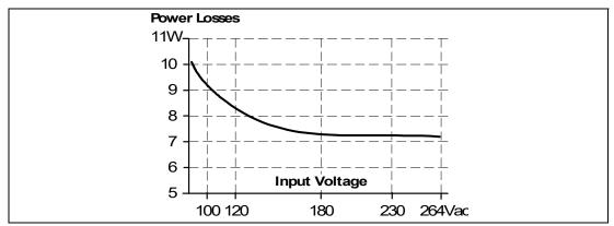
Figure 11.4 Losses vs. input voltage at 24V, 5A, typ.
