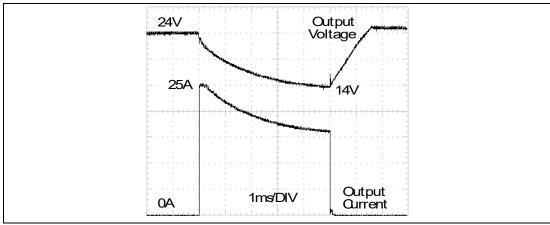
Figure 25.2 25A peak current for 5ms, typ. (5x the nominal current)
