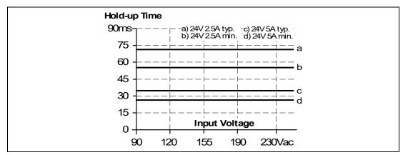
Figure 9.1 Hold-up time vs. input voltage
