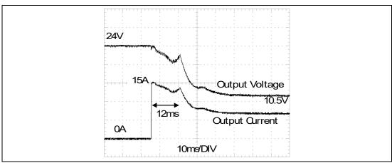
Figure 25.3 15A peak current for 12ms, typ. (3x the nominal current)
