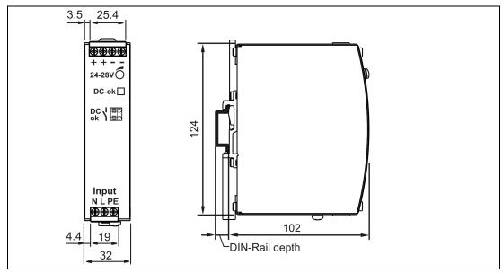
Figure 23.1 Device dimensions, all dimensions in mm
