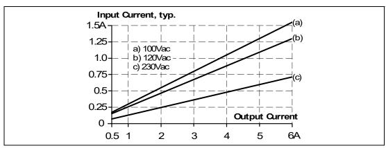
Figure 5.3 Input current vs. output current at 24V output voltage
