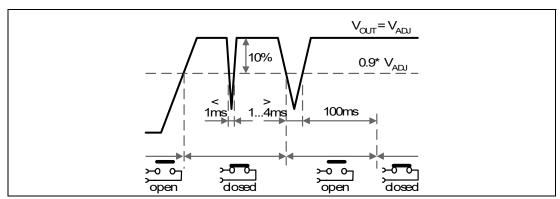
Figure 10.1 DC-OK relay contact behavior
