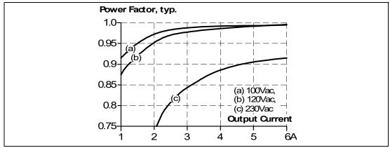
Figure 5.4 Power factor vs. output current at 24V output voltage
