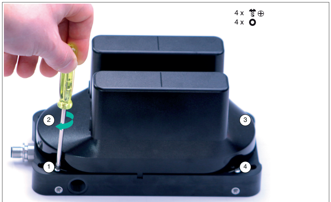
Figure 5.7 Mounting the protective cover
