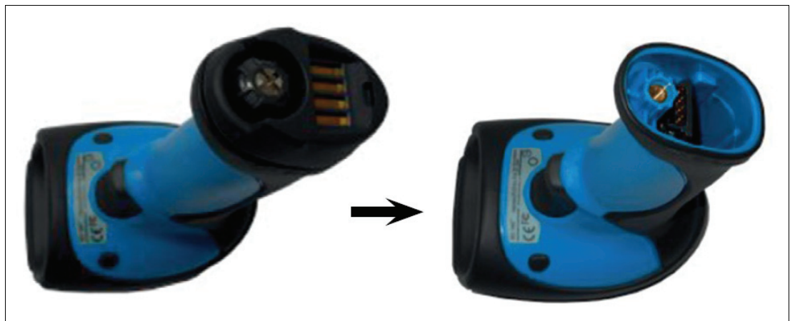
Figure 5.1 Removing the battery compartment lid.
