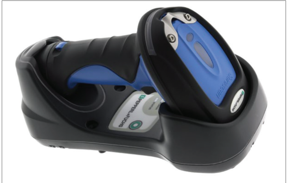
Figure 5.8 Inserting the scanner into the base station.
