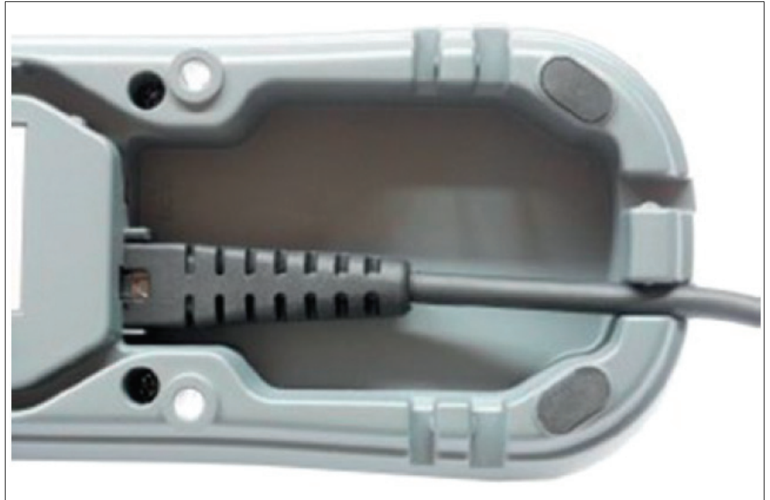
Figure 5.10 Connecting the RJ50 cable to the base station. The handheld reader is placed in the charger. The underside of the handle is used first to ensure that the charging contacts are properly connected. The LED light on the scanner head indicates successful charging.
