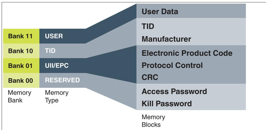
The memory of an EPC Gen2 (ISO/IEC 18000-63) tag is split into four memory banks. The main contents of these memory banks are:
