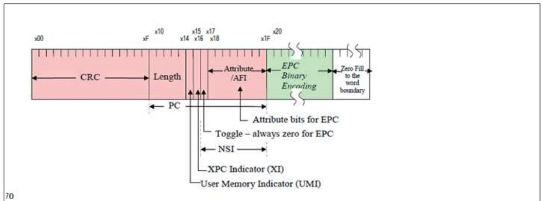
The first data word of the EPC memory bank contains the CRC checksum. This checksum is generated by the tag and transmitted when the memory bank is read out.
