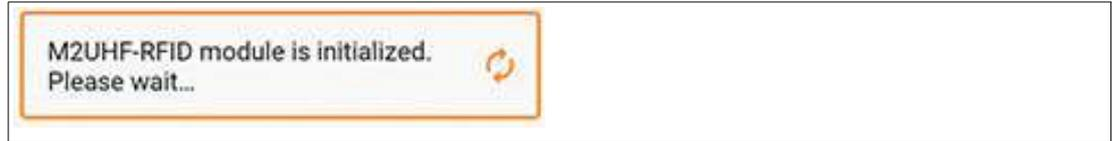
The module is always switched off to save power when the screen is switched off or the handheld is placed in idle mode. The module is switched on again and initialized when the handheld is reactivated.
