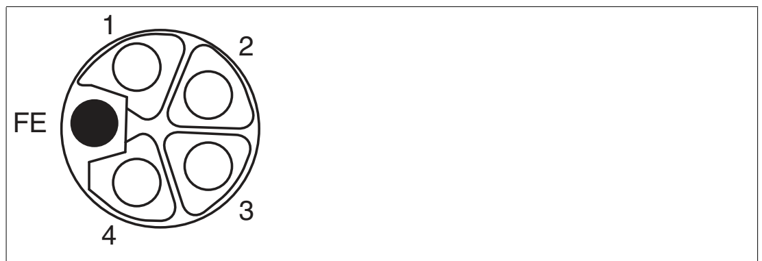
Figure 3.5 Schematic drawing of M12 L-encoding (socket); port X04 (OUT)
