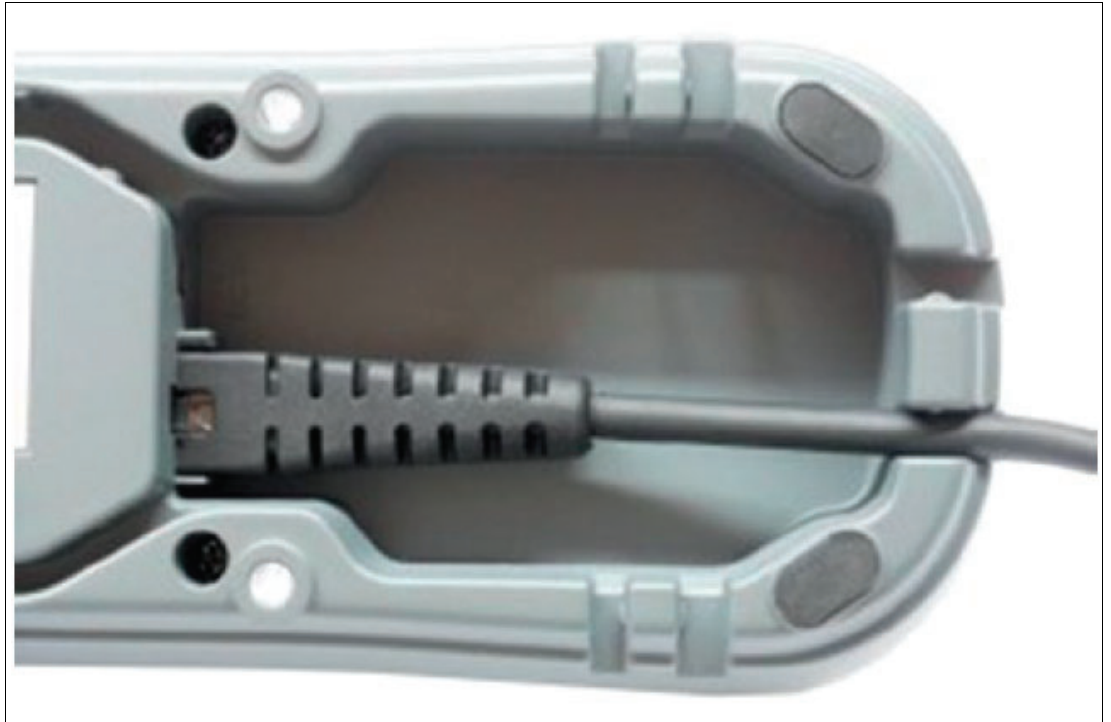
Figure 5.10 Connecting the RJ50 cable to the base station
