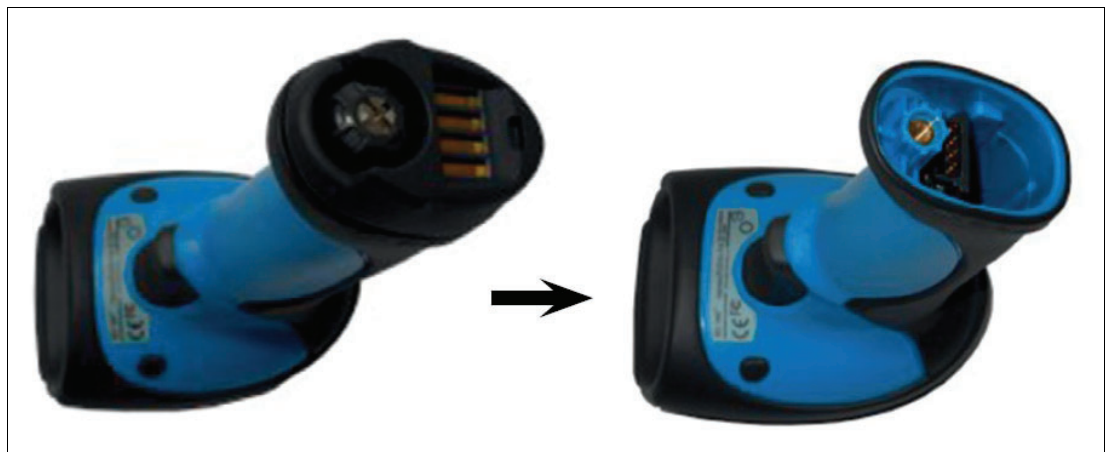
Figure 5.1 Removing the battery compartment lid
