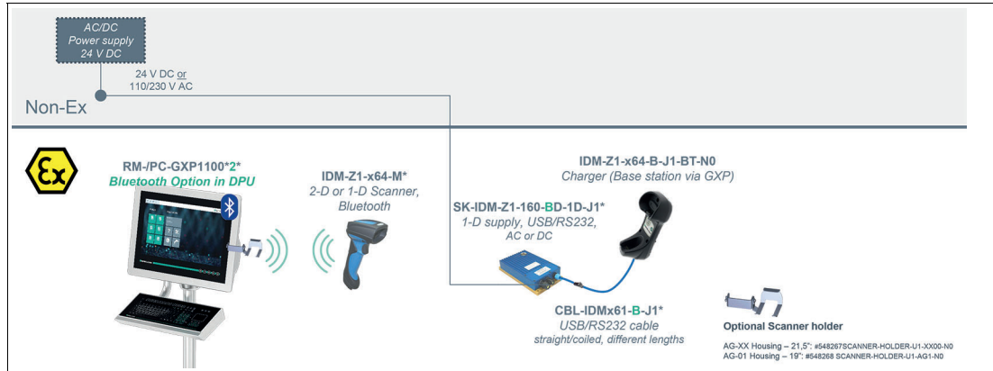
Figure 4.2 System structure 2 - scanner with base station connected to VisuNet GXP
