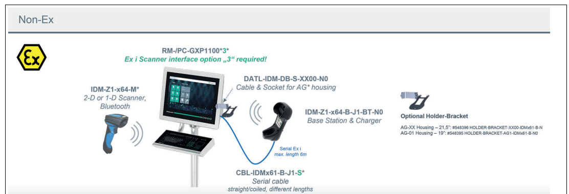
Figure 4.1 System structure 1 - Charger and base station connected to internal GXP "3" Ex i scanner interface
