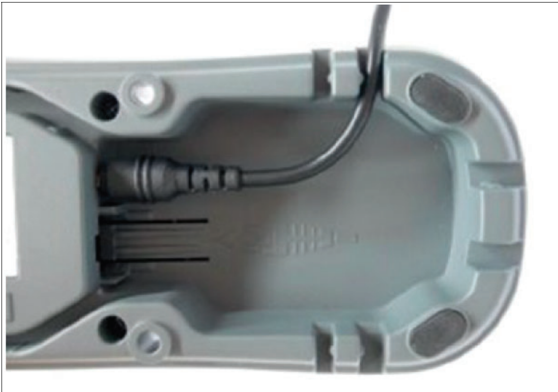
Figure 5.9 Connecting the power supply for the non-explosion-hazardous base station
