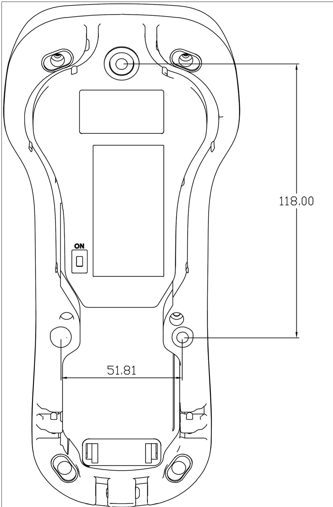
Figure 3.1 Hole pattern spacing of the IDM base station for wall mounting
