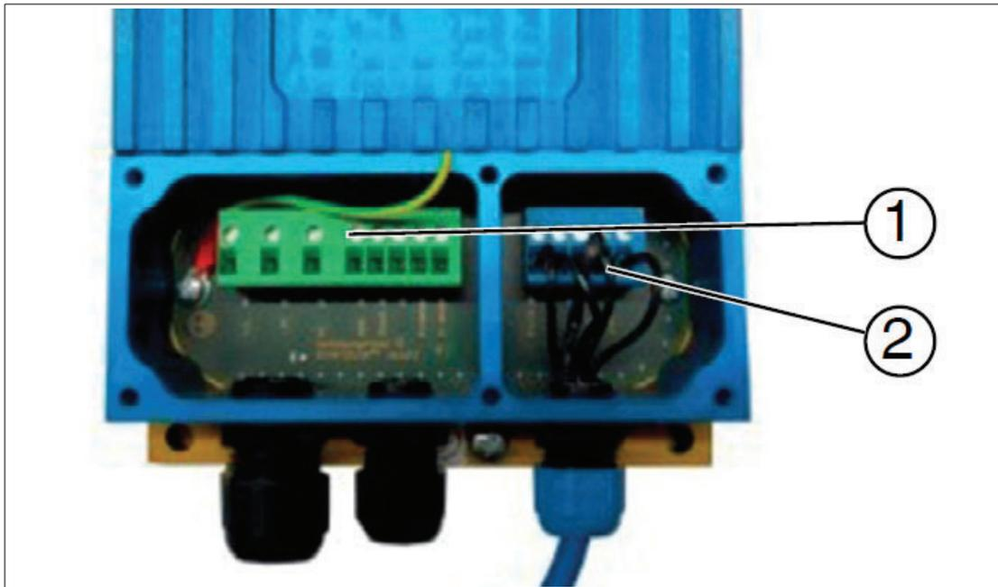
Figure 5.16 Supply module terminal compartment
