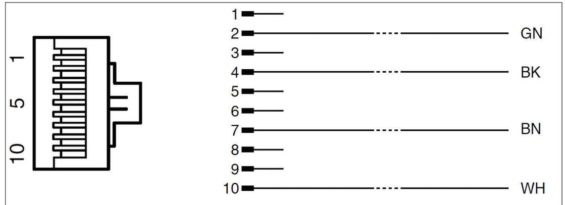
Figure 5.20 RJ45 plug - connection layout
