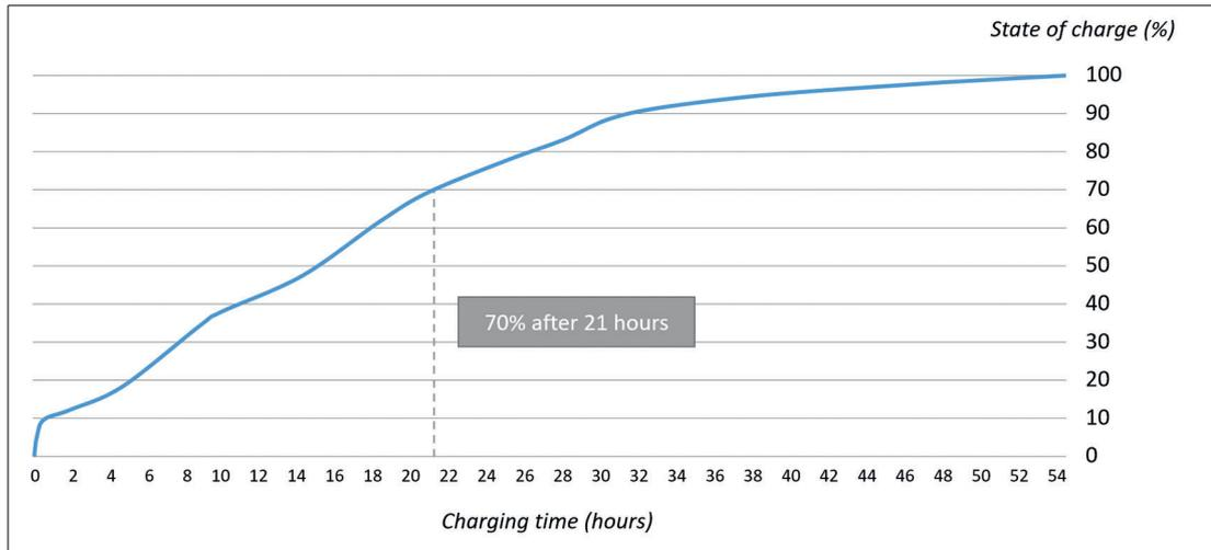
Figure 3.4 To reach a charging level of 100% in this setup, it requires 54 hours of charging time.
