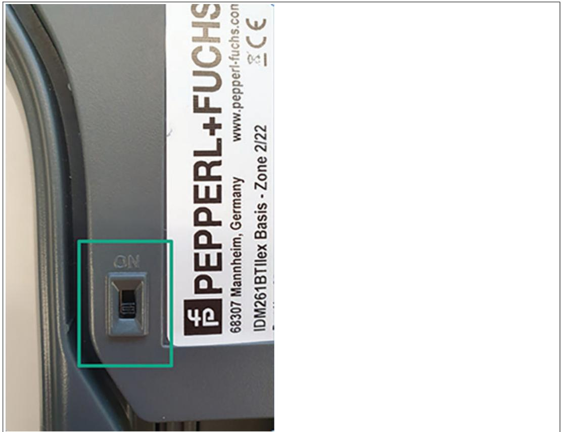
Figure 4.7 When USB 3.0 is available set the USB bus power switch to "ON". Then connect the cradle and host device via a USB cable.
