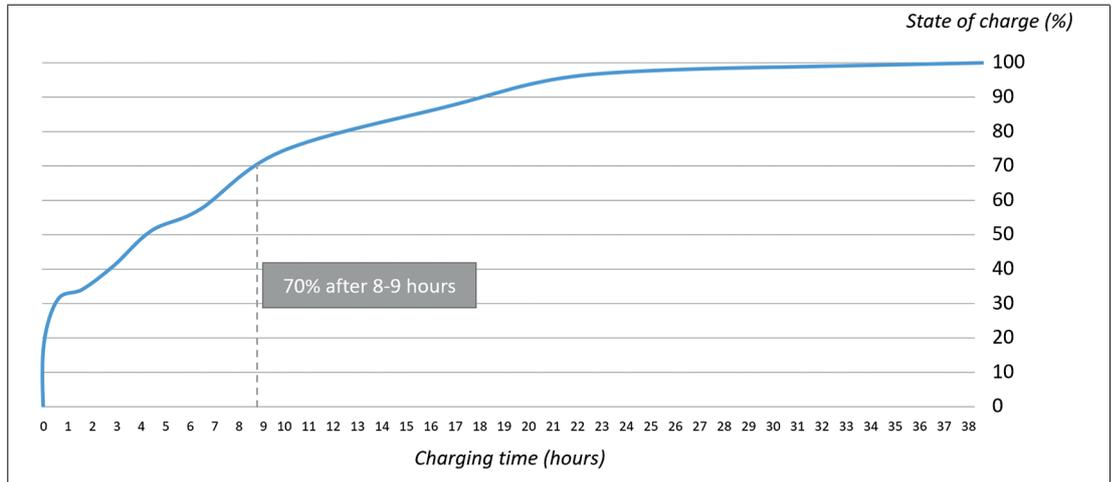
Figure 3.2 To reach a charging level of 100% in this setup, it requires 38 hours of charging time.
