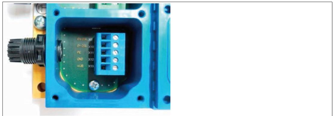
Figure 5.18 Intrinsically safe terminal compartment of the supply module after removing the connector connection cores
