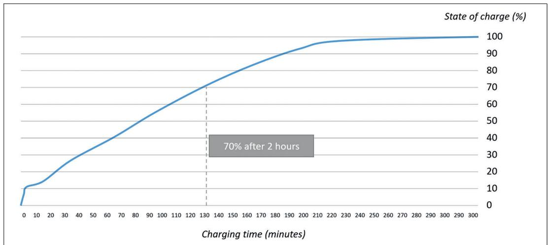
Figure 3.3 To reach a charging level of 100% in this setup, it requires 5 hours of charging time.
