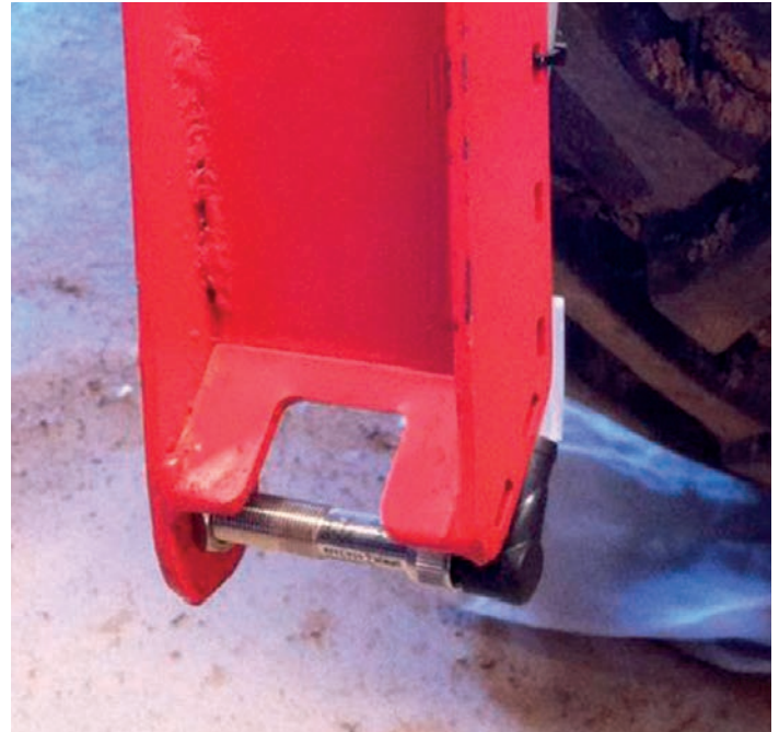
Each wheel is equipped with an ultrasonic sensor that continuously detects the distance between the wheel and the strawberry field row.
