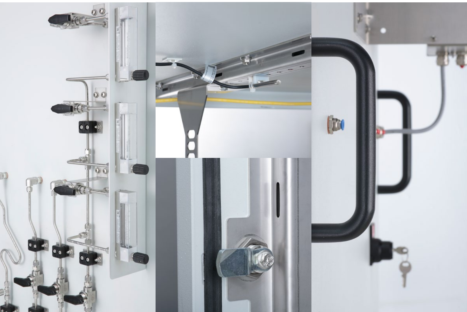
Detailed shots of the solution: special stainless steel tubes to the analyzers, door handles for quick access, and air holes for safe explosion protection
