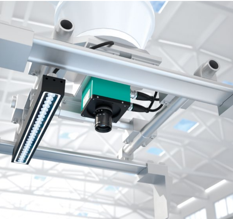
Identification of the battery cell via the Data Matrix code
