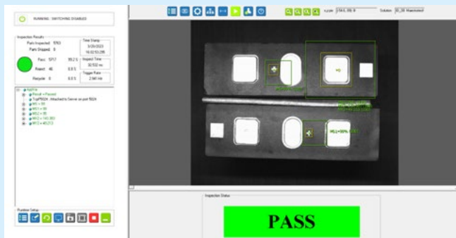
Battery cell alignment test
