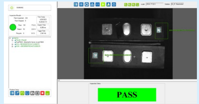
Identification of the battery cell via the Data Matrix code
