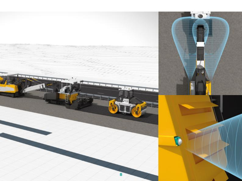
in road construction, have no influence on the measuring operation. Through vehicle-typical connectors such as AMP Superseal or DEUTSCH and the CANopen or J1939 interface, the sensors can be easily integrated into the on-board network.
