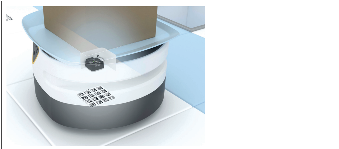
Figure 3.20 Application example: Exact AGTS alignment when picking up goods carriers (picking of loads).
