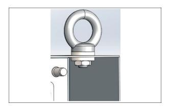
(5) The following total loads are allowed with a symmetrical load: F= 2000 N, Max 45°, see DIN EN 818-4.
