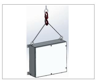
(6) The following maximum allowable load per eyebolt with a symmetrical load suspended vertically applies: F= 1400 N, total load: F= 2800 N.
