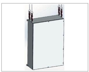
(9) Remove the eyebolts after mounting the enclosure.
