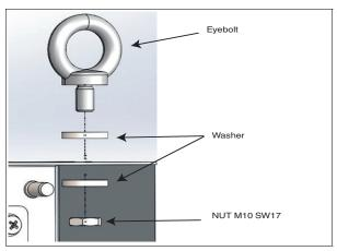
Tighten the locknuts to 20 Nm.
