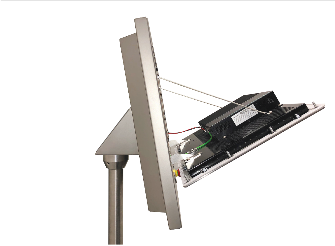
Figure 4.10 The safety lines hold the display when fully extended
