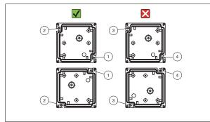
Use all existing screw holes for mounting the enclosure.
