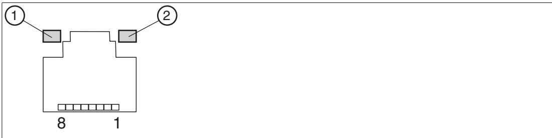
Figure 5.17 RJ45 pinout with LED display
