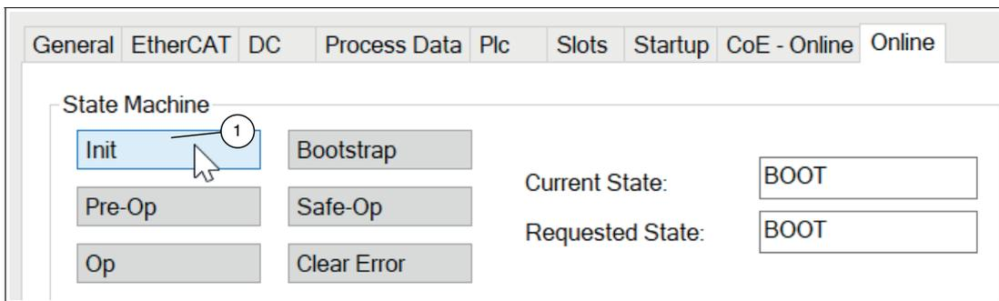
Figure 5.3 State Machine—Init
