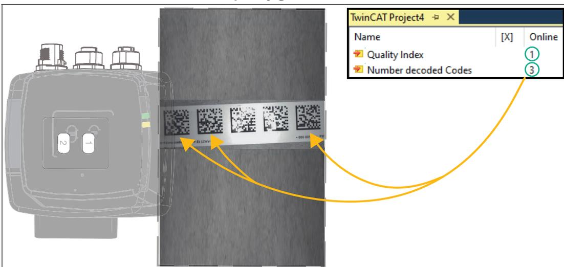
Figure 3.34 Code tape damaged by aggressive cleaning agent
