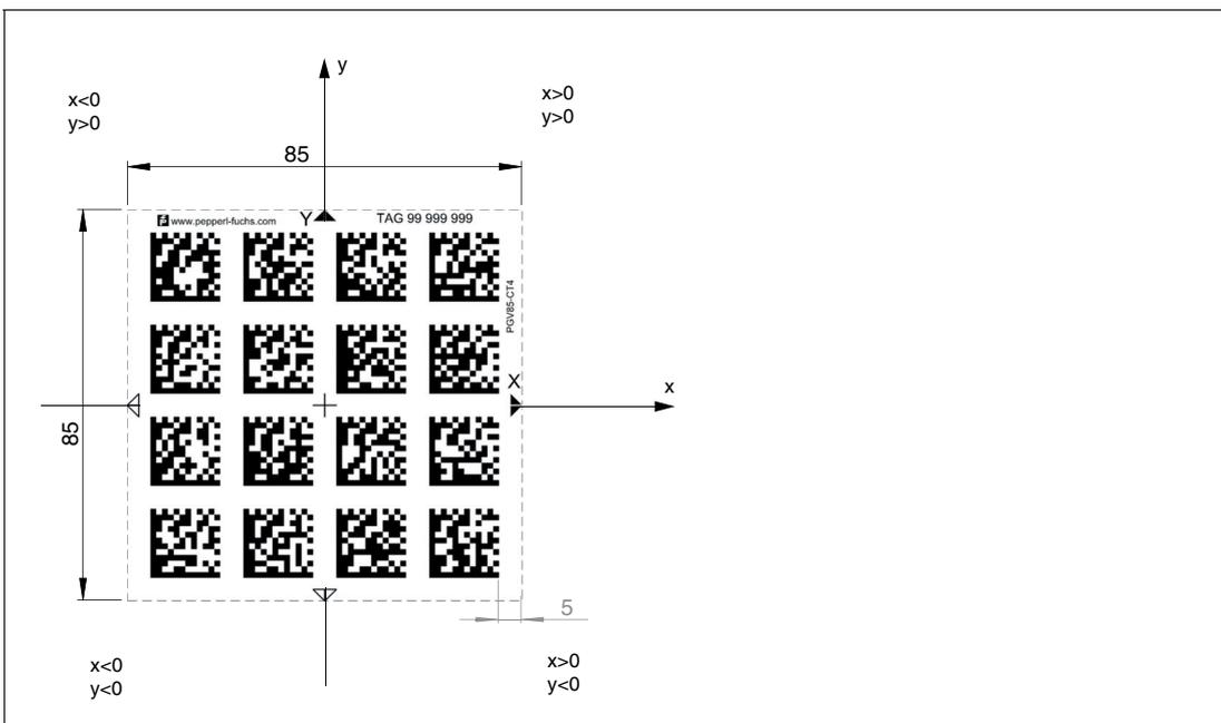
Figure 3.10 Data Matrix tag example with the number 99999999 and position information
