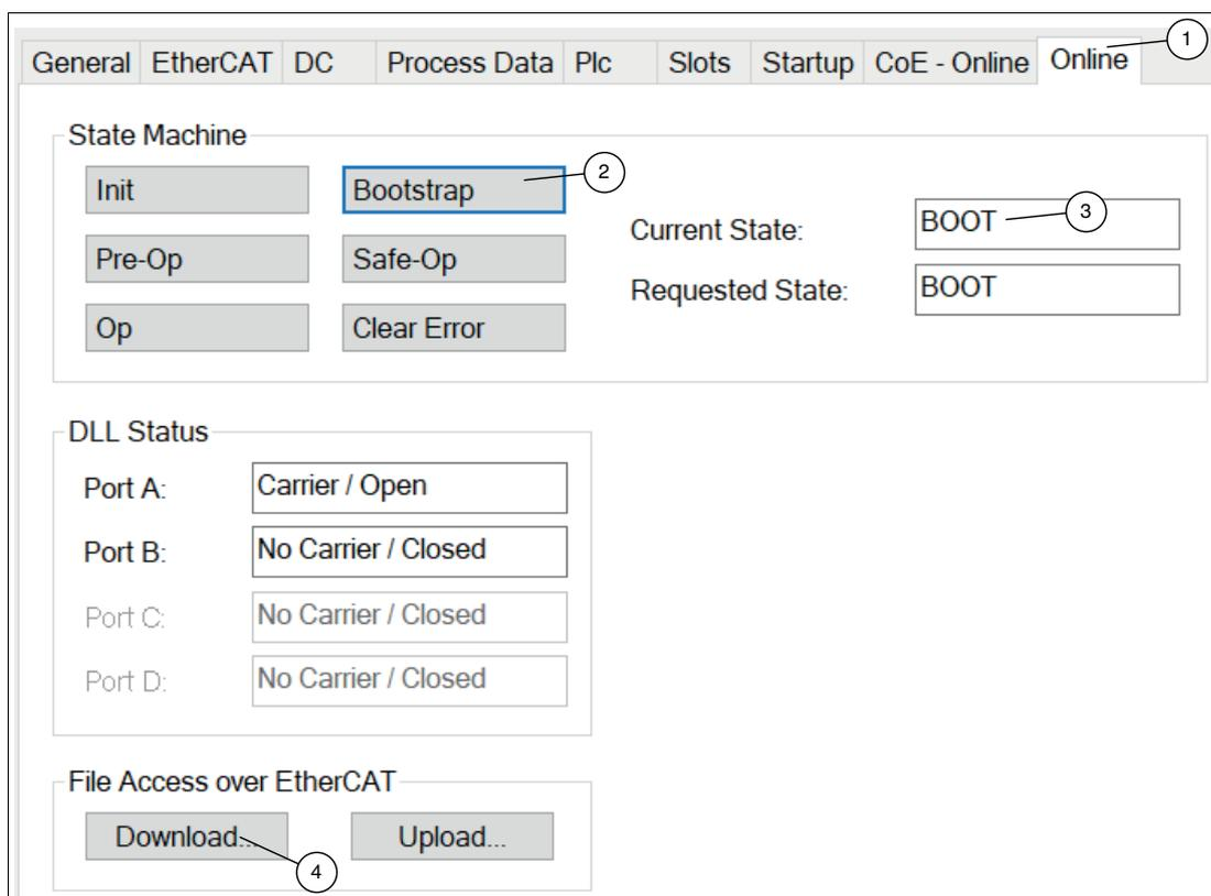
Figure 5.1 State Machine—Bootstrap
