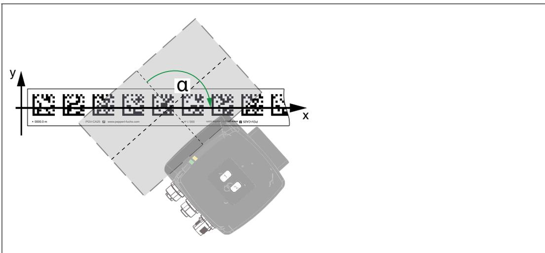
Figure 3.13 Absolute angle at  $130^\circ$
