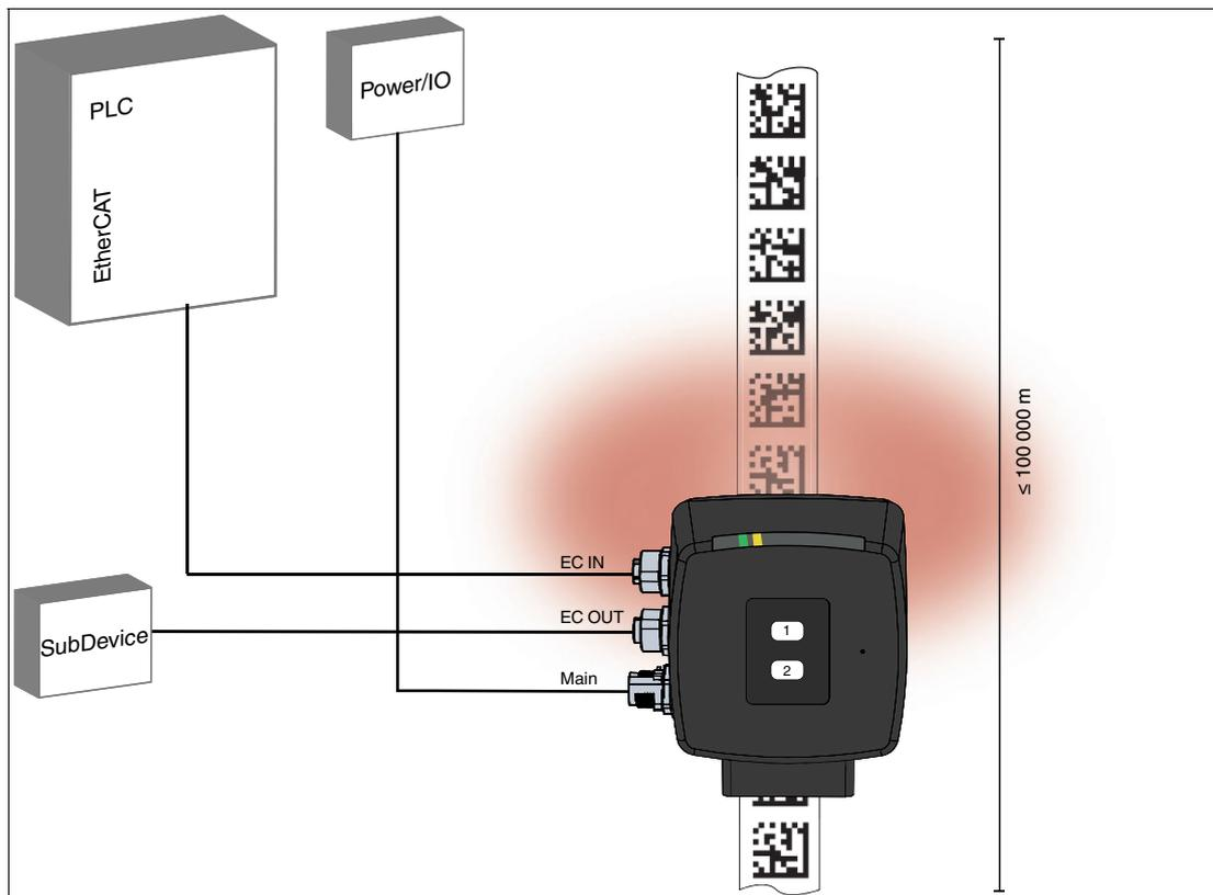
Figure 2.1 Schematic structure of the positioning system
