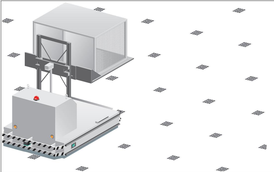
Figure 2.3 Auto-guided transport system with Data Matrix tags
