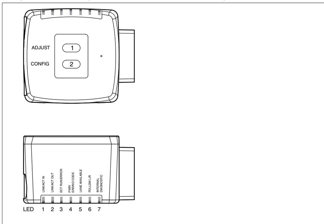
Figure 2.4 Overview of LED indicators and operating elements
