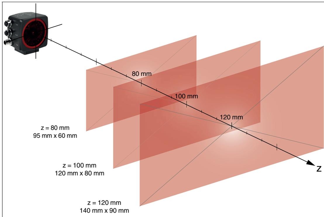
Figure 3.15 Size of the reading window of the read head in relation to the read distance z
