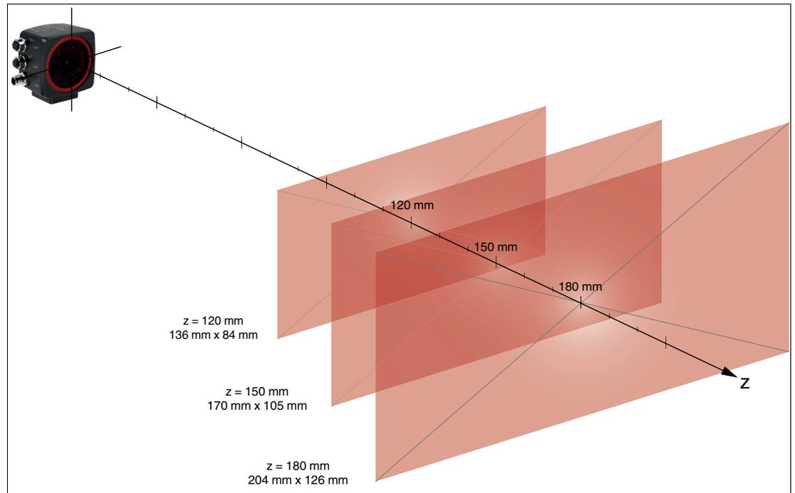
Figure 3.16 Size of the reading window of the read head in relation to the read distance z
