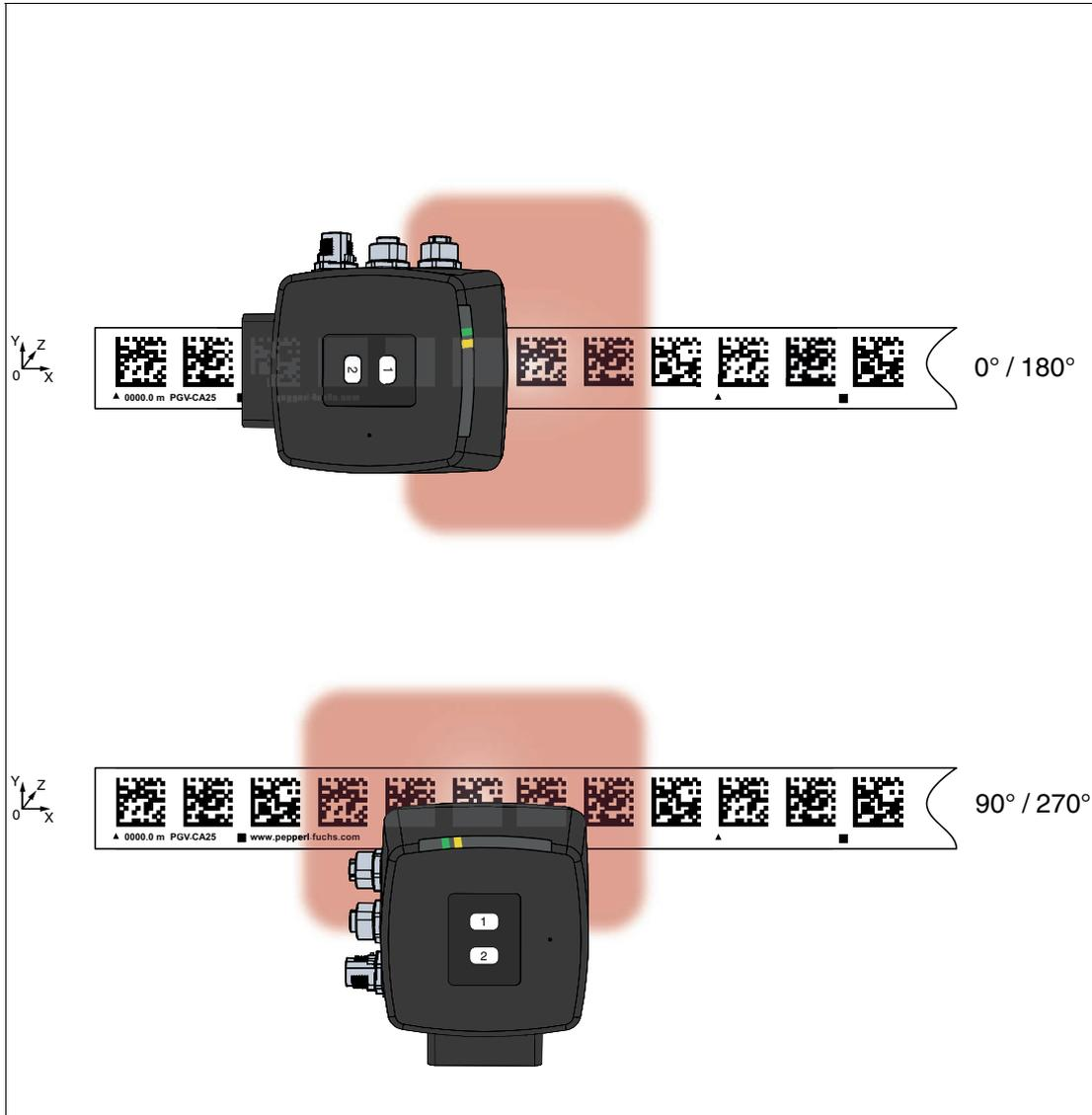
Figure 3.17 Read Head Orientation
