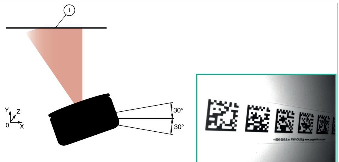
Figure 3.21 Horizontal orientation tolerance
