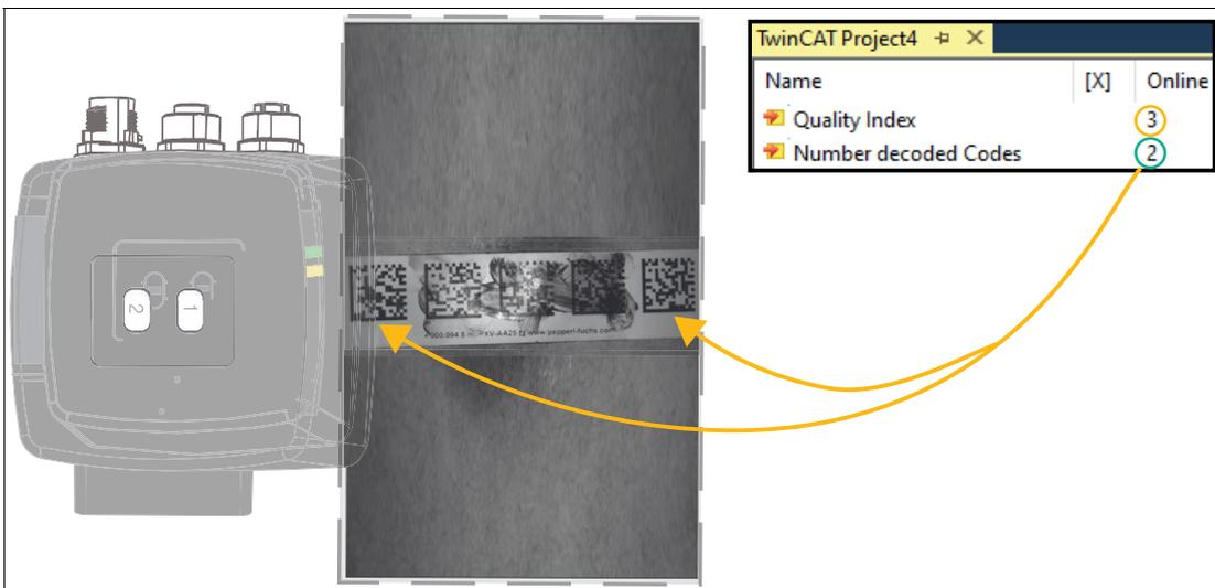
Figure 3.33 Code tape contaminated
