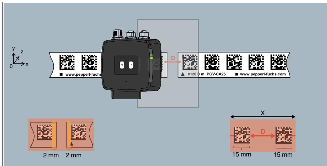
Figure 3.22 Expansion Joints / Gaps
