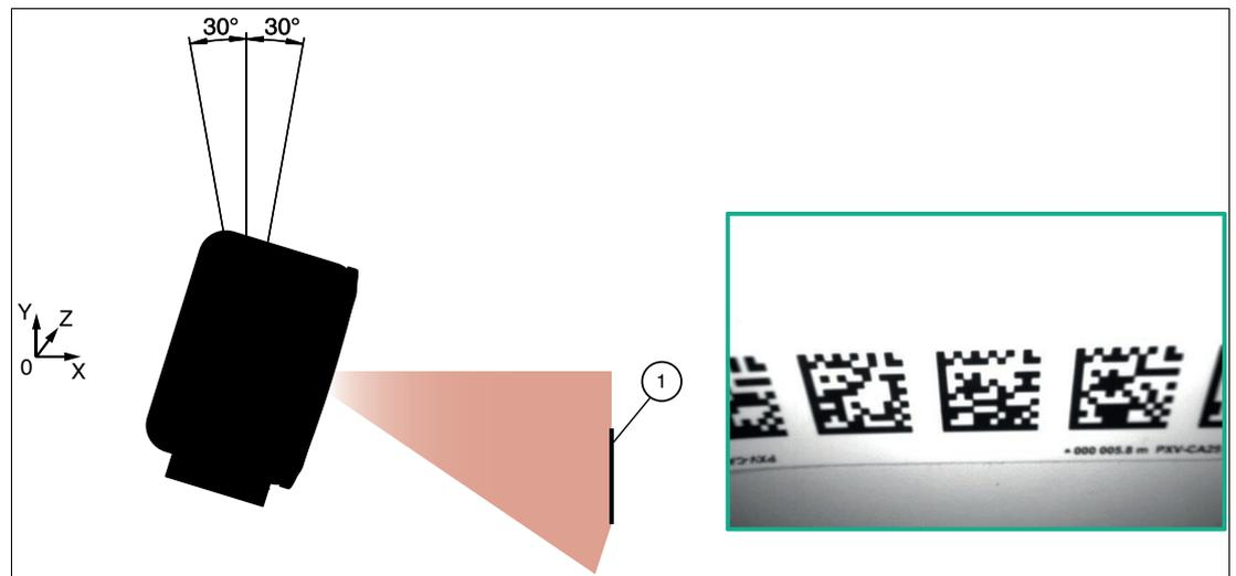
Figure 3.20 Vertical orientation tolerance
