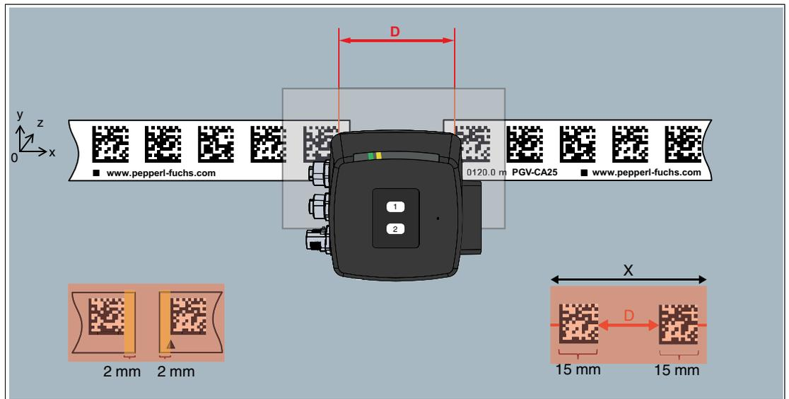
Figure 3.23 Expansion Joints / Gaps
