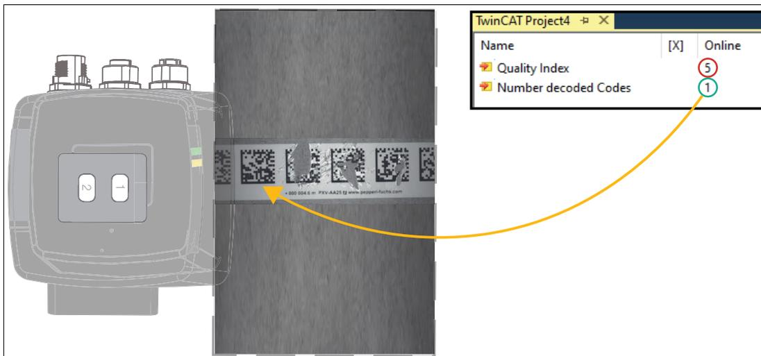
Figure 3.35 Code tape damaged
