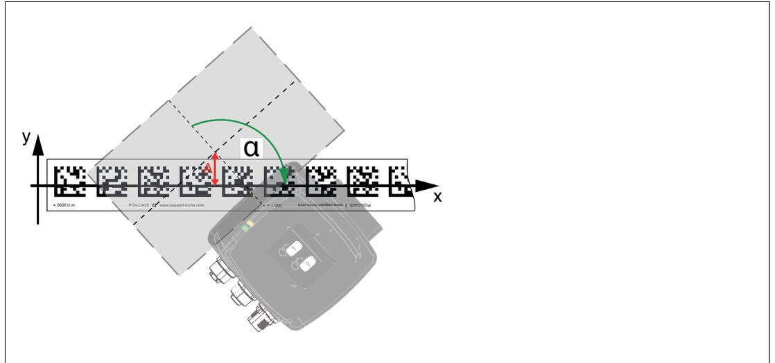
Figure 3.14 For example: Distance A = 20 mm and angle  $\alpha = 130^\circ$
