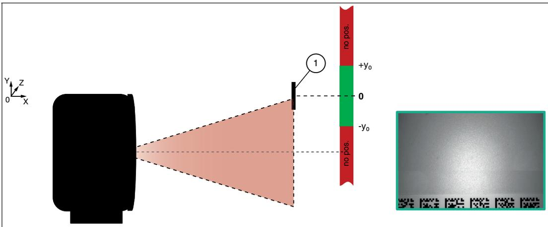
Figure 3.19 Red: Range in which a "No-position" message is set
