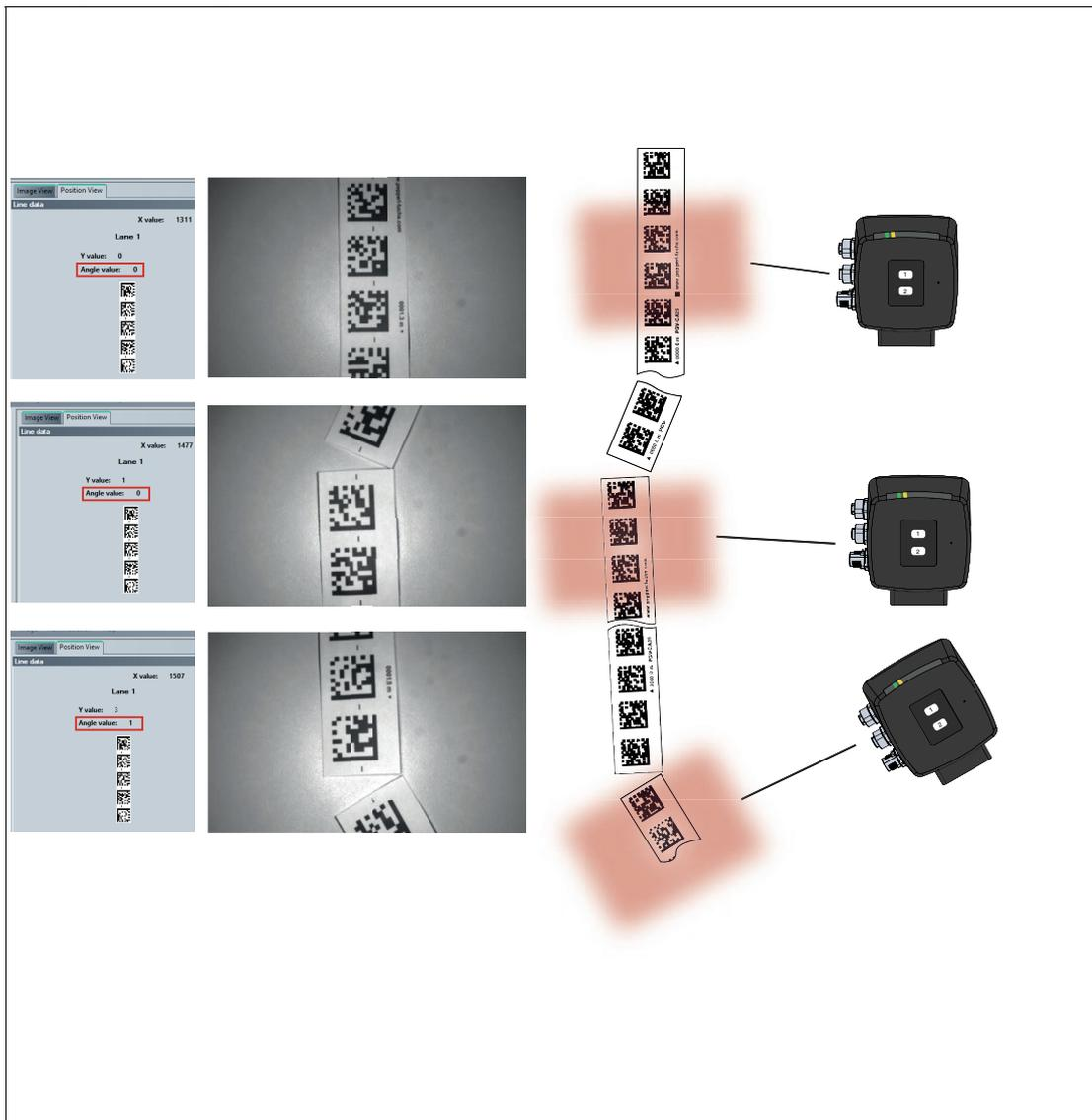
Figure 6.16 Example of an angle value
