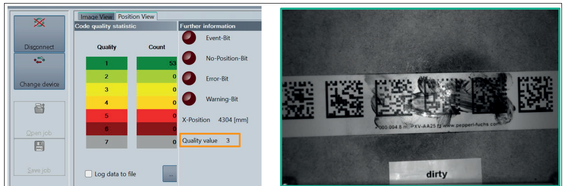
Figure 3.25 Code tape contaminated
