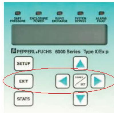
Using a keyboard sequence, simultaneously pressing: | EXIT | ◀ | START/STOP | ▶ | power will be interrupted to the EPCU and it will reset. All user-programmed functions will be saved, but the unit will reboot and then go through its procedure to energize the enclosure.
