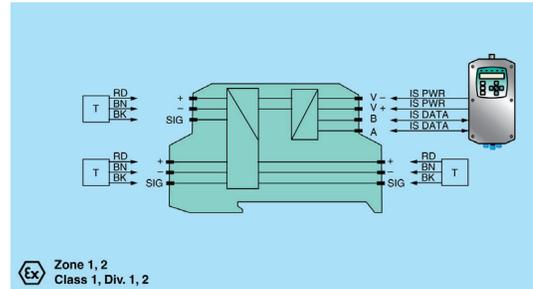
*Temperature hub and three sensors connected to the 6000 control unit*
