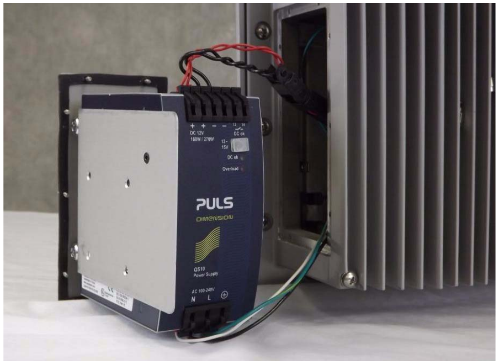
Figure 7.3 Power Supply Removed
