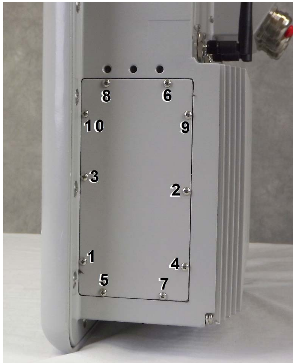
Figure 7.7 Power Supply Cover Plate Incremental Screw Tightening Order
