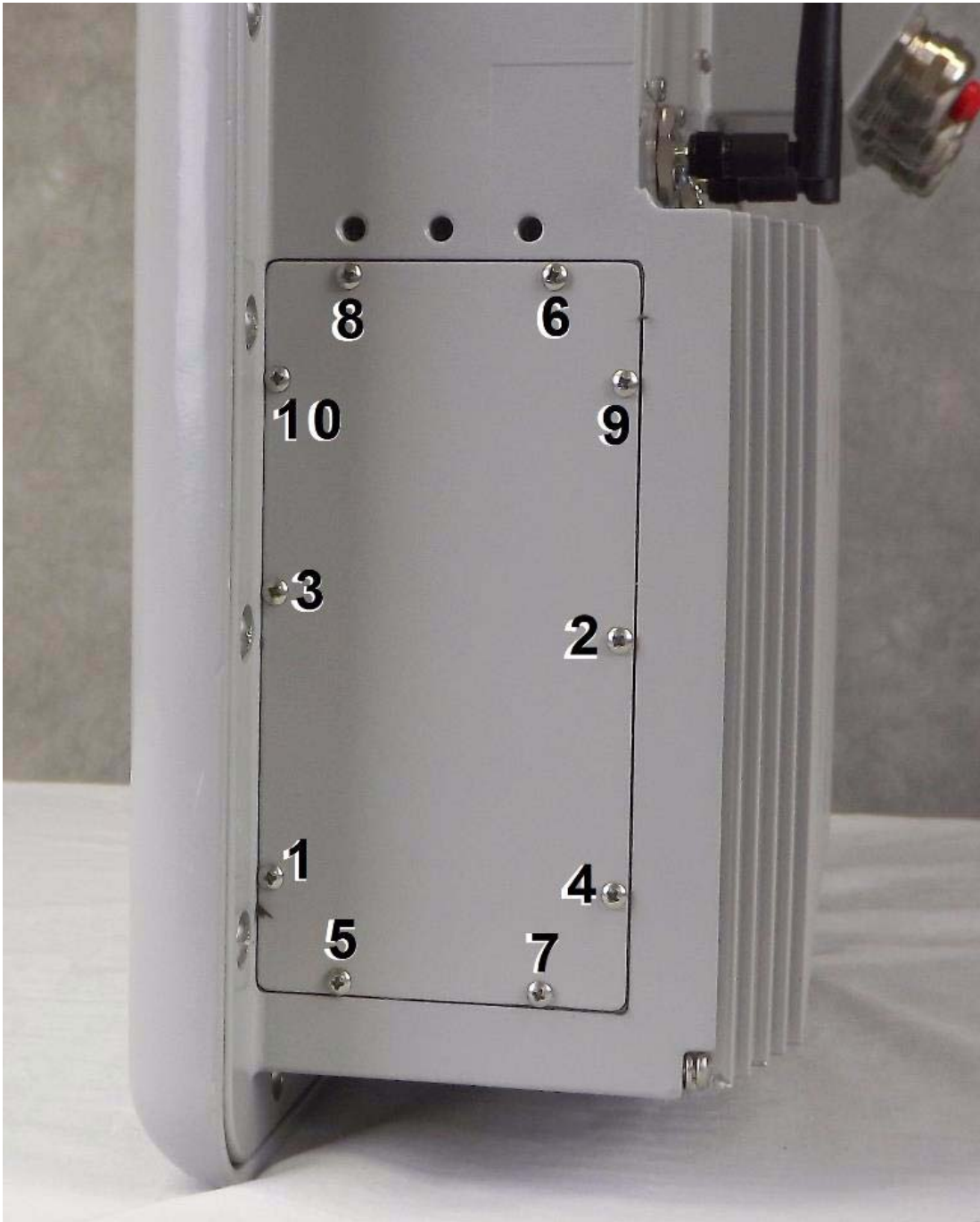
Figure 7.13 Correct inside-to-outside crisscross pattern
