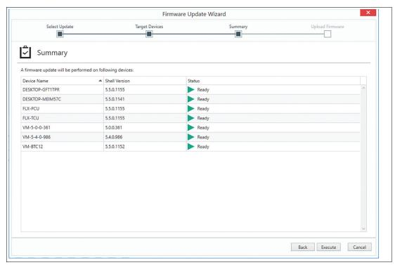
→ When every device Status is set to "Success", the performed action is completed and the wizard can be finished
