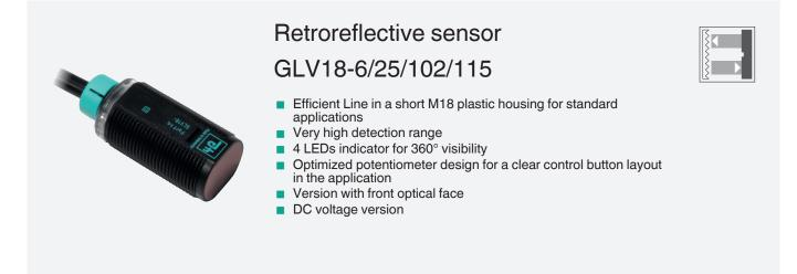
Retroreflective sensor, M18 threaded housing design, plastic housing, front optical face, 6.5 m detection range, red light, light on, DC version, NPN output, fixed cable
