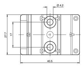
You may screw the device onto a level mounting surface using two M4 attachment screws. The attachement screws are not included.
