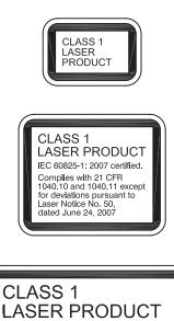
IEC 60825-1: 2007 certified. Complies with 21 CFR 1040.10 and 1040.11 except for deviations pursuant to Laser Notice No. 50, dated June 24, 2007 OBT300-R100-2EP-IO-V31-L
