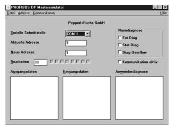
The PROFIBUS master simulator is a simple universal machine tool for data exchange with PROFIBUS slaves of almost all manufacturers via PROFIBUS DP. The PROFIBUS master simulator exchange data with many **PROFIBUS** slaves even without GSD file, type file and without PROFIBUS master. The PROFI-BUS slaves default I/O width can
