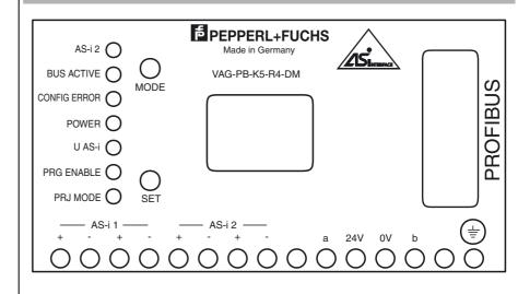
the master shall be supplied by AS-Interface-1 circuit (pos.1) or via an own power pade (PELV) (pos. 2).
