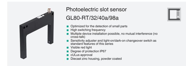
Photoelectric slot sensor, zinc pressure diecast housing, 80 mm slot width, red light, light/dark on, sensitivity adjuster, DC version, PNP output, 3 pin M8 plug
