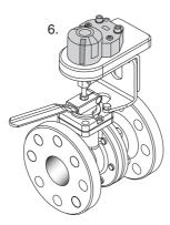
Finally perform a mechanical check of the assembly and a functional check of the position feedback.
