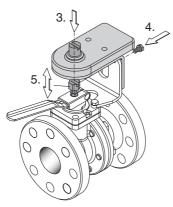
6. Install the actuator (puck) on top of the shaft and the valve sensor on the sensor plate.
