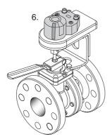
Finally perform a mechanical check of the assembly and a functional check of the position feedback.
