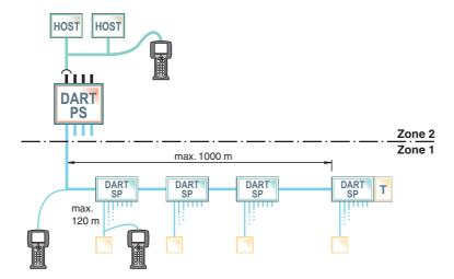
DART protects the fieldbus trunk. The DART power supply limits energy on the trunk to intrinsically safe levels Ex ib IIC.
