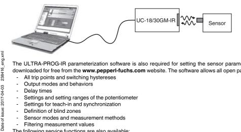
The ULTRA-PROG-IR parameterization software is also required for setting the sensor parameters. The ULTRA-PROG-IR software can be downloaded for free from the www.pepperl-fuchs.com website. The software allows all open parameters to be set, including:
