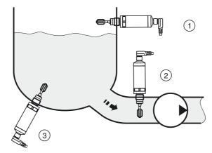
Example 1: overfill protection or top level detection Example 2: dry running protection for pump Example 3: lower level detection
