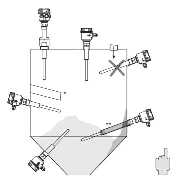
Horizontal installation/vertical installation
