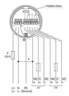
$U \approx 19 \ V \dots 253 \ V \ (AC) \qquad U = 19 \ V \dots 55 \ V \ (DC)$
