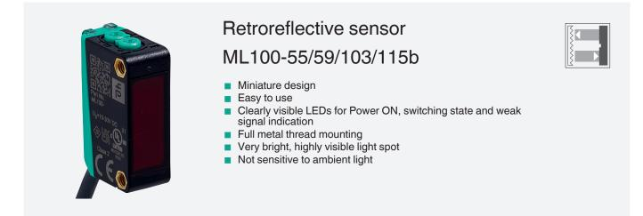
Retroreflective sensor with polarization filter, plastic housing, 5 m detection range, red light, sensitivity adjuster, light/dark on, DC version, PNP output, fixed cable with M12 plug
