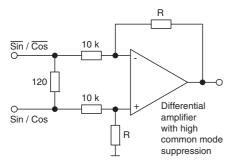
It is important to ensure that the load current does not exceed 10 mA at the output connection. The rotary encoder outputs are short-circuit proof.
