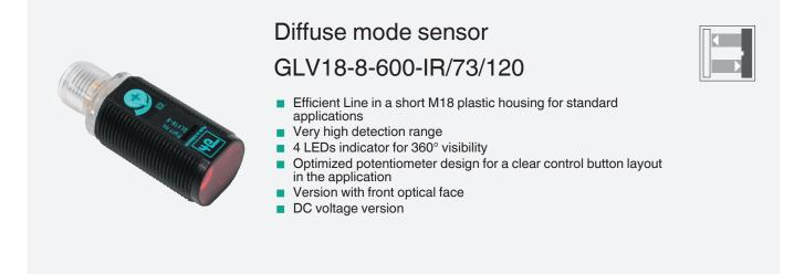
Diffuse mode sensor, M18 threaded housing design, plastic housing, front optical face, 600 mm sensing range, red light, light/dark on, DC version, 2 PNP outputs, M12 plug
