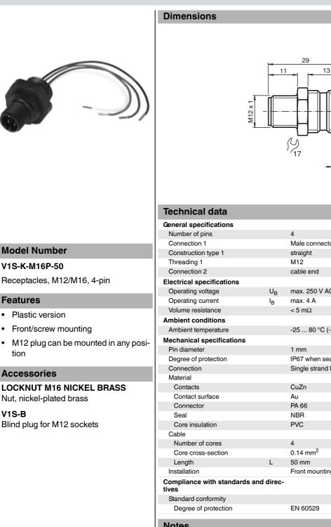
Male connector max. 250 V AC/DC -25 ... 80 °C (-13 ... 176 °F) IP67 when sealing with O-Ring Single strand leads with connector sleeves
