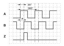
U cw - with view onto the shaft phase relationsships electrical \* 1 Measuring step is 90°
